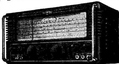
Four wavebands covering 32 mc/s to 480 Kc/s continuous except for a small gap around 1,600 Kc/s. Eleven valves. Separate oscillator, supplied with stabilized H.T. Independent R.F., I.F. and A.F. gain controls. Linear frequency scales, directly calibrated. Mechanical bandspread. With high reduction ratio geared tuning mechanism.
