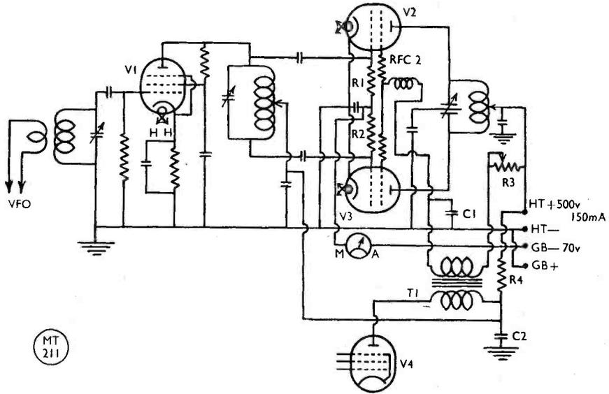
Fig. 1. The buffer-doubler PA circuit, showing connections for screen and control grid modulation of the push-pull 807's. The values given in the table are those directly affecting the operation of the system; otherwise, the circuit follows normal practice. (See also *Short Wave Magazine*, January and April, 1950.)
