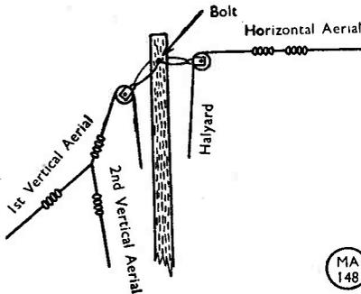
Fig. 2. General idea of the tie-up at the top of the mast, allowing independent lowering of the two sets of aerials.
