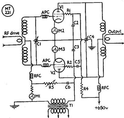
Fig. 3. The circuit as used by G6TA, derived from Fig. 2. All necessary values are given in the tables and results discussed in the text.
