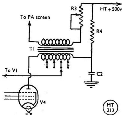
Fig. 2. The 6V6 modulator and modulation transformer as shown here illustrate the method of tapping the HT feed for V1 towards the anode of V4, thus providing a greater audio swing at the control grids of V2, V3.
