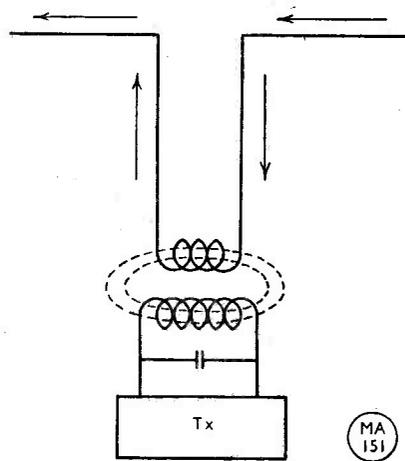
Fig. 1. Dipole and feeder system excited by inductive coupling. Instantaneous current distribution is as shown by the arrows. Note that equal and opposite currents appear in the feeder line.
