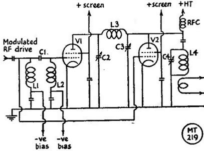
Fig. 1. If the effective load of L4, C4 with aerial connected is R1 ohms, then  $\omega L3 = 2R$ ;  $1/\omega C2 = 2R$ ; and  $1/\omega C3 = 2R$ . If the grid input resistance of V1 is Rg ohms, then  $\omega L1 = Rg$ ;  $\omega L2 = Rg$ ; and  $1/\omega C1 = Rg$ . There should be no mutual inductance between L1 and L2.
