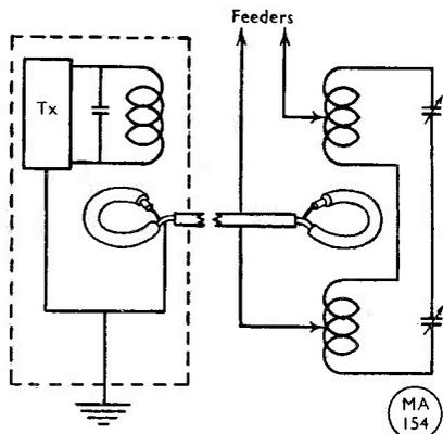
Fig. 4. Typical aerial tuning unit coupled to the transmitter using coax and two screened loops as Fig. 3.
