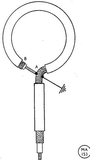
Fig. 3. Suitable screened coupling loop constructed from a length of coax, as described in the text.
