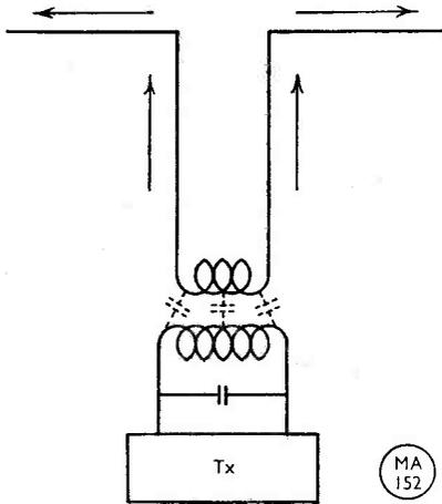
Fig. 2. The effect of stray capacity coupling from the transmitter; the dipole and its feeder are excited in a spurious mode, with in-phase currents appearing on the feeder line.
