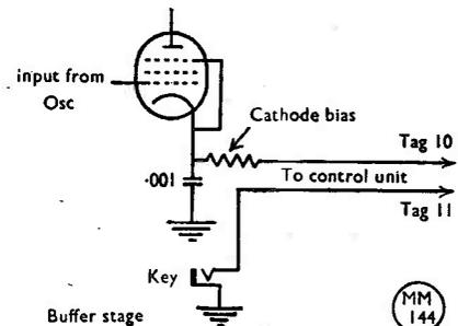
Fig. 2. The VFO connections in the control circuit.
