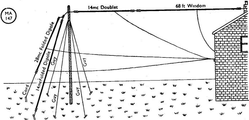
Fig. 1. Having noticed how coats can be hung round a hat-stand, G8UA decided to use his mast as a suspension for vertical aerials, somewhat in the manner shown in the sketch. His system consists actually of four separate aerials—two vertical, and two horizontal. Vertical or near-vertical aerials have the great advantage, on the HF bands, of almost omni-directional radiation.
