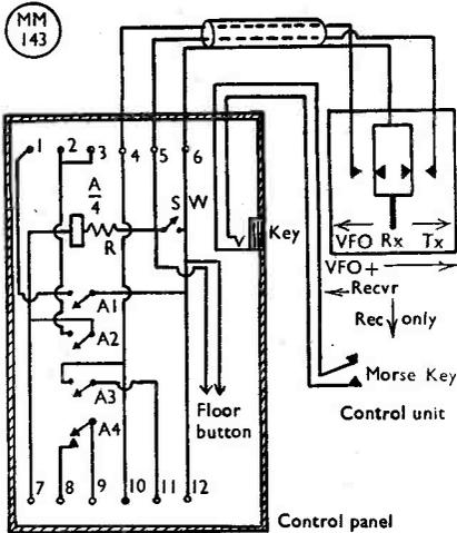
Fig. 1. General arrangement of the switching and control system devised by G2QY and discussed in the text. The key for the connections is given separately.
