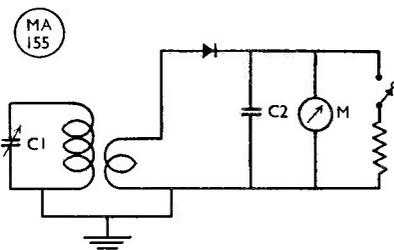
Fig. 5. A simple RF detector for investigation of current distribution along feeder and aerial systems, as discussed in the article. C1, C2 are .0001 μF and M is 0.1 mA
