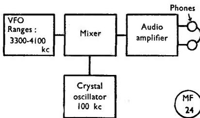
Fig. 1. Block schematic showing basic arrangement of the circuit.
