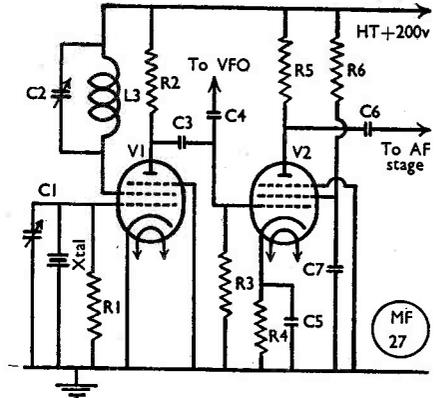
Fig. 4. Where it is desired to use two valves of the SP61 variety, as Pierce oscillator and separate mixer, the circuit can be modified as shown here; there is no particular virtue in having a combined oscillator-mixer.
