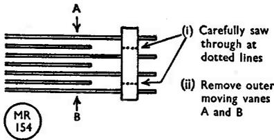
Fig. 2. The operation for improving bandspread on the S.640. The outer vanes of the bandspread condenser are removed (see text).
