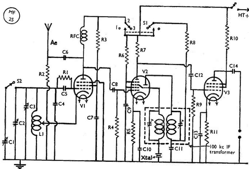
**Fig. 2. Circuit of the Heterodyne Frequency Meter complete, as described by G3CPR.**
