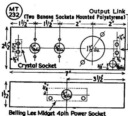
Fig. 2. Suitable chassis layout for the 145 mc Exciter.
