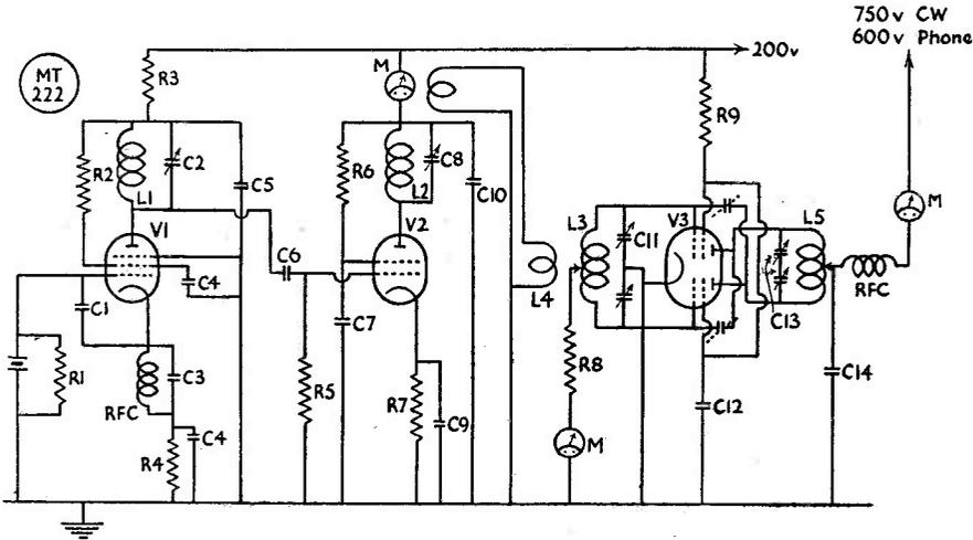
With a 7 mc crystal, it is possible to get full output on 28 mc using this circuit, as described in the text. The meters are for V2 plate (0-50 mA), V3 grid (0-25 mA), and V3 plate (0-250 mA).
