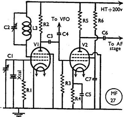
Fig. 4. Where it is desired to use two valves of the SP61 variety, as Pierce oscillator and separate mixer, the circuit can be modified as shown here; there is no particular virtue in having a combined oscillator-mixer.
