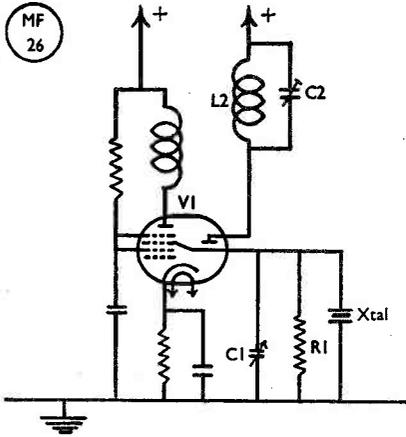
Fig. 3. G3CFR discusses the possibility of using crystals oscillating in the parallel mode; this is the circuit for it.
