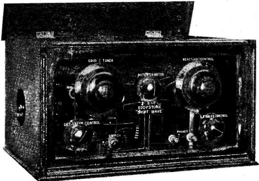
Many years ago, the firm of Stratton & Co. produced one of their first short wave receivers, made in the old factory in Bromsgrove Street, Birmingham. The model shown here was actually built in 1925, and is still in full working order. One of the features of this set, which was 0-V-1, was the glass panel—no doubt it was that which helped so much to get the tuning range down to 15 metres, considered an extraordinary low wavelength in 1925!
