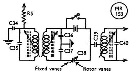
Fig. 1. The crystal phasing condenser C38 as originally connected in the receiver; by connecting C38 the other way round, the rotor vanes (and spindle) become earthy and direct pick-up at IF is minimised.
