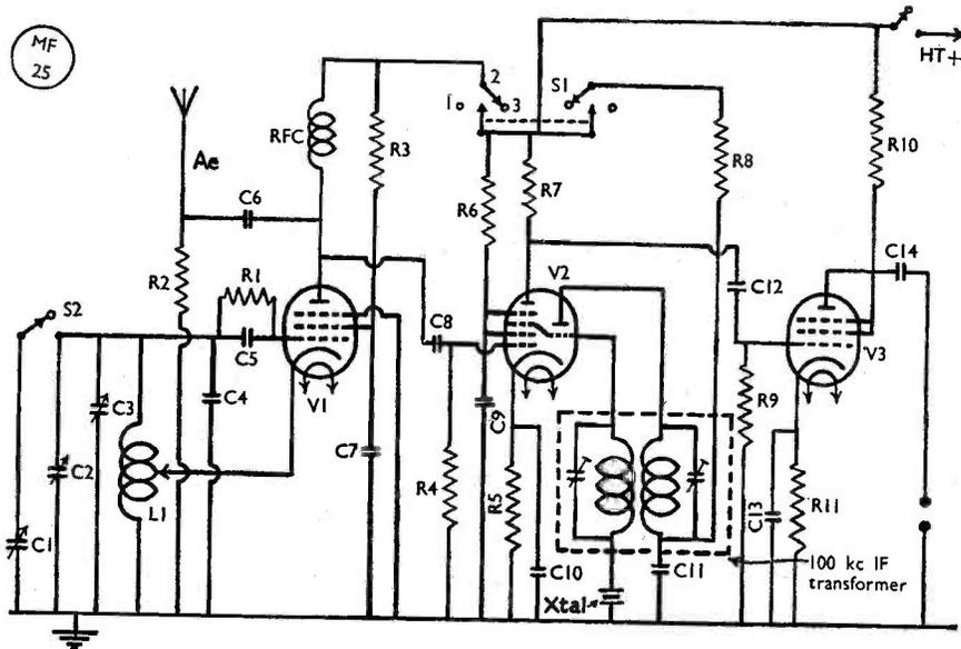
**Fig. 2. Circuit of the Heterodyne Frequency Meter complete, as described by G3CFR.**
