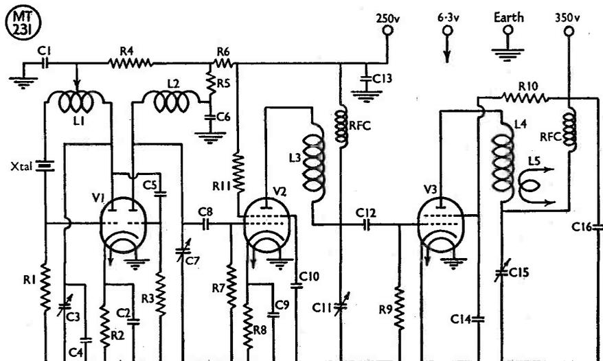
Fig. 1. Circuit complete of G2AJ's TVI-proof exciter-driver for the 145 mc band. It depends on correct choice of multiplier frequencies for the avoidance of TVI (see text).
