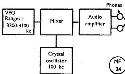
Fig. 1. Block schematic showing basic arrangement of the circuit.
