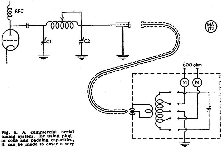
Fig. 5. A commercial aerial tuning system. By using plug-in coils and padding capacities, it can be made to cover a very wide frequency range.
