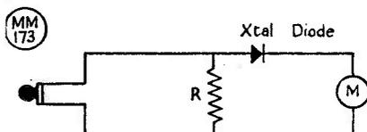
Fig. 2. The plug-in null indicator, discussed in the text. The crystal diode can be a 1N21 or 1N34, the meter 0-1 mA or 0-500  $\mu$ A, and the value of R is a matter of experiment, 8000 ohms being about right for an 0-1 mA meter.
