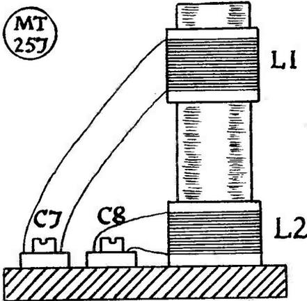
Fig. 4. Mechanical arrangement of the broad-band couplers described by G3ESV in his article. Compare this sketch with the photograph of a completed unit. It should be noted that with this form of construction the power must be kept low, otherwise the circulating current will be high and the units will tend to over-heat.
