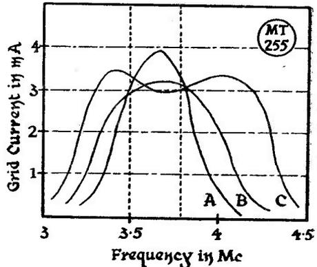
Fig. 2. These curves are of grid current against frequency in terms of band-width and show how changing the degree of coupling between L1, L2 in Fig. 1 affects the response. Taking 3.65 mc as the reference frequency, curve B indicates the correct degree of coupling for level drive conditions over the 80-metre band; in curve A the circuits are under-coupled (too "sharp") and in curve C they are too tightly coupled, giving the double-hump tuning effect.
