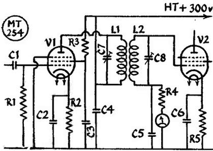
Fig. 1. Test circuit originally used by G3ESV for investigating broad band couplers in low power circuits. L1, L2 are the coupler windings, fixed-tuned by C7, C8 and the optimum degree of coupling between L1, L2 was determined by the reading obtained on the meter in the grid of V2 for a given input at the grid of V1.
