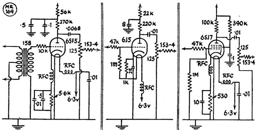
Fig. 2. Three possible methods of wiring in the additional speech amplifier, depending upon what type of microphone and 1st audio stage valve are to be used. In each case, RFC is 20 turns of No. 28 SWG enamelled wire on a 1-watt resistor as former.
