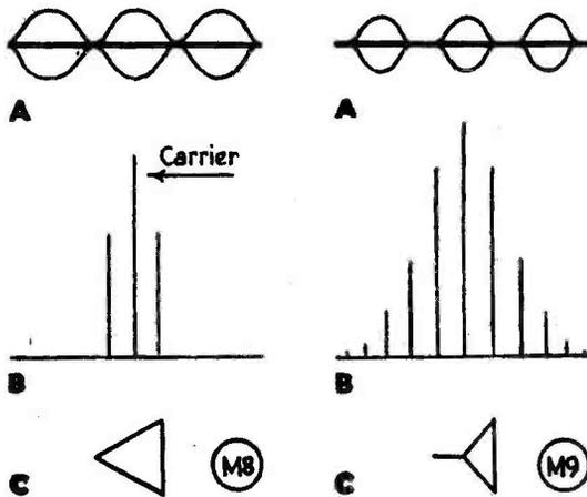
Fig. 1. Sine-wave modulation, 100%. (A) Modulation envelope; (B) Carrier and two sidebands; (C) Modulation pattern as seen on CRT. Ideally, with pure-tone modulation only two sidebands of half carrier peak amplitude are produced.
