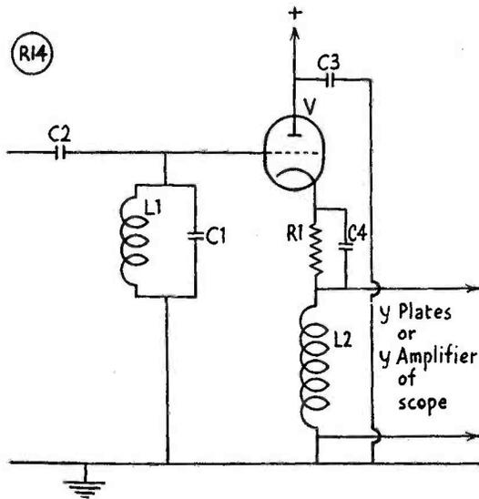
Fig. 1. Cathode follower connection for the 'scope. C2, 20 $\mu$ F, silver mica; C3, C4 .005  $\mu$ F; R1, as required; L1/C1, to resonate at IF, or replaceable by 100,000 ohm resistor; L2, RF choke; V, 6J5 or similar.
