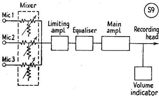
Block diagram of a typical recording system.
