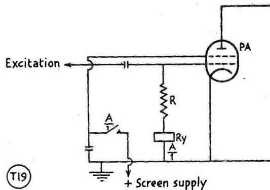
The circuit used by G5WB. The relay Ry cannot operate until drive is applied; it then switches HT to the screen of the valve. If drive falls or the grid resistor breaks down, screen HT is removed. The resistor R, with the relay resistance itself, should equal the total resistance required to give the necessary bias.
