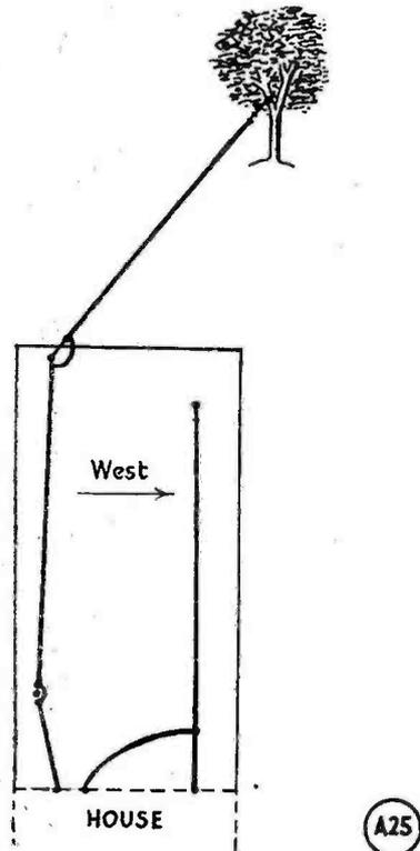
Fig. 3. A modification of the system as used during the 1951/52 Top Band DX Tests.
