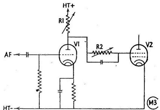
Fig. 1. Heising Constant Current Modulation on the screen-grid of a PA stage.
