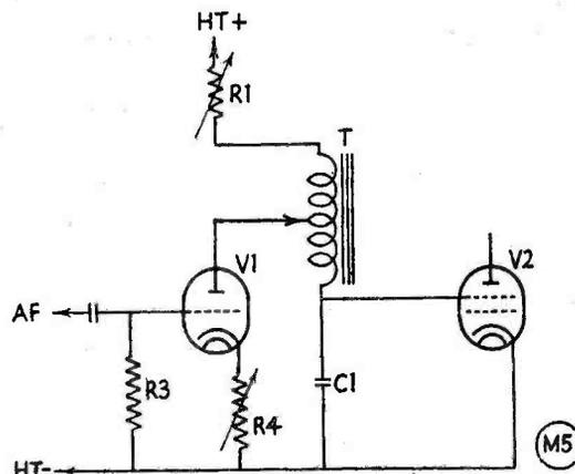
Fig. 3. An Improved Clamp Tube Modulator circuit, discussed by G3ENI.
