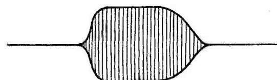
Fig. 11. Key filter overdone. Signal will sound woolly. No clicks. Primary keying with power pack filter too large gives same effect.
