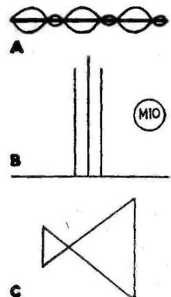
Fig. 3. Negative carrier insertion. (A) Modulation envelope accommodating "negative" modulation peaks; (B) Carrier and sidebands. While sidebands are much stronger than with 100% modulation, no spurious sidebands are introduced; (C) The characteristic double-triangle modulation pattern produced on the CRT.
