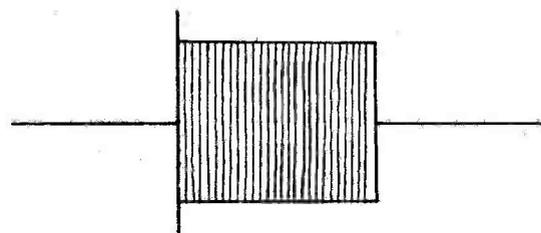
Fig. 9. Incorrect or no key filter. Signal fairly clean to read but bad click on make. Click persisting off resonance.
