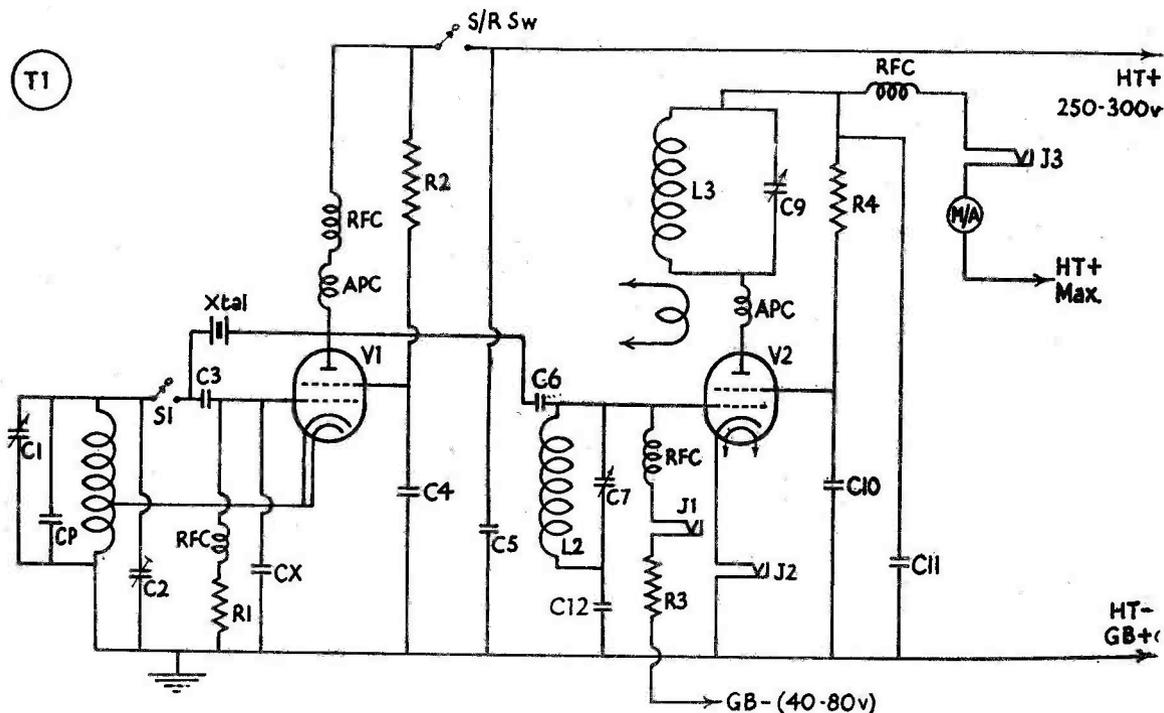
Fig. 1. Circuit of the 807 two-stage four-band transmitter suggested by G4AY. APC are aperiodic RF chokes, and the condenser from the bottom of L2 to the base line is C12, of .001  $\mu$ F.
