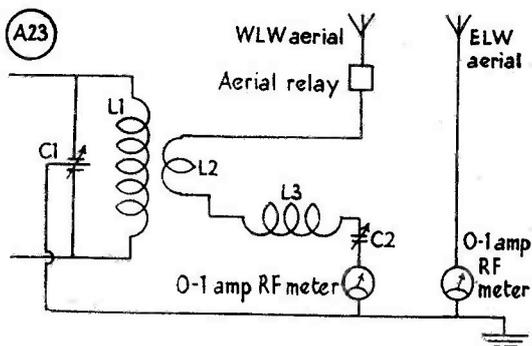
Fig. 1. Current-feed system used with 135ft. end-on wire operated as a Marconi aerial on 160 metres. C1/L1, balanced tank circuit; L2, coupling link; L3, loading coil, 24t. of 18g. enam. on 2 in. former; C2, .0005  $\mu$ F receiving type condenser.
