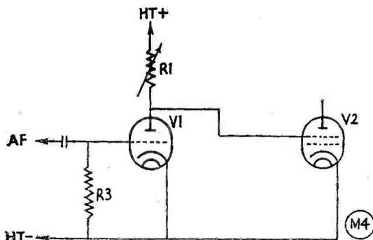
Fig. 2. Clamp Tube Modulation—which has been discussed in recent articles.
