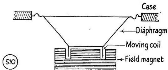
Outline sketch showing arrangement of a typical moving-coil microphone.
