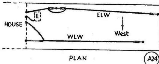
Fig. 2. General arrangement of the two 135ft. aerials at G5JU (roughly to scale). Point E indicates the position of the buried earth mentioned in the text.
