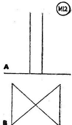
Fig. 5. Double Sideband Suppressed Carrier. (A) Two sidebands with no carrier; (B) The double-triangle pattern as seen on the CRT. This condition corresponds to a modulation index (and modulation percentage) of infinity. Such a signal is easy to produce but is impracticable for communication purposes owing to difficulties at the receiver.
