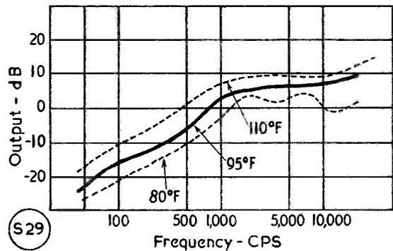
Fig. 2. Change in frequency response with temperature.
