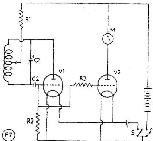
Fig. 1. Circuit of the GDO as constructed by G6FW. It is based on the original G5JU design, but is made self-contained and therefore fully portable by the use of miniature valves and battery power.
