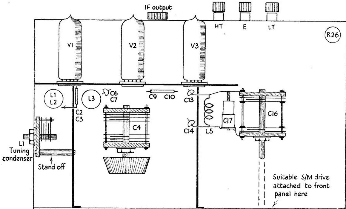
Fig. 4. Disposition of parts in G5RZ's version of the G2IQ 144 mc converter. References are to circuit elements as given in the original article—see August, 1949, issue.
