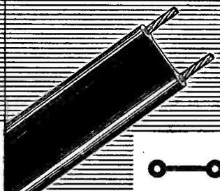
**K.25.B** 300-ohms nominal impedance, flat ribbon-type twin; capacitance 4.6 mmf/ft; attenuation at 50 Mc/s, 1.0 db/100ft; power rating at 100 Mc/s 500 watts.
