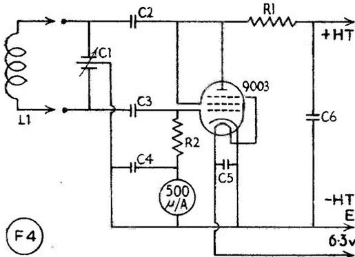
Fig. 1. Circuit of the two-metre GDO used by G5RZ. It was found to be absolutely essential for all tests and exploratory work on the 144 mc converter.
