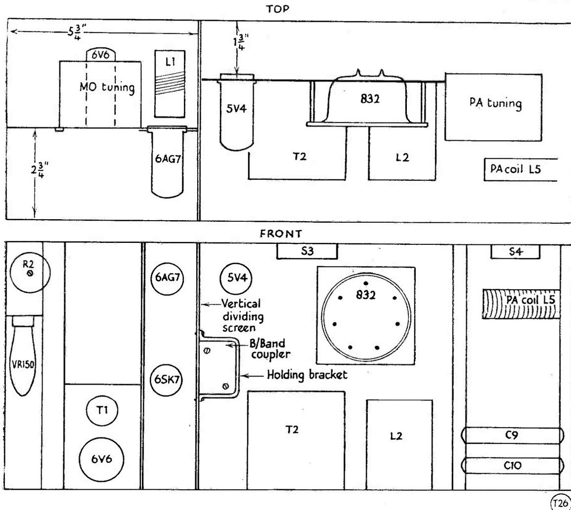
Fig. 2. Sketches showing levels of screens and general layout of the main components on the TU6 chassis; as indicated here, all the space is carefully used.
