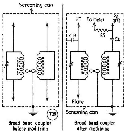
Fig. 4. Modification to the commercial broad band coupler, as mentioned in the article by VQZAH. C6 is 100  $\mu\text{F}$ ; C13, .005  $\mu\text{F}$ ; and R5 20,000 ohms.
