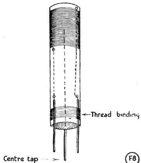
Fig. 2. Showing the construction of the coils for the LF ranges—see text for explanations.
