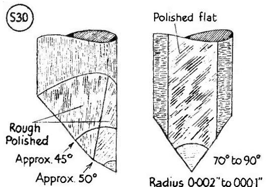
Fig. 3. The shape of a recording stylus (greatly enlarged), as explained and discussed in the text.
