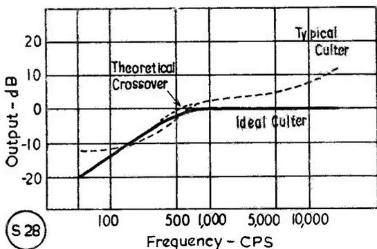
Fig. 1. The recording characteristic.
