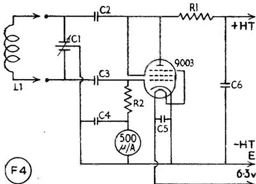
Fig. 1. Circuit of the two-metre GDO used by G5RZ. It was found to be absolutely essential for all tests and exploratory work on the 144 mc converter.
