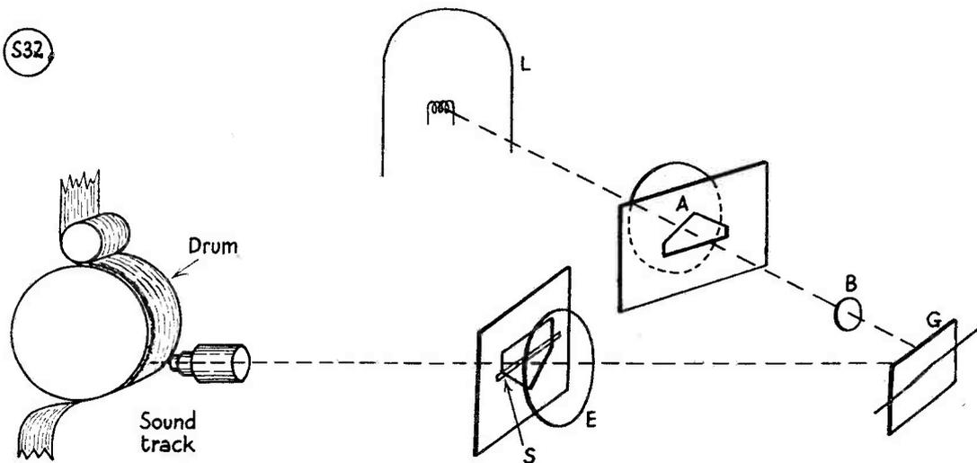
Fig. 5. Diagrammatic representation of the optical system involved in photographic sound recording. This is as for the sound-on-film technique now generally used in recording for the cinema.
