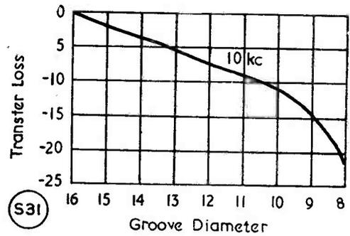
Fig. 4. Representation of losses due to what is known as Tracing Distortion, an important factor in high quality work.
