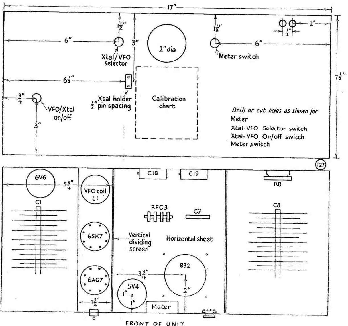
Fig. 3. Further constructional details and placing of components. This is a front-panel and top-chassis view and is not to scale.
