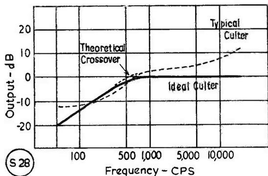
Fig. 1. The recording characteristic.
