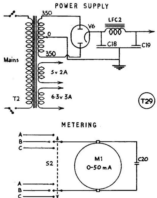
Fig. 5. Power supply unit and meter connection for the QRP 20/40 Transmitter. C20 is .002  $\mu$ F; S2 is a Yaxley switch; M1 an 0-50 mA meter; T2 the mains transformer; LFC2 a suitable smoothing choke; C18, 8  $\mu$ F 500v. DC electrolytic; C19, 16  $\mu$ F rated as C18; V6, suitable rectifier.
