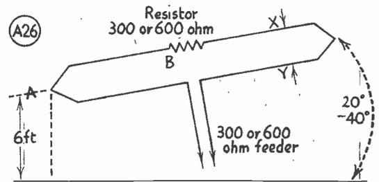
See table 1 for length of leg AB and spacing XY
