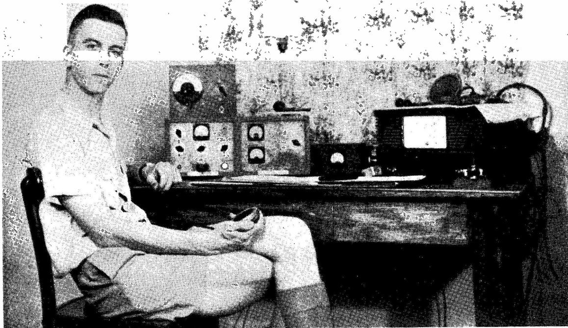
Station of ZE3JJ, Salisbury, Southern Rhodesia, who has been on the air since early 1950. The Tx is 6V6-807-807 running 60 watts, with optional CC or VFO control using a TT11 in an ECO circuit. Modulation is by a pair of 6L6's, and the aerial for Ten a 2-element rotary beam ; on the 21 mc band, ZE3JJ gained the world's first WAC, using a vertical Zepp. The Rx is an Eddystone S.640.
