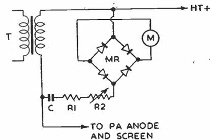
Circuit of the modulation indicator described by G3FYY in the accompanying article. Values are for 25-watt operation—see Table.
