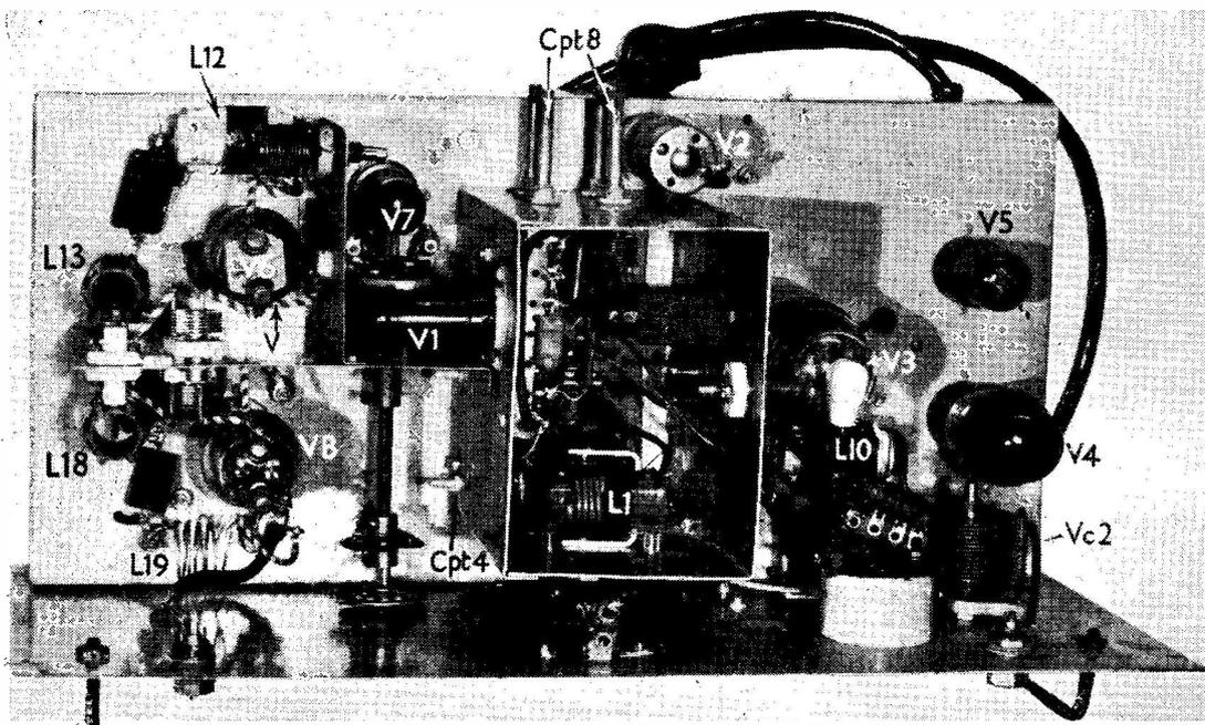
Behind-panel construction of the Exciter, showing main parts. In this view, "Cpt8" refers to padder condensers Cp5-8 (see text) and "VB" is V8 in the circuit of Fig. 4.
