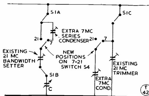
Fig. 3. Method of accommodating different bandwidths in the VFO tuner to cover the 7 and 21 mc bands.
