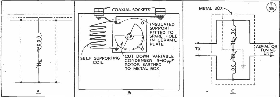
Fig. 4. Theoretical circuit (A), and practical construction (B), of a TVI filter designed to attenuate one particular harmonic with negligible effect on the fundamental output. The unit is contained in a fully-screened diecast box and the condenser is a cut-down miniature variable. A second tuned circuit (C) has to be added if the output line is of the balanced type.
