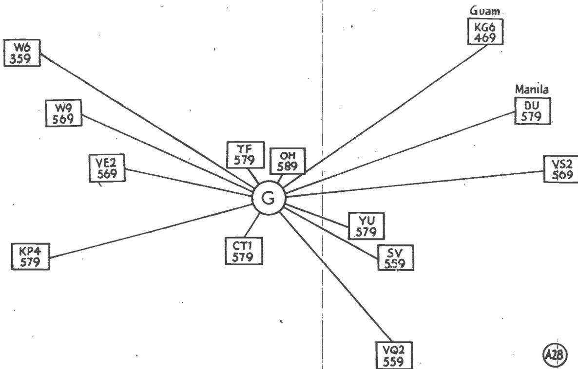
Fig. 3. Results obtained by G2NS under actual test conditions using the "T2FD" aerial described in this article. Transmission was on the 20-metre band for ten operating sessions and the directions shown here are roughly great circle paths in each case.
