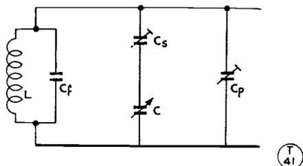
Fig. 2. Basic circuit of the VFO tuning system in the Exciter unit described in the article.
