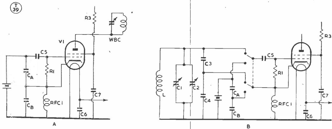
Fig. 5. The transmitter can easily be converted to crystal by changing the "front end" to correspond to (A) above.  $C_a$  is  $20 \mu\mu F$  &  $C_b$   $40 \mu\mu F$ , other values being as in Fig. 1. Crystal or VFO control is possible by the throw of a switch if the circuit at (B) is adopted.
