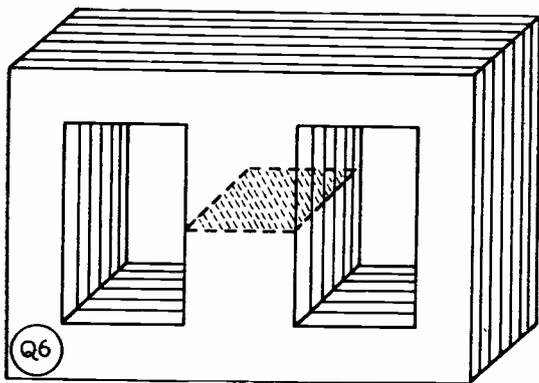
Fig. 1. Shaded portion shows cross-sectional area referred to in text. The width of the centre arm is exactly double the width of the sides, and there is no air gap.
