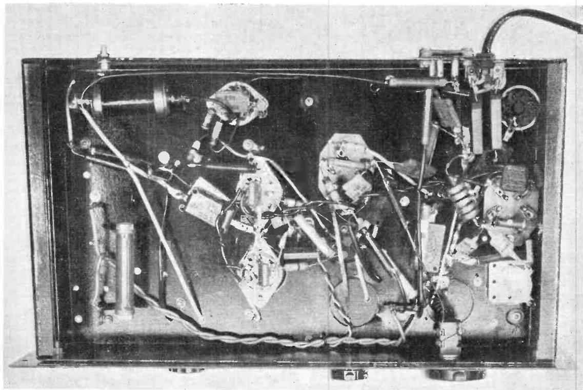
Underneath the chassis of the All-807 HF transmitter. Resistors R4 and R16, which develop some heat, are mounted well away from the oscillator stage.
