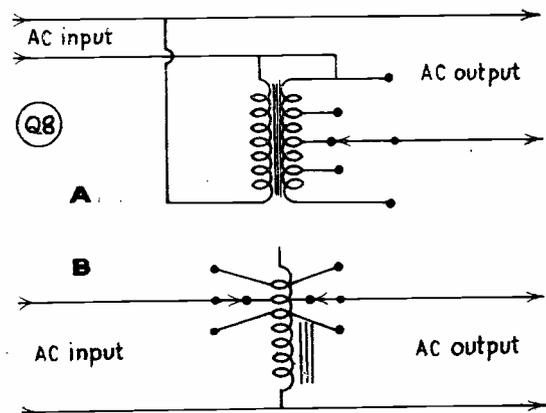
Fig. 5. Two methods of adjusting supply voltage; in (A) a small transformer would be quite adequate.
