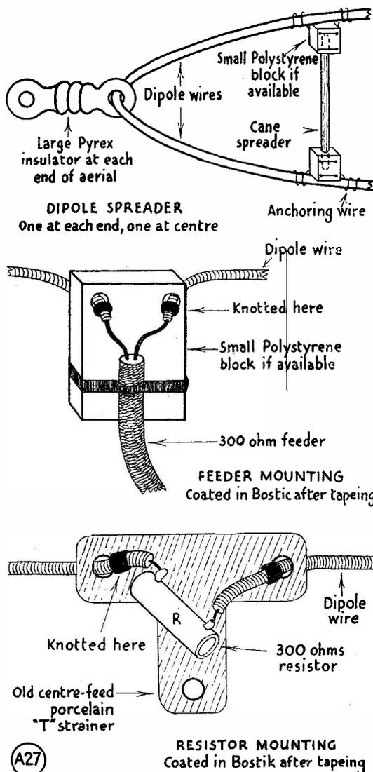
Fig. 2. Necessary constructional details for the Terminated Tilted Folded Dipole system described by G2NS.
