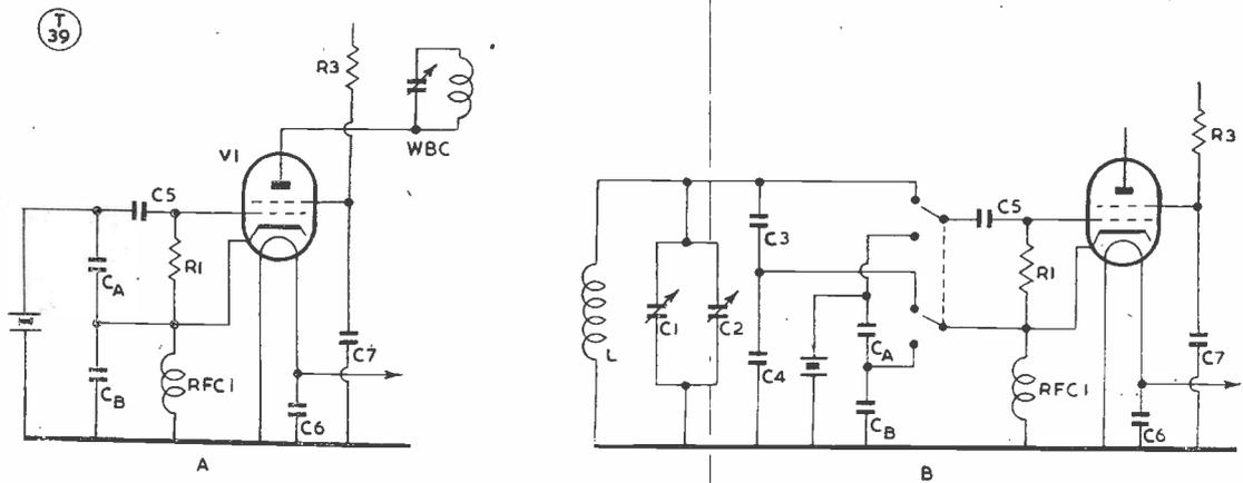
Fig. 5. The transmitter can easily be converted to crystal by changing the " front end " to correspond to (A) above. Ca is 20µµF & Cb 40µµF, other values being as in Fig. 1. Crystal or VFO control is possible by the throw of a switch if the circuit at (B) is adopted.
