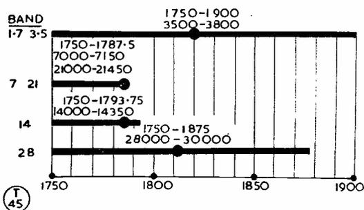
Fig. 6. This diagram shows the six bands covered by the Exciter, giving the frequency relationship, band-to-band, based on the fundamental tuning range.
