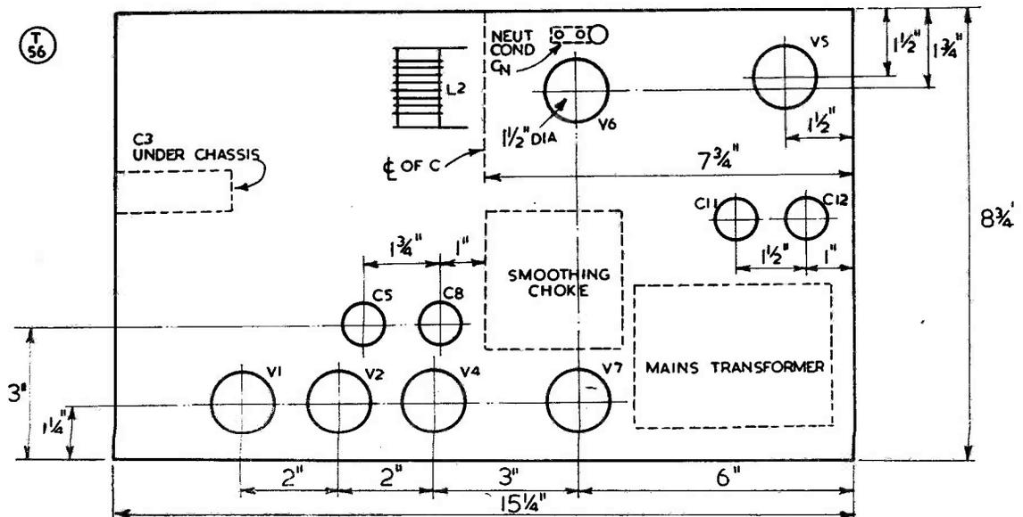
Fig. 3. Layout of the Transmitter chassis. This can be varied to suit individual requirements, but must be closely followed if construction is to be as specified.
