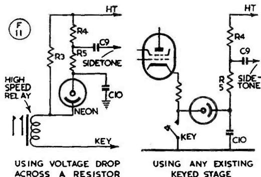
Fig. 5. An ingenious application of the neon to get sidetone on CW. Two possible arrangements are shown, and are covered in the text. Values of C9, C10 can be found by experiment.
