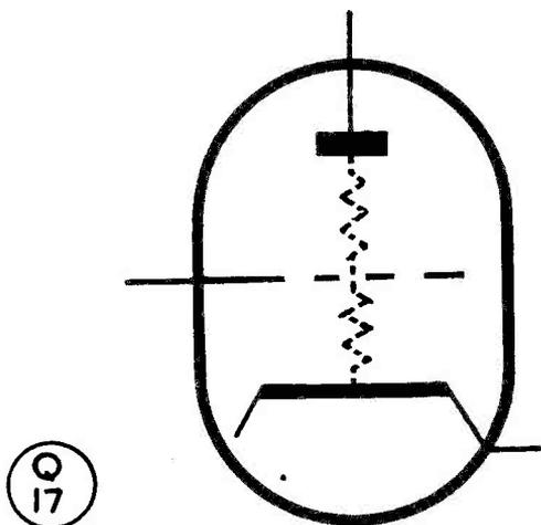
Fig. 1. The dotted resistors represent leakage paths between anode-grid and grid-cathode in a triode valve.
