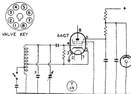
Fig. 2. The arrangement of Fig. 1 applied to another type of VFO. The basis of the idea is to be able to keep HT on the VFO, with the valve oscillating normally, but to prevent beating in the receiver on the operating channel. The effect is a high degree of VFO stability, as there is no HT switching, and therefore no change in valve temperatures and no variation in HT loading.
