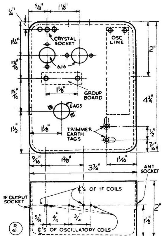
Fig. 2. Drilling detail and dimensions for mounting box for the G2DD Converter. It can be one of the standard Eddystone shapes.
