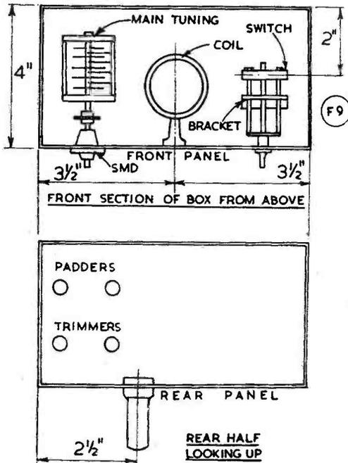
Fig. 3. Sketch showing general arrangement and layout of main components.
