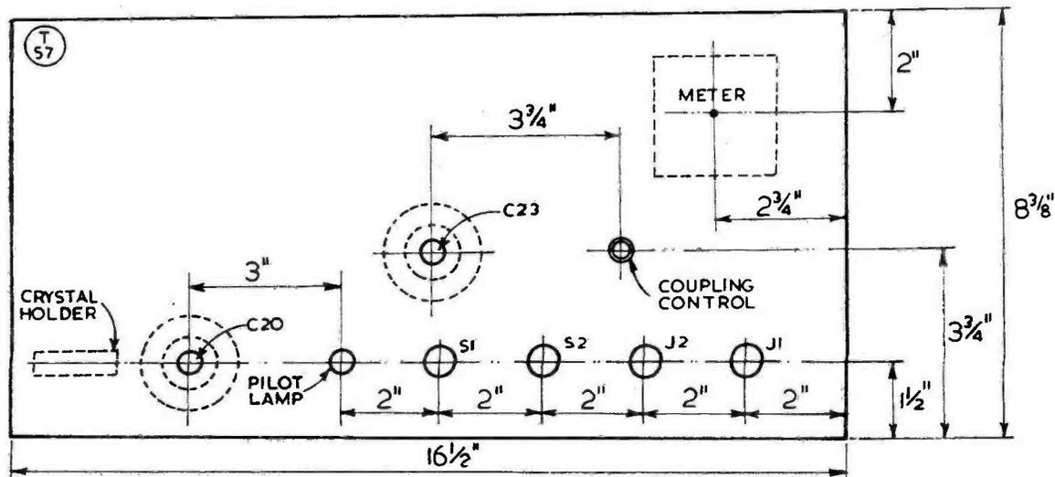
Fig. 4. Panel layout for the 10-metre Transmitter.
