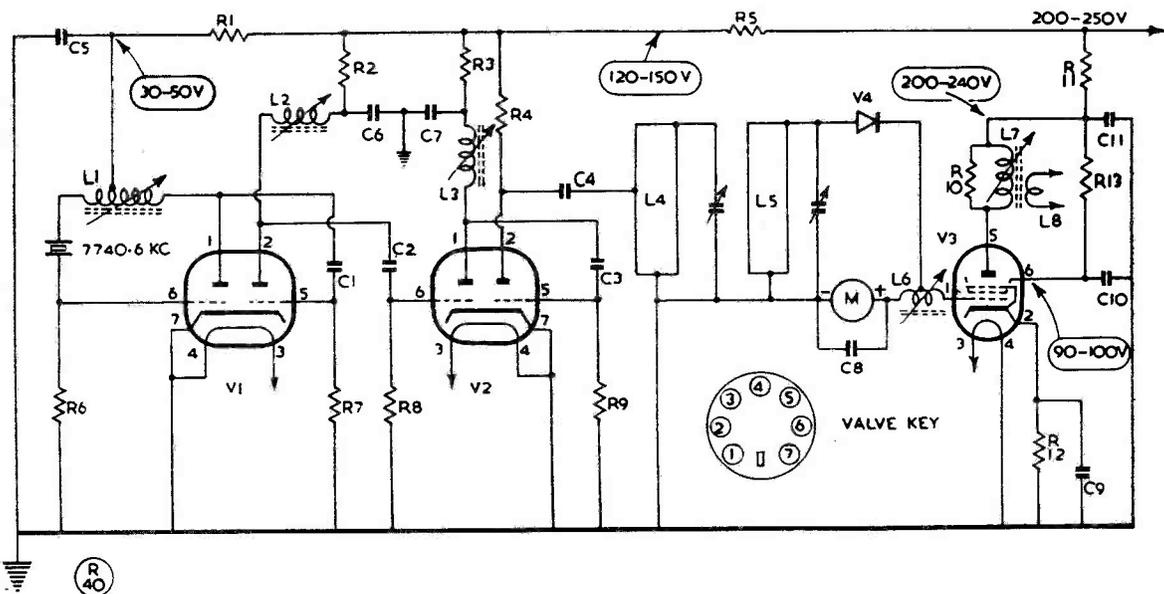
Fig. 1. Circuit of the Simplified 70-Centimetre Converter designed by G2DD. Elements marked L4, L5, are the brass strips for which dimensions are given in the coil table, the variable capacities across them being the air-spaced trimmers. The aerial coupling is arranged as described in the text.
