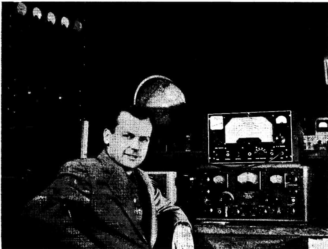
All those who heard or worked W0NWX, Newton, Iowa, during our Trans-Atlantic Tests on 160 metres earlier in the year will be particularly interested in this photograph. The gear includes a Lysco VFO driving a pair of 805's to 200 watts, and the receiver is an SX28A, modified as described in "Short Wave Magazine" for October, 1952. Outside, W0NWX has a 75 ft. mast supporting one end of an aerial 1,100 ft. long running across a valley.
