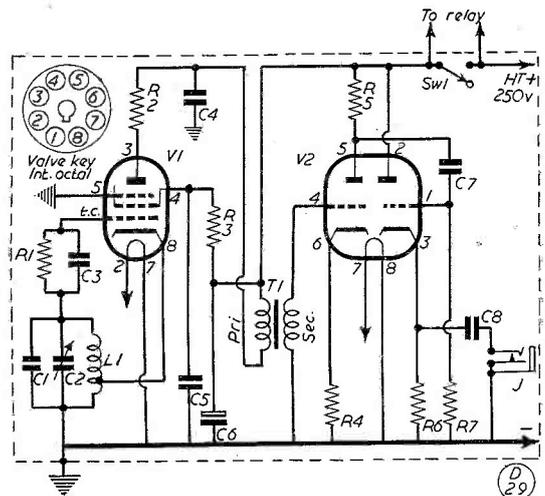
Fig. 1. Circuit of the all-band CW monitor suggested by G2NS.
