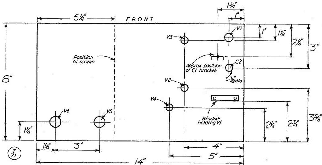
Fig. 3. Chassis drilling for the 14/21 mc Table Topper, which can be related to the half-rear view photograph. If the dimensions are carefully followed everything will fall nicely into place.
