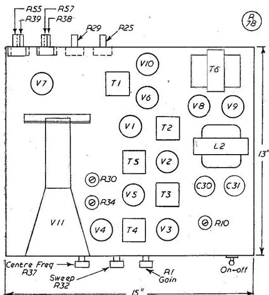
Fig. 4. Plan view of the general chassis layout, showing how the main parts can be disposed. Almost any convenient form of construction can be adopted.
