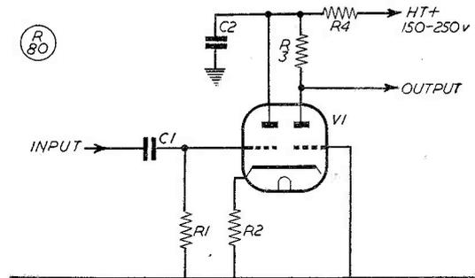
Fig. 6. Cathode coupled amplifier for the Panadaptor, values for which are given in the table.
