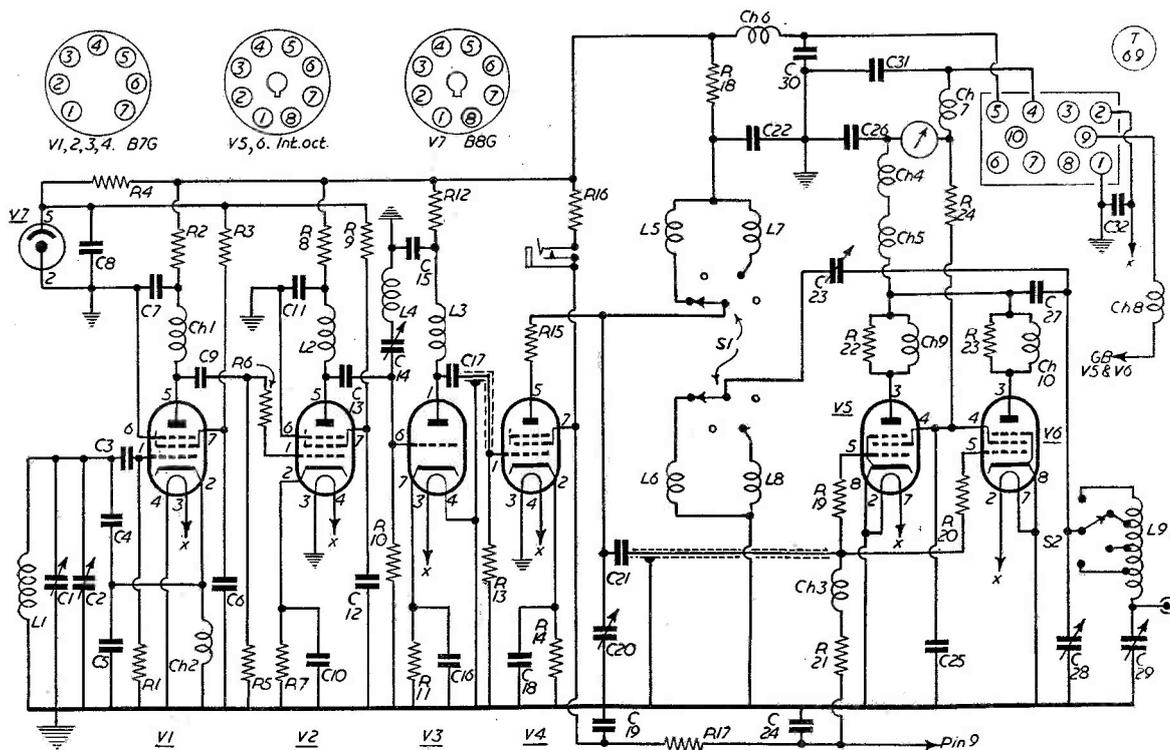
Fig. 1. Circuit complete of the Two Band Table Top Transmitter described in detail in this article. Ample drive is available for plate modulating the KT66's in the PA.
