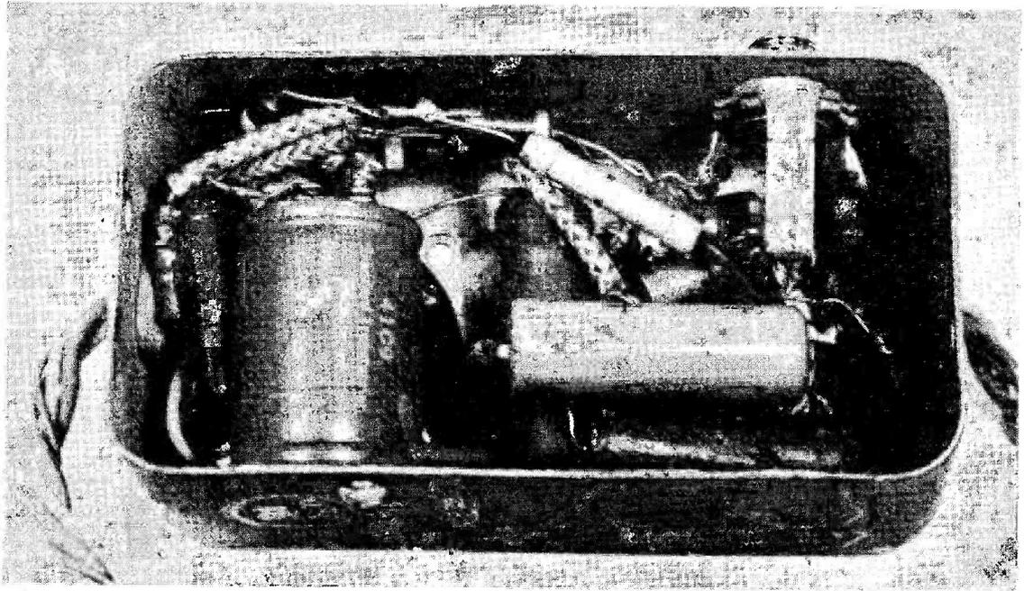
Construction underneath the little screen modulator unit discussed in this article.
