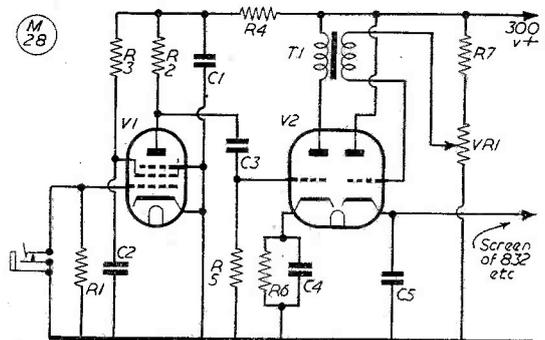
Fig. 2. Circuit complete of the screen modulator unit discussed by G3MY. Adjustment and operation are covered in the text, and values given in the table.
