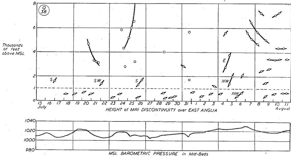
Fig. 1. Showing the reflecting layers which formed over East Anglia during the period July 15 to August 11. Occasionally they extended out along paths in various directions from the U.K., producing EDX conditions. The relevant dates are summarised in the Table.
