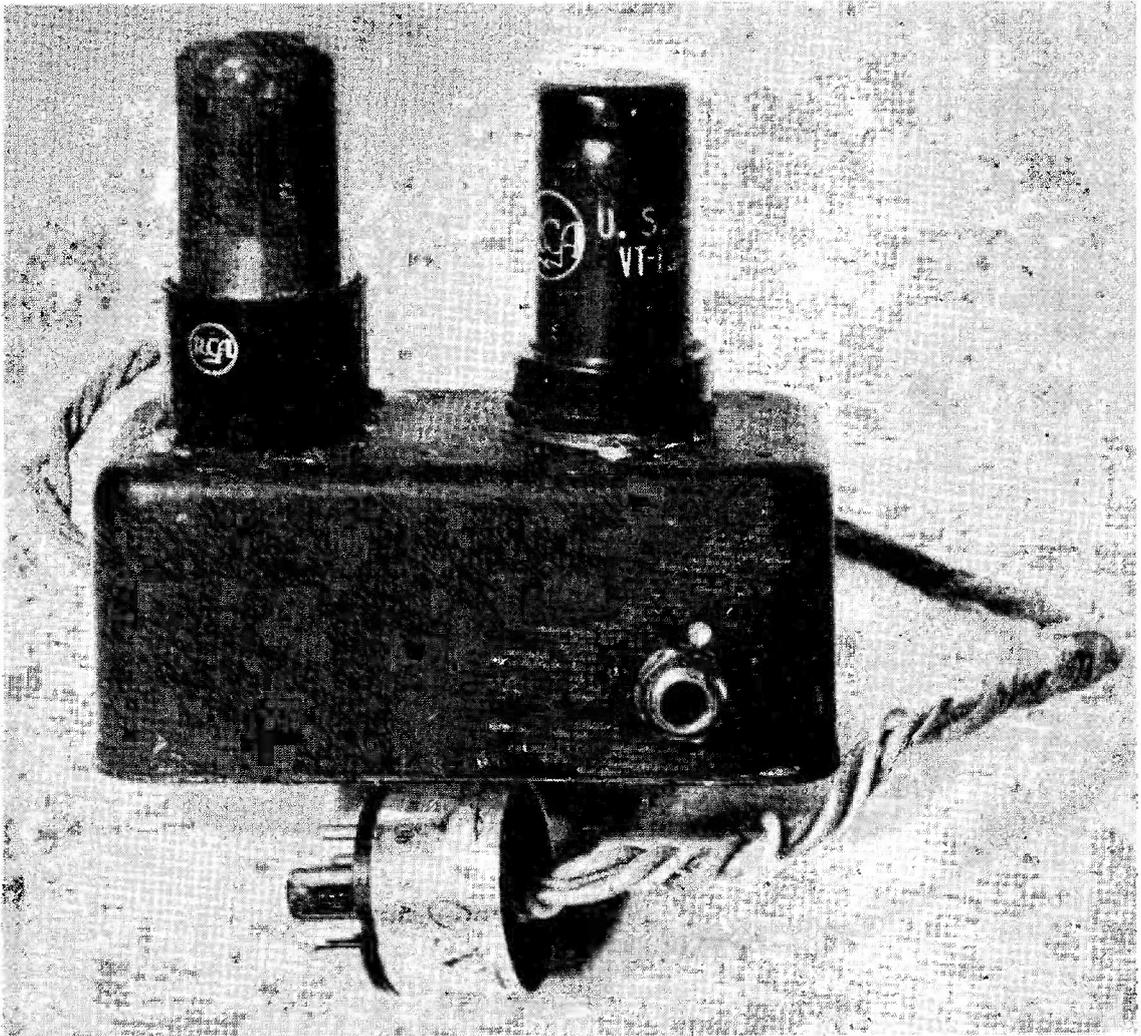
The screen modulator designed and described by G3MY. Though intended originally for portable gear, it is equally applicable to any PA stage using a tetrode—see Fig. 2 for circuit details.
