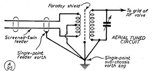
FIG. 3 Showing balanced shielded aerial transformer for terminating screened-twin feeder
