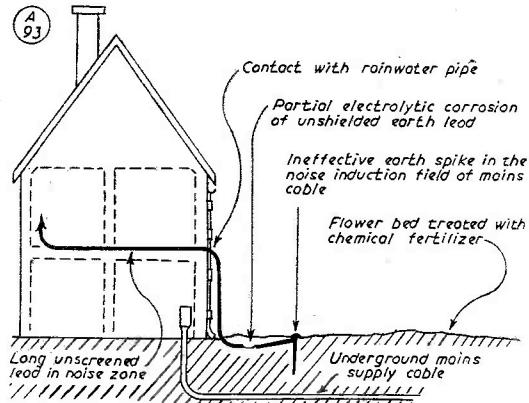
FIG 1b Typical installation of a poorly designed earthing system
