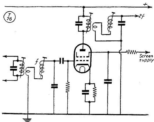
Fig. 1. Doubler stage as normally connected.
