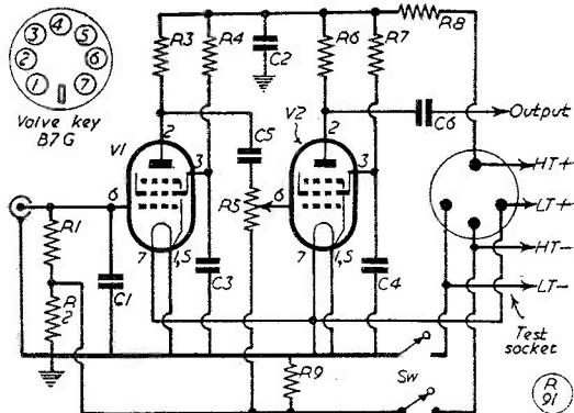
Circuit of the audio pre-amplifier, a simple enough arrangement giving reasonable gain and an absolutely hum-free output.
