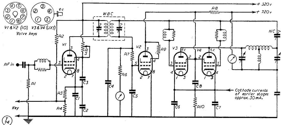
Fig. 3. Circuit of the 130-watt transmitter at VK2AWU, embodying the principles discussed in his article. The PA output can be so closely adjusted for a good keying characteristic that no thumps are audible at a nearby station tuned only a few kc off the transmission.
