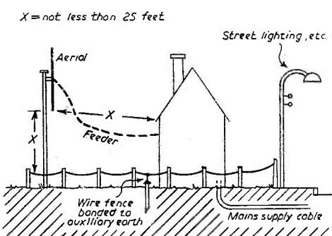
FIG 2B—TYPICAL VERTICAL AERIAL INSTALLATION
