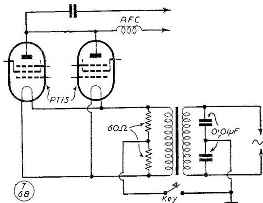
Modifications to the PT15 PA stage of the T.1154, as suggested by G2ASY. By these and the minor alterations to the driver stage as detailed in the text, he has been able to obtain a good T9 note.
