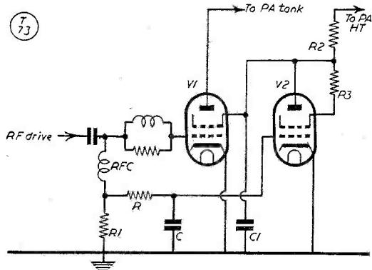
Fig. 2. Typical PA stage with screen-control valve. R is the "make" delay resistor; R<sub>1</sub>, PA grid resistor; R<sub>2</sub>, PA screen dropper; R<sub>3</sub>, 100 ohms,  $\frac{1}{2}$ w.; C, "make" delay condenser; C<sub>1</sub>, PA screen by-pass condenser; V<sub>1</sub>, PA valve(s); V<sub>2</sub>, the control valve, which can be a 6L6, 6Y6G or similar
