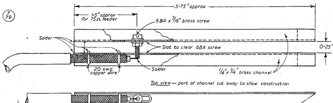
General arrangement of the 430 mc transmitter output coupling device suggested by G4MW. These are exploded views, and the general principles are fully discussed in the text. Lower sketch is side view.
