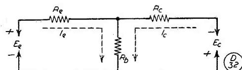
Fig. 1. The equivalent circuit of the transistor.
