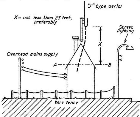
FIG 2D—INSTALLATION SUITABLE WHERE OTHER TYPES NOT PRACTICABLE
