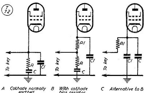
Fig. 1. Cathode keying of an early stage. Values would be: R, 100-500 ohms,  $\frac{1}{2}$ w.; R<sub>1</sub>, usual cathode bias resistor; C, "break" delay condenser, .05-0.5  $\mu$ F; C<sub>1</sub>, usual RF by-pass condenser.
