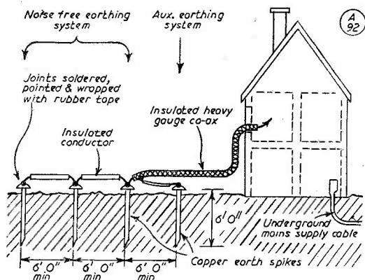
FIG 1a Typical installation of an ideal earthing system
