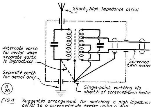
**FIG 4** Suggested arrangement for matching a high impedance aerial to a screened-twin feeder using a WBC.
