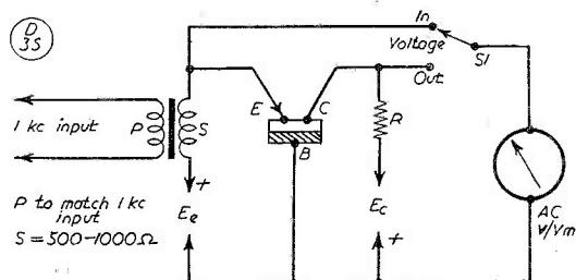
Fig. 4. The voltage amplification of a transistor can be directly checked by using the circuit shown here in the manner explained in the text.
