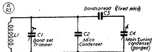
Fig. 2. The circuit actually involved in the BC-348 bandspread modifications explained by EI7D.
