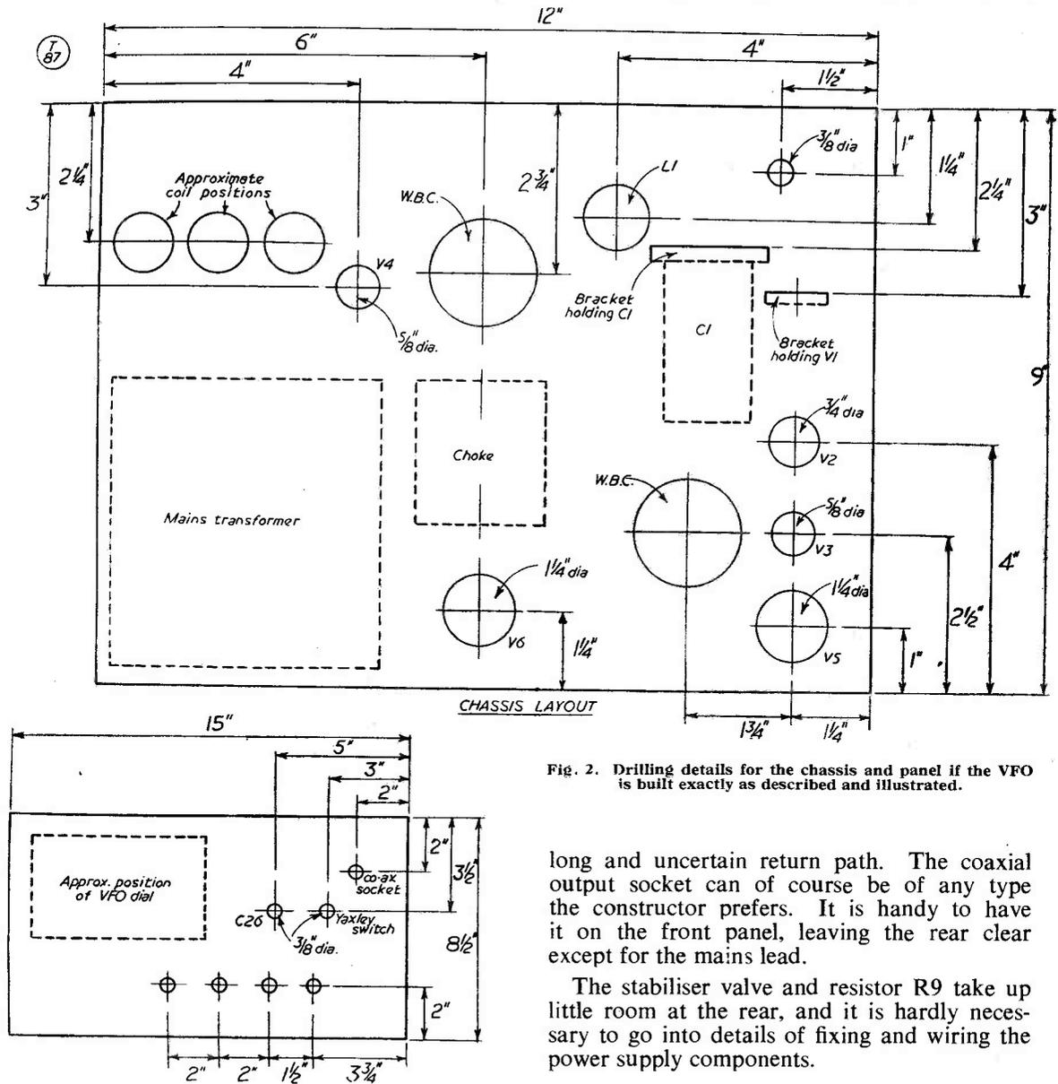
Fig. 2. Drilling details for the chassis and panel if the VFO is built exactly as described and illustrated.
