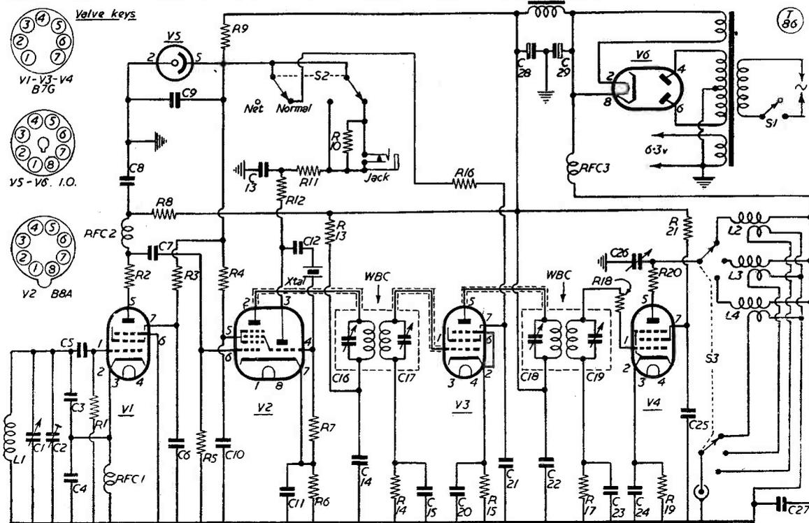
Fig. 1. Circuit of the Crystal-Mixer VFO Unit complete. The "net-normal" switch S2 allows the VFO to be set on frequency during reception. The wideband couplers WBC1 and WBC2 are surplus items (see text and table) or can be home-made in the manner described in recent articles on this subject. The general design of this VFO will appeal to the discriminating operator who wants the best.
