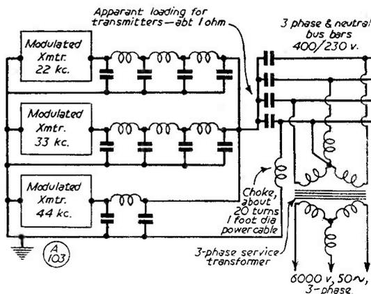
Fig. 1. Transmitter arrangement for the system of three-channel "wired wireless" developed by Eckersley in Liverpool in the 1930's. It was probably the first practical application of low-pass filters, and showed that an attenuation of 70-80 dB could be achieved between the three frequencies employed.
