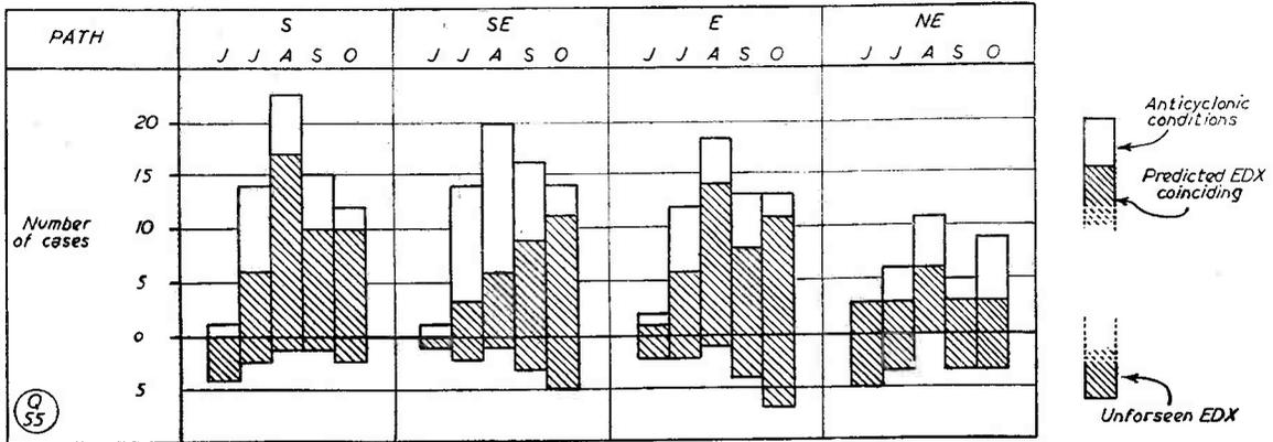
Fig. 1. This diagram gives an idea of the degree of success achieved during 1953 in the prediction of EDX/GDX possibilities by a study of surface weather charts. The shaded columns are estimated results and are drawn over clear columns showing weather chart predictions. The residual clear portions represent prediction failures, while shaded areas below the zero-line are missed openings. The limitation of surface weather chart prediction is well brought out.
