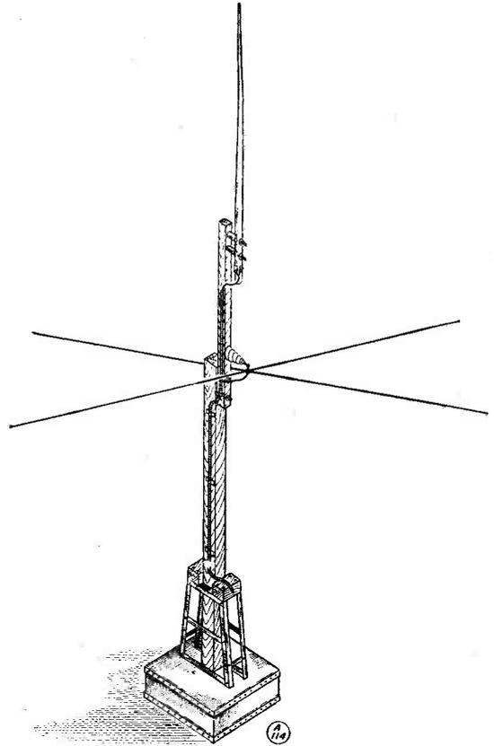
The constructional detail sketch for G6VC's Ground Plane mounting.
