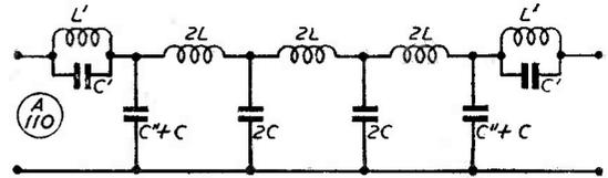
Fig. 15. Filter complete for the requirement called for at point "X" in Fig. 13. Values are : 2L, 0.46 μH ; 2C, .00018 μF ; C' + C, .00014 μF ; C', .000097 (.0001 μF near enough) ; L', 0.14 μH.
