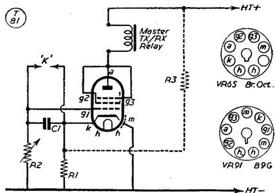
Circuit of the key-controlled change-over system devised by G80D, and fully explained in the text.
