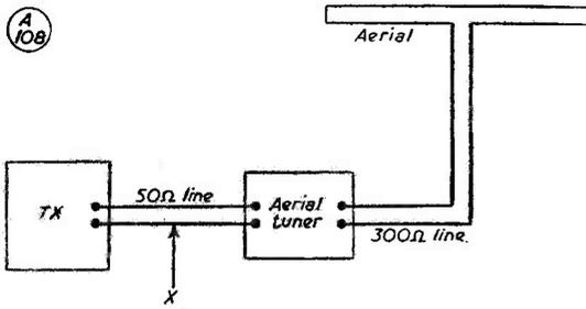
Fig. 13. Practical case in which a filter is required at point "X"
