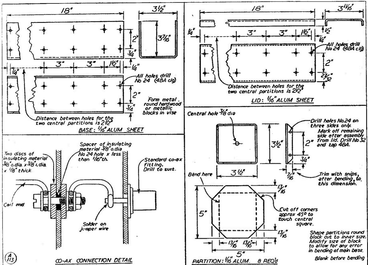
Fig. 18. Construction of the screening box for the filter shown at Fig. 15, with inter-connection details.
