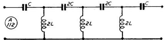
Fig. 17. A high-pass filter, in which positions of C and L are reversed. For working into 50-ohm line, and designed to give a cut-off frequency of 35 mc, values would be: 2L, 0.46  $\mu\text{H}$ ; 2C, .00018  $\mu\text{F}$ ; C, .00009  $\mu\text{F}$ .
