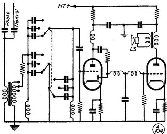
Fig. 2. The receiver, or "Selector" circuit, giving a choice of three programmes from over the power lines, without mutual interference.
