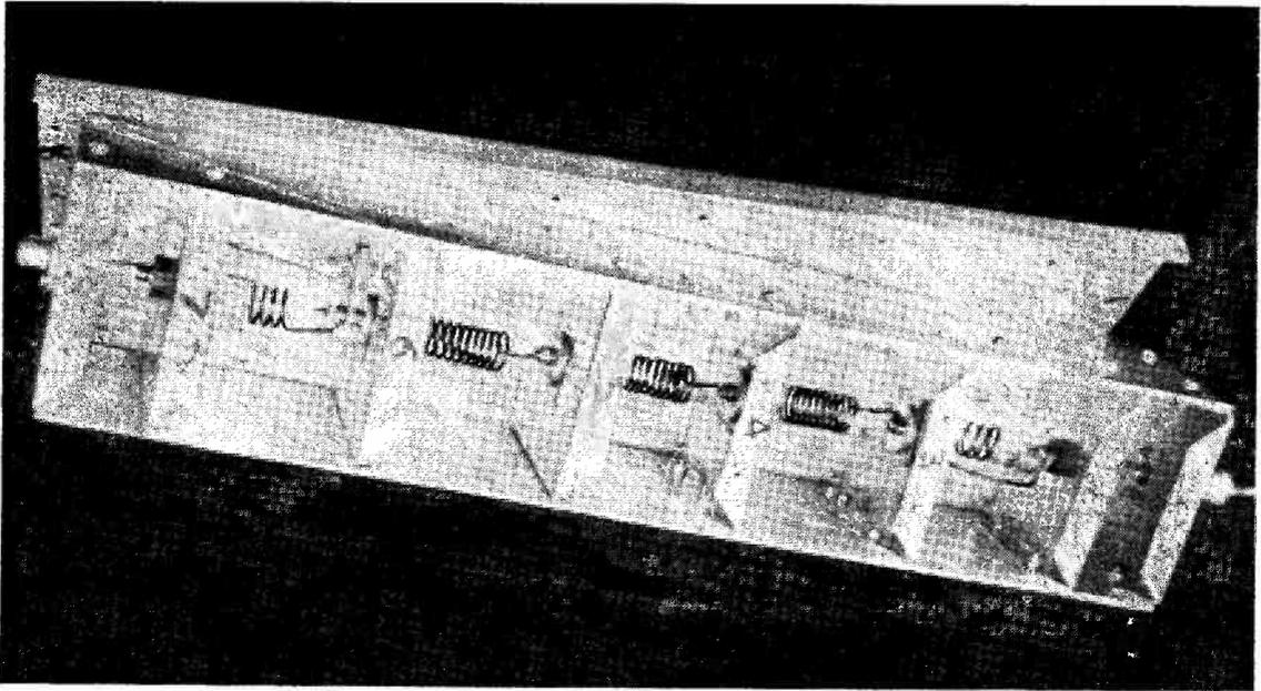
Method of construction of the complete filter shown at Fig. 15. Details of the coupling capacity used are given in the text, and constructional data for the screening box in Fig. 18.
