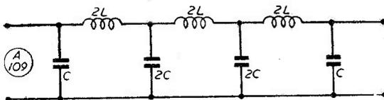
Fig. 14. For the case in Fig. 13, a 3-section Pi filter would be as shown here. Values are : 2L, 0.46 μH ; 2C, .00018 μF ; C, .00091 μF.
