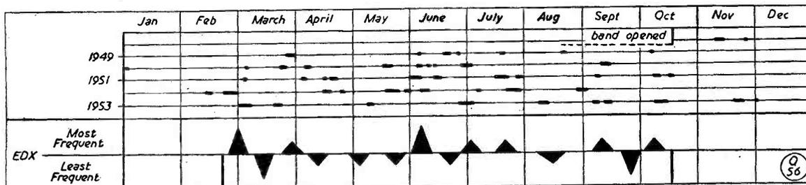
Fig. 2. Showing EDX openings actually encountered during the last five years. Upright triangles represent the periods of the year that have most frequently brought openings. Triangles pointing downwards show the periods during which EDX occurred the least. From this, it would seem that VHF operators should take their holidays in April, May or August!
