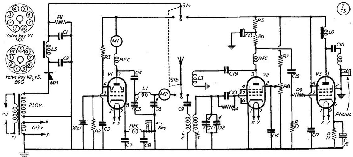
Circuit of the transmitter/receiver as used by G3AHO for CW operation on the 40-metre band. It is essentially a low-power CC transmitter (V1), with an O-V-1 receiver (V2, V3). Particularly interesting results should be possible on the LF bands, where the receiver would be more effective.
