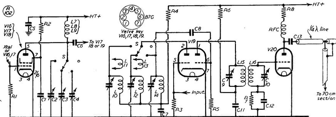
Fig. 4. The crystal oscillator-multiplier section, in which the circuitry of V16 represents the three stages V16-V18 (see Fig. 1.) Stages V19, V20 produce the injection frequency for the 430 mc converter; the injection at 116 mc for two metres is taken off V19. Two different crystals are used (see text) to arrive at the correct output frequencies without beats in either band or in the IF tuning range.
