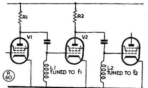
Fig. 3. Circuits in staggered pair.
