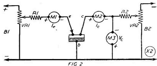
Fig. 2. Circuit for measuring the current amplification factor of a transistor. This is the essential value for determining its goodness.
