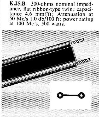
**K.25.B** 300-ohms nominal impedance, flat ribbon-type twin; capacitance 4.6 mmf/ft; Attenuation at 50 Mc/s 1.0 db/100 ft; power rating at 100 Mc/s, 500 watts.
