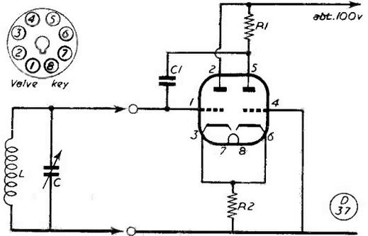
Circuit of the two-terminal oscillator. This will go off with almost any value L, C, and is the basis of the method of measurement suggested in the article. Readings are obtained against the station frequency meter or a calibrated receiver. The unknown inductance is connected as L in this circuit.
