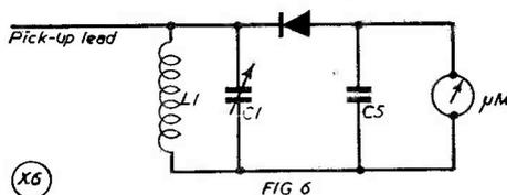
Fig. 6. It is a great advantage to have a sensitive RF indicating device available when setting up transistor transmitter circuits. This is the usual crystal-diode arrangement, but in this case it calls for a low-range microammeter and fairly tight coupling to the aerial lead on the transmitter. The usual rules apply as regards coupling, and maximum readings off the aerial indicate greatest RF output from the transmitter.
