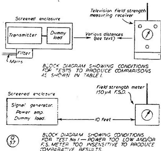
Fig. 1. Diagrams showing the test set-up, as explained in the text, to determine the relative screening value of different materials.
