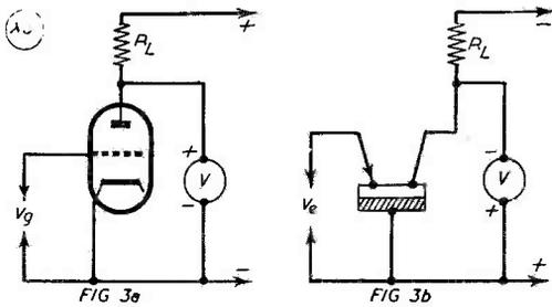
Fig. 3. Comparison of the phase relationship between the input and output in a valve (A) and a transistor (B), connected as an amplifier.
