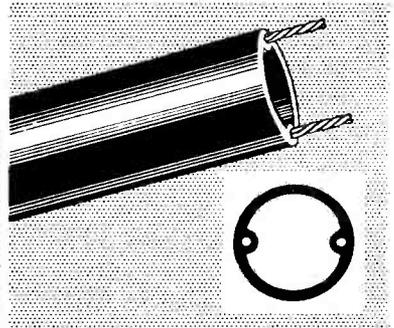
**K.35.B** 300-ohms tubular twin feeder with stable characteristics in varying weather conditions. Capacitance 4.0 mmf/ft; attenuation at 50 Mc/s, 0.92, db/100 ft; power rating at 100 Mc/s, 550 watts.
