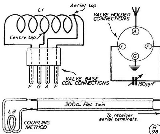
Fig. 2. Circuit and values of the HF signal booster as applied to the 14 and 28 mc bands for any usual type of receiver. The parallel condenser of 150  $\mu\mu\text{F}$  has two settings, one for each band; for 14 and 28 mc, coil L1 should be 6 turns of 14g. wound to a diameter of 1.1ins. and about the same length; L2 is a 2-turn coupling loop in insulated sleeving, inserted into L1. Taps are taken out as explained in the article.
