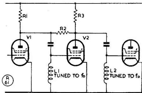
Fig. 4. Circuit for a feed-back pair.
