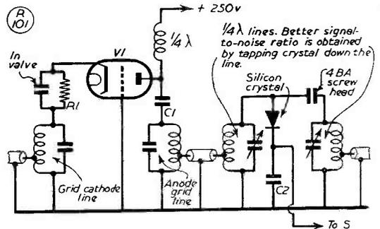
Fig. 3. The 70-centimetre front end for the VHF receiver. V1 is a GL446A ground-grid triode, with a silicon-crystal mixer used in a quarter-wave line input/output circuit. The input and output are actually tapped down the line in each case to get a better signal-to-noise ratio. The detail for the construction of the 430 mc RF and mixer stages will be given in the second part of the article, with all coil values.
