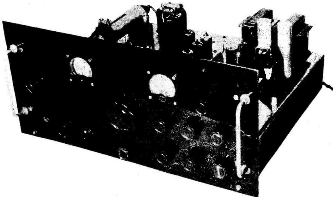
General appearance of the G2BVW two-channel VHF receiver, designed for the 144 and 430 mc bands. A block layout appears in Fig. 1., and an interior view of the receiver was shown on p.304 of the July 1953 issue.
