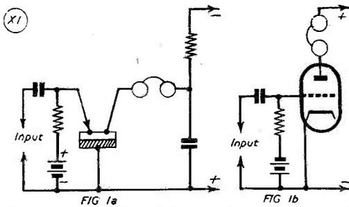
Fig. 1. Comparing the circuitry of a transistor with a valve in the ordinary audio connection.
