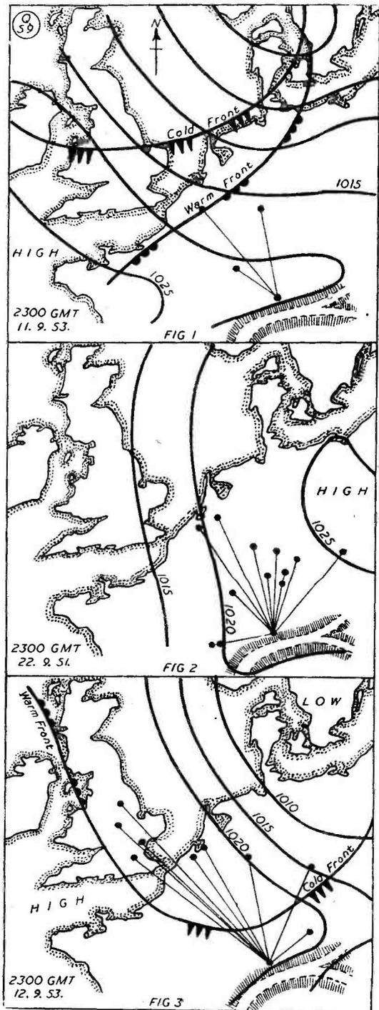
Figs. 1-3 above show how active "warm fronts" can screen off VHF DX working, and how the direction of DX working from HB tends to lie parallel to the isobars (lines of equal barometric pressure). HB9IV was on Mount Pilatus in September 1951 (Fig. 2.) but on that occasion did not get into the U.K.
