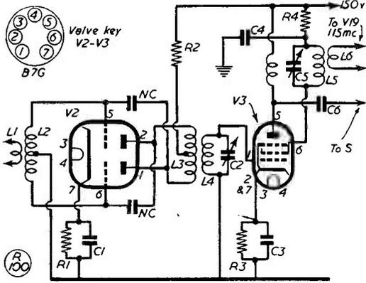
Fig. 2. Two-metre converter section of the G2BVW receiver. Valves are 6J6 for V2 and 6AK5 (or 6AK5) for V3.
