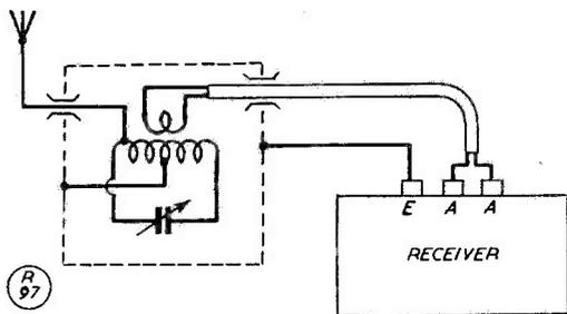
Fig. 1. Method of connecting the external tuned circuit to any usual type of communications receiver fitted with a doublet aerial termination.
