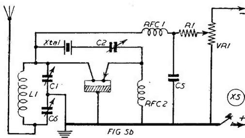
Fig. 5. Crystal controlled transistor transmitter circuits as evolved by G3HMO in the course of his experiments with home-made transistors. It will be noted that the C1, L1, C6 network is the usual Collins-coupler arrangement. Setting up procedure is discussed in the article.
