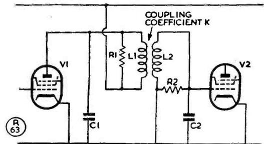
Fig. 6. Transformer inter-stage coupling; values and the significance of the coefficient K are discussed in the text.
