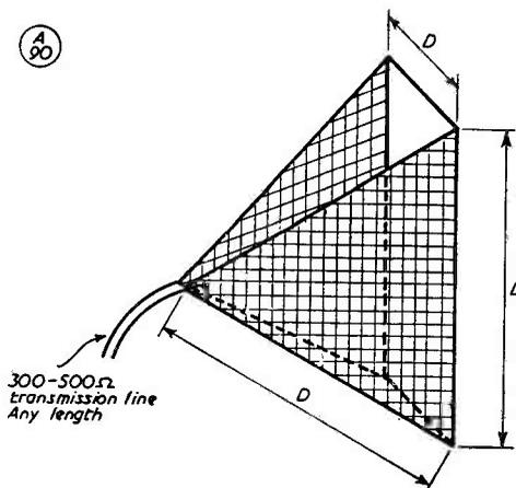
Fig. 1. The modified 60° Horn Beam. The vertical triangular areas are covered with wire mesh and are insulated from each other. A beam of this sort can be fed with 300-ohm line, and if built for two metres, can be used "third-harmonically" on 430 mc without any alteration, the gain increasing as the frequency goes up. The feeder connection is made to the mesh sections.
