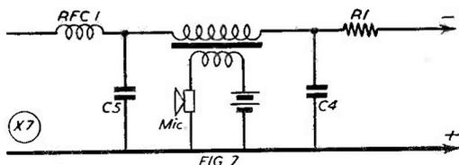
Fig. 7. With either of the transmitter circuits of Fig. 5 (A) or (B) modulation can be applied by the method shown here. With a strong oscillator and the crystal holding well, it becomes correspondingly more difficult to obtain full modulation. In general, the rules against modulating a crystal oscillator also apply to transistor transmitters, and an obvious line of development is a transistor PA driven from a transistor GO, with two more transistors operating as speech amplifier-modulator.
