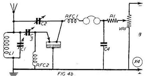
Fig. 4. A simple one-stage transistor receiver with reaction, controlled by C2, showing alternative methods of connecting the emitter (circuits A or B). In both circuits, L1/C1 are proportioned for the band to be tuned.
