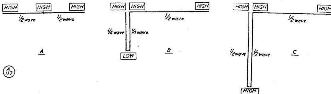
Fig. 1. Illustrating the well-known Zepp aerial system, familiar in amateur working. As shown at (b) and (c), the length of feeder affects the impedance to be matched, and hence the method of feeding, at the transmitter end. It will also be seen that (a) is an "opened-out" version of (b), and is the best way to think of the Zepp.
