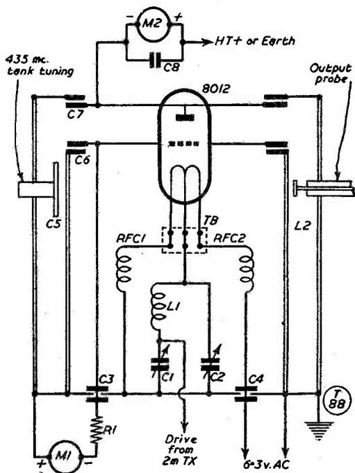
Fig. 1. Electrical cross-section through the 70-centimetre tripler, showing also the circuit arrangement. L1, C1, C2, comprise the 2-metre tuning assembly.
