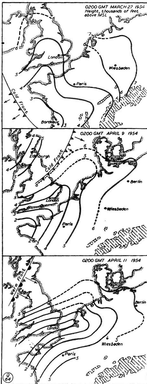
Fig. 1. These charts show the refraction discontinuities that developed during this period. VHF reflection from the first one is mainly to the South and South-Easterly directions, probably when there was little activity to exploit the possibilities. The second shows how even a weak cold front can break up a reflecting layer. For a warm front the break-up usually occurs in advance of the front, as in the lower sketch.
