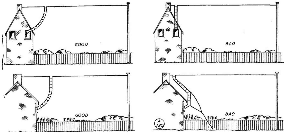
Fig. 4. Suggesting feeder layouts for a Zepp system. The aim should be to get the high-impedance feed point at the house end as well in the clear as is reasonably possible, with an easy run for the feeder line.
