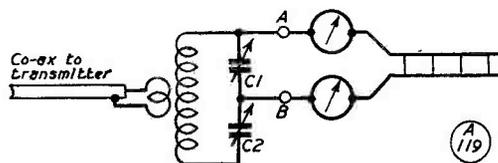
Fig. 3. When it is convenient or necessary to use a coaxial coupling system between transmitter and aerial tuning unit this is the method by which a Zepp system can be fed; C1, C2, comprise a movable tapping point for the B-leg of the feeder line, the adjustment being to obtain equal, and highest possible, reading in the RF meters consistent with proper loading of the PA stage.
