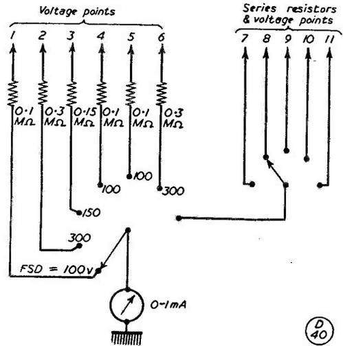
Fig. 1. Wiring diagram for voltage measurement at eleven separate points in a circuit, and showing how a second rotary selector can be switched in if the first selector has insufficient switching positions. The basic idea is to make one 0.1 mA meter, with suitable series resistors, function as a check voltmeter on circuits which are not normally metered continuously.
