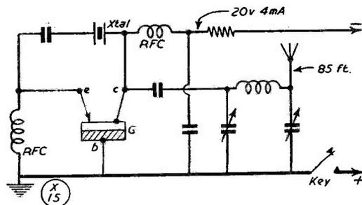
Fig. 1. Transistor circuit in use by G3IYX on 1822 kc, with an 85-foot aerial and Collins coupler; his input is 85 milliwatts and he radiates a very good local signal up to 10 miles or so, with a 28-mile reception report as best DX so far. G3IYX is regularly active from Bradwell in North Bucks and can be found on the air most evenings.
