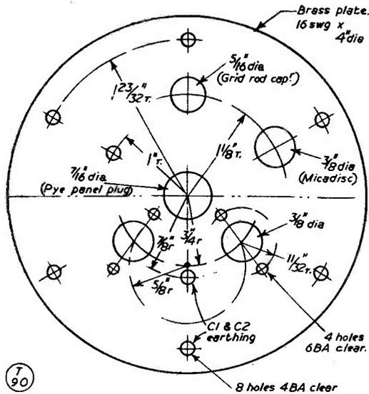
Fig. 3. Some accurate metal work is called for in the construction of the 430mc tripler. This is the drilling template for the bottom cover plate.
