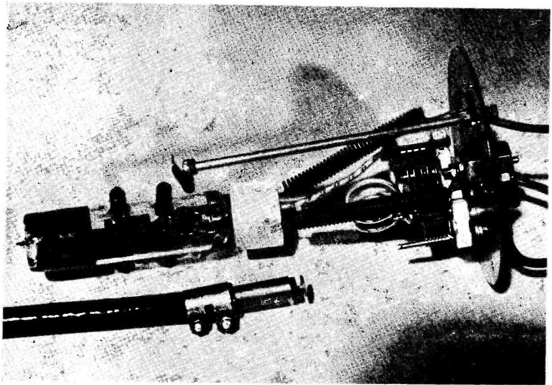
Exploded view of the 8012 70 cm tripler as described by G3HAZ. The two-metre drive circuit is the assembly on the right, bolted to the circular plate. The 8012 is a glass triode with plate and grid connections brought out on two sides of the envelope; in this design, the valve is mounted by its filament pins on a 3-way porcelain connector (centre), the spiralled leads being the RF chokes in the filament supply — see circuit Fig. 1. In the foreground is the RF output probe for 70 cm.
