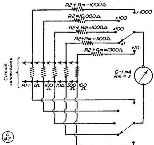
Fig. 3. Wiring layout for current measurement at five separate points in a circuit, the principle being the same as in Fig. 1, except that parallel resistors are involved. The switching motions can be carried out by a 2-pole 5-way rotary selector.
