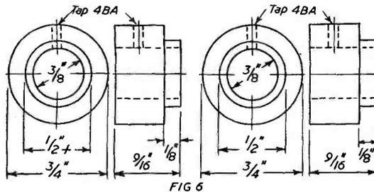
Output probe and output tuning capacitor bushes
