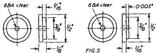
Grid and anode capacitor plate insulating bushes
