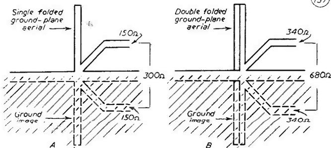
Fig. 2. Showing the equivalent radiating system for single and double-folded ground plane systems, with feed impedances.
