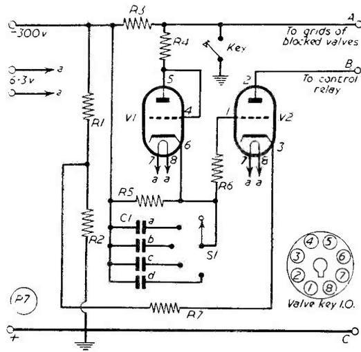
Fig. 1. Circuit of the control section in the change-over system discussed by G3EFI. V1, V2, can be a single 6SN7, one half V1 connected as a diode, or a separate triode and diode can be used. The unit requires a negative supply of about 300 volts.
