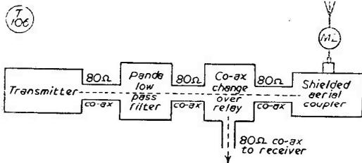
Fig. 4. Block schematic of the layout complete on the output side of the 160-metre transmitter—an arrangement contributing very largely to the elimination of BCI and TVI.
