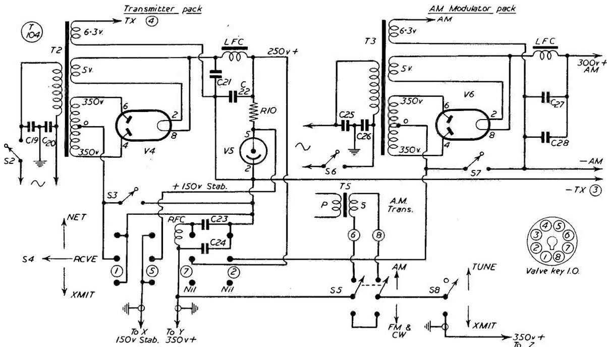
Fig. 2. Suitable power packs, which are separate units, for the Safe Top Bander. The control switching is also shown. If NBFM only were to be used — quite permissible and entirely satisfactory in this application — the amplitude modulator section would not be required, dispensing with the circuitry and switching round rectifier V6.
