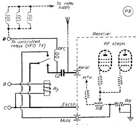
Fig. 2. Circuit of the relay unit, giving muting of the receiver (aerial shorted to earth on "mark," with aerial relay open) and in-step control of the transmitter relays. On "space," the aerial relay (not shown) closes, and the receiver is at a sensitivity determined by R8, R9. The leads to aerial and earth terminals on the receiver itself must be kept as short as possible to minimise direct pick-up of the radiated signal.
