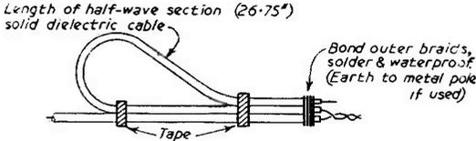
FIG 2 Balun impedance transformer for 145 mc
