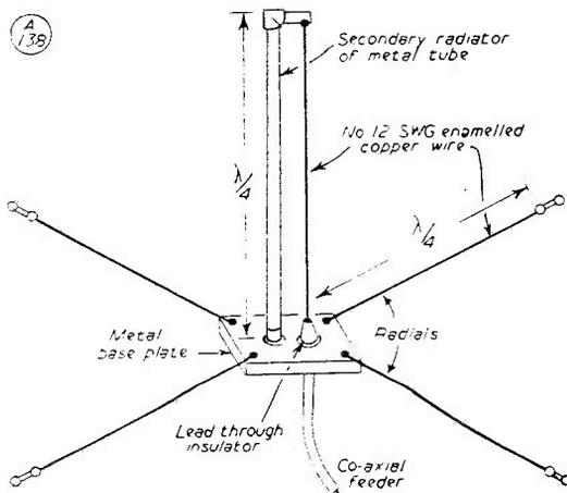
Fig. 3. A folded ground-plane, built on the same principle as a folded dipole. In the case illustrated, it calls for a feed line of 150 ohms surge impedance and gives a broad-band characteristic, which is an added advantage.
