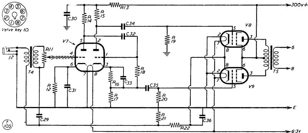
Fig. 3. A simple amplitude modulator for the 160-metre transmitter described in the article. This gives plate-and-screen control of the 807 PA. V7 is a 6SN7 and V8, V9, are 6V6; note how the energising current for the carbon microphone at J2, T4, is supplied by tapping off the cathodes of the 6V6's.
