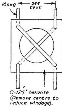
FIG 4 Transposition piece
