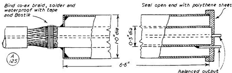
Fig. 7. Balun for 430 mc. The inner tube should be chosen to give a wall thickness making a tight fit over the polythene insulation of the cable used.
