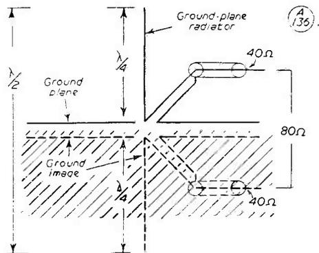
Fig. 1. The equivalent radiating system for the usual type of ground-plane aerial, which demands a low-impedance feed, sometimes awkward to achieve.
