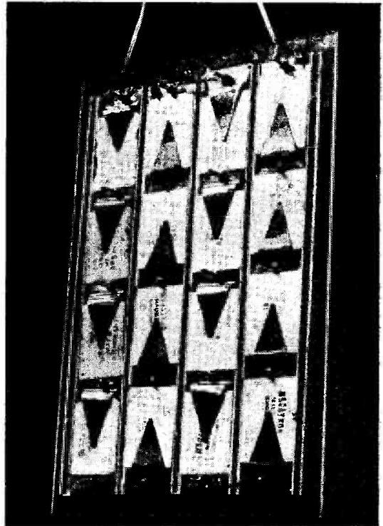
Rear view of the photo-cell battery constructed by G3HMO, shown as P in the circuit at Fig. 1. The triangular pieces are cut from springy brass sheet, set to give good contact with the back of each cell. The perspex sheet is about 8 ins. wide by 10 ins. deep, approximately the size of an ordinary window pane.
