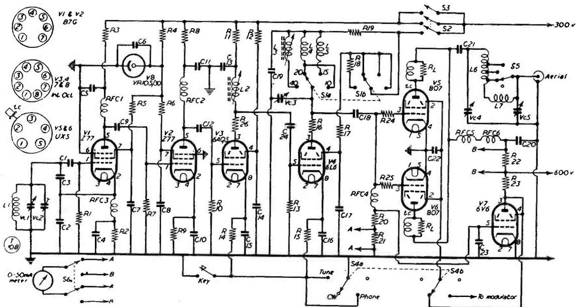
Fig. 1. Circuit of the RF section of the VQ2AH transmitter as described. The driver section V1, V2, V3 can be built and tested as a separate unit before fitting to the main chassis. The switched coils in the plate of V4 give output on three HF bands, operation of the PA on 10 metres being obtained by doubling from the 20-metre drive at L4. The 807's in the PA are in parallel and modulation is by screen control.
