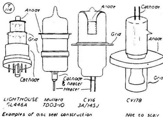
Fig. 4. Outline drawings (not to scale) of valve types designed for concentric line circuits at UHF.
