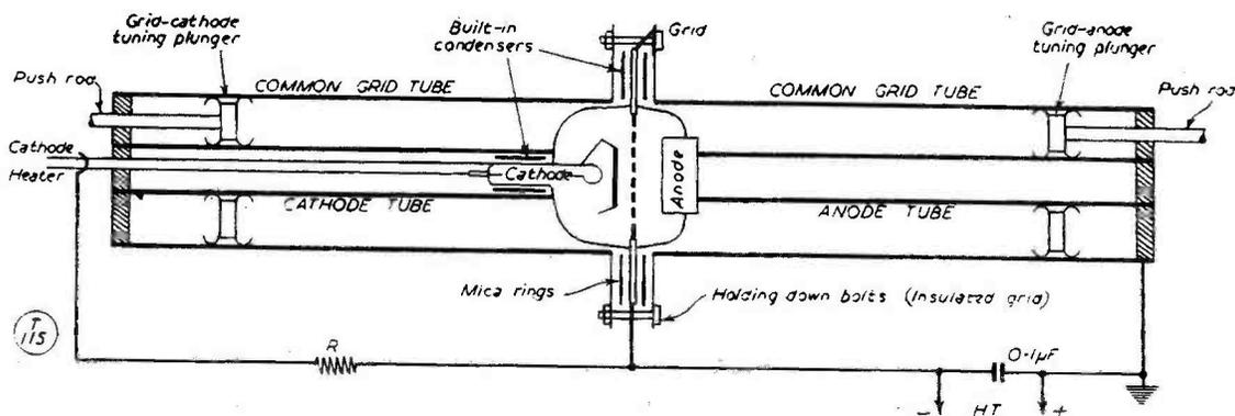
Fig. 5. The basic coaxial or concentric-line oscillator circuit as a logical development of Fig. 3. This is a sketch of the electro-mechanical arrangement, in section, the actual construction being cylindrical.
