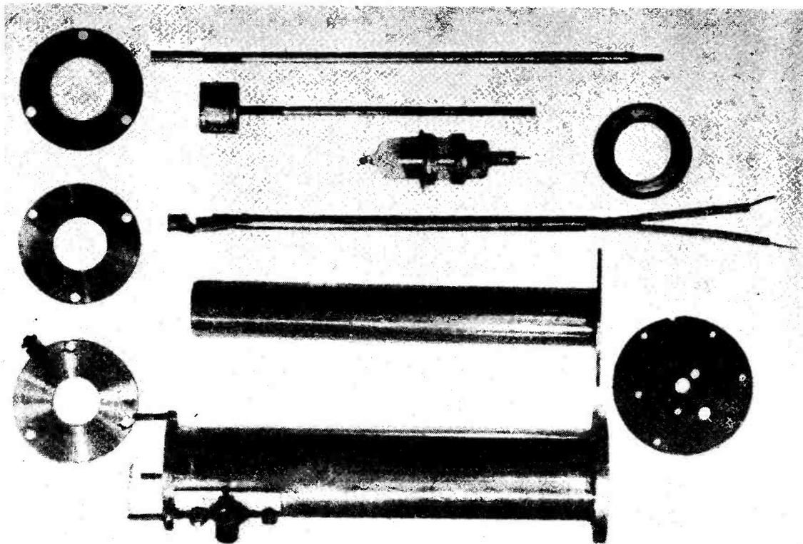
All the parts for the 25-centimetre oscillator, which make up to the assembly shown in the accompanying photograph. The valve is a Mullard TD03-10 (ME-1000) and a detail drawing of the oscillator appears in Fig. 5A.
