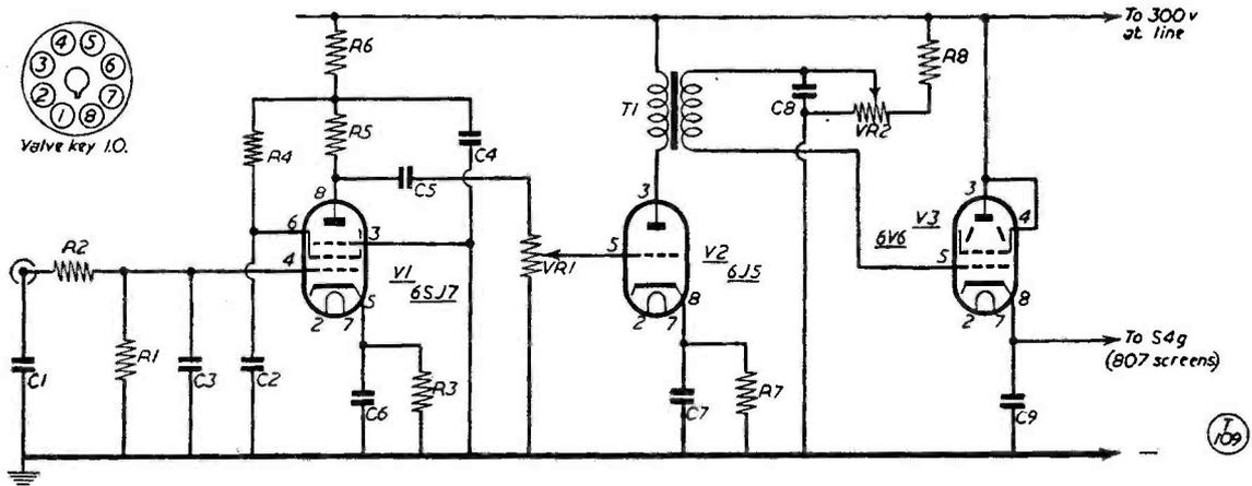
Fig. 2. Screen-control modulator unit for the VQ2AH transmitter. This arrangement will give full modulation of a 70-watt carrier, with good quality speech and easy adjustment, provided the screen voltage of the 807 PA, controlled by VR2, is correctly set.
