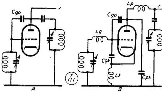
Fig. 1. (A) shows the basic circuit of the conventional TPTG oscillator. At (B) is the TPTG as it appears at VHF, showing the effect of lead inductance, inter-electrode and stray capacities.
