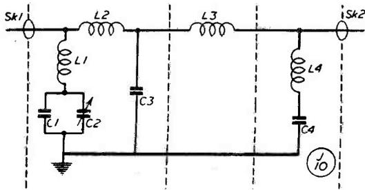
Fig. 1. Circuit of the filter suggested by G8PG. Values are: C1, 100  $\mu$ F silver mica; C2, 50  $\mu$ F air trimmer; C3, 440  $\mu$ F silver mica; C4, 120  $\mu$ F silver mica; L1, L4, 13 turns spaced 1-½ ins.; L2, L3, 20 turns spaced 2 ins.; all coils are ½-in. diameter. Sk1, Sk2, are coax sockets.
