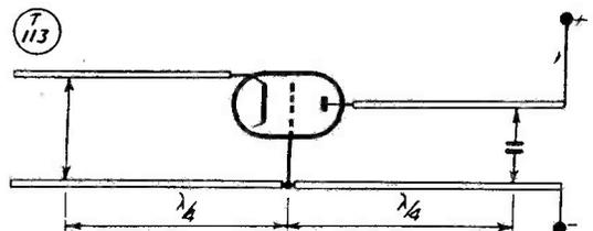
Fig. 3. The next step is the substitution of tuned quarter-wave lines for the conventional coil-condenser combination, as a means of reducing unwanted L and C components.
