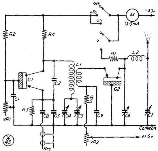
Fig. 3. VFO-PA transistor transmitter now in use at G3CSZ, of which details are given in the text. He uses the VFO circuit suggested by G3CCA, while the PA arrangement is that devised by G3HMO. The result is a handy, stable TTX for 160-metre working; in G3CSZ's case, the transistors are home-made but GET-2's could very well be used.
