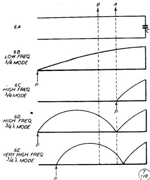
Fig. 6. Showing how quarter-wave and three-quarter wave modes of oscillation can be obtained over the same pair of lines. As explained in the text, this is one of the most important attributes of the concentric line principle.
