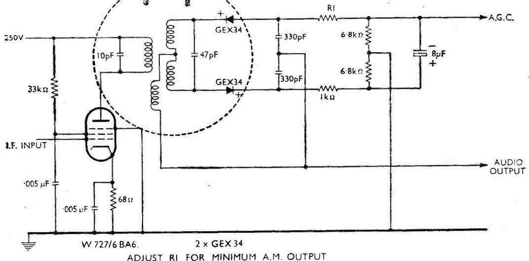
**Transformer Design.** Although the circuit shown above is conventional, an I.F. transformer designed for use with thermionic diodes is not necessarily the most suitable for germanium diodes. A suitable design of transformer has been evolved at the G.E.C. Research Laboratories, details of which are available on request,
