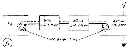
Fig. 3. Incorporating the filters in the transmitter output, as described in the article. If the filters are working properly, operation should be possible on both LF bands without risk of TVI by 14 mc break through.
