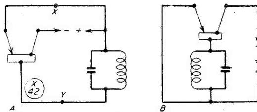
Fig. 2. An explanation of the base-tuned transistor oscillator in terms of the amplifying properties of a transistor rather than negative resistance. Circuit (A) shows direct feedback from collector to emitter. Circuit (B) is the same as (A) but is the more conventional layout of a base-tuned oscillator.
