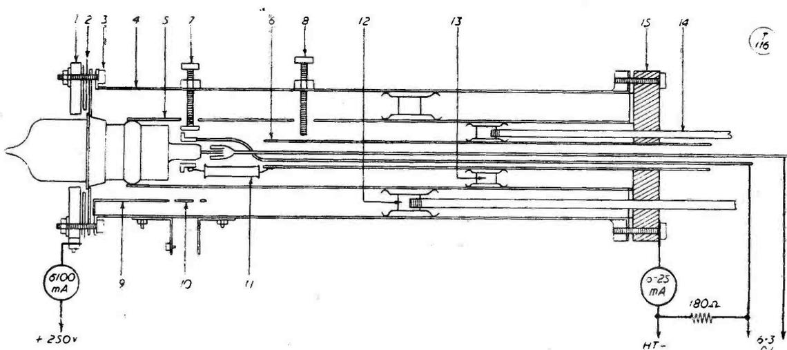
Fig. 5A. Detail of the 25-centimetre oscillator designed by G5RZ and illustrated in the photographs. This is a sectional view ("cut in half down the centre") showing both the mechanical arrangement and the electrical layout and connections - see key for details, and refer exploded view photograph.
