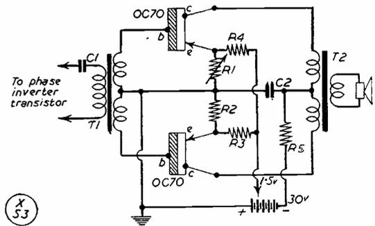
Fig. 6. Basic circuit of a Class-B push-pull transistor amplifier which will give more audio output than the Class-A connection used in the receiver as described. Values are: C1, 1.0  $\mu$ F; C2, .01  $\mu$ F; R1, R2, R5, 2,000 ohms; R3, R4, 4,700 ohms. Note that with a centre-tapped input transformer, phase inversion would not be required.
