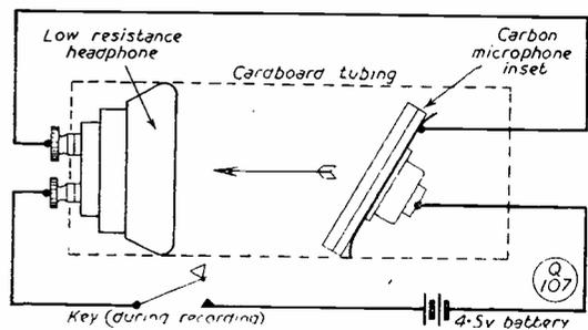
Fig. 2. To obtain the CW recording on the tape, a feed-back hummer is used, the audio tone so produced being picked up by the microphone of the tape recorder. There are other ways of getting the CW signal on to the tape, such as by using the output of an audio oscillator plugged directly into the recorder microphone circuit. Whatever method may be used, the recorded CW is a true reproduction of the operator's own keying characteristic.
