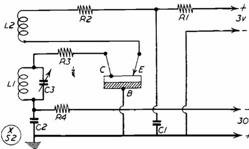
Fig. 5. Alternative oscillator circuit for the BFO, using a MW coil having a reaction winding. R2, R3, are inserted to give good waveform, and values are: C1, C2, .01  $\mu$ F; C3, tuning; R1, 12,000 ohms; R2, R3, 4,700 ohms; R4, 10,000 ohms.
