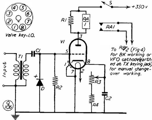
Fig. 1. The triggering circuit for the G2NS auto-sender using a tape recorder. The tape output, with the recorded CW signals, is fed to T1, relay RA1 then operating to follow the recorded keying. The contacts RA1 control the actual change-over and keying relay, RB/2 in Fig. 4.
