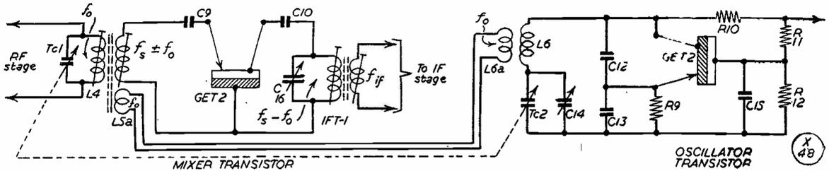
Fig. 1. The frequency changer stage with link coupling is an alternative method of injecting the oscillator output into the mixer transistor. The link is adjusted for optimum results. In this circuit bias voltages have been omitted for simplicity — see Fig. 7 for detailed arrangement.
