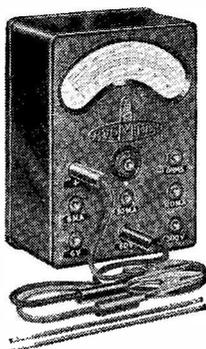
A conveniently compact 2½-inch moving coil precision meter for making D.C. measurements of milliamps, volts and ohms. The total resistance of the meter is 100,000 ohms, and full scale deflection of 300 v. or 600 v. is obtained for a current consumption of 3mA. or 6mA. respectively
