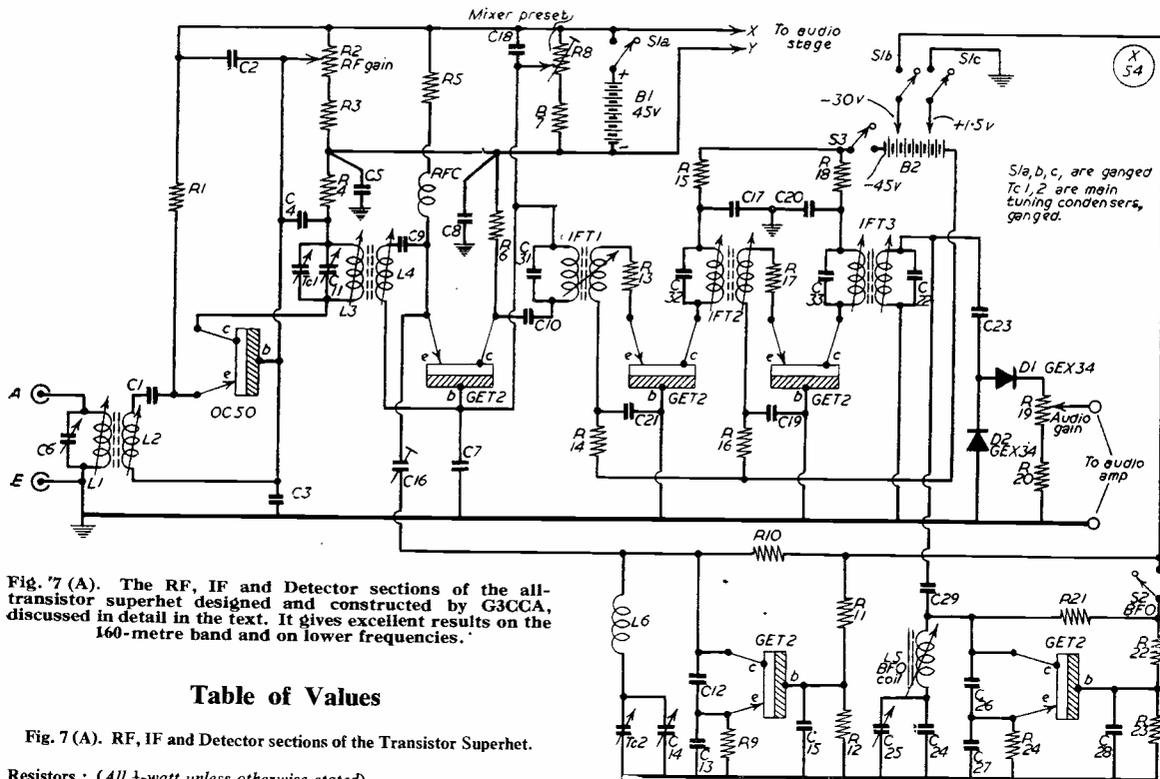
Fig. 7 (A). The RF, IF and Detector sections of the all-transistor superhet designed and constructed by G3CCA, discussed in detail in the text. It gives excellent results on the 160-metre band and on lower frequencies.
