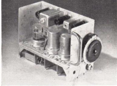
We can now offer this self-contained Unit, comprising 6 valves: 2-6BA6, EB91, VR137, EF54, EF54. Two I.F. stages and separate local oscillator, also Muirhead graduated vernier drive assures easy tuning.
