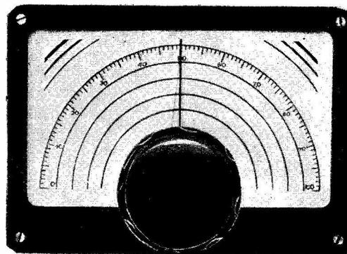
**FULL VISION DIAL No. 598.** The epicyclic ball bearing drive mechanism is smooth and free from backlash and has a reduction ratio of approximately 10 to 1. Escutcheon measures 6" x 4½", in ripple black finish. Scale 0-100 over 180. Spare scales included. PRICE 24/6.
