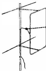
**SINGLE SLOT** Portable Antenna with 2 Reflectors
