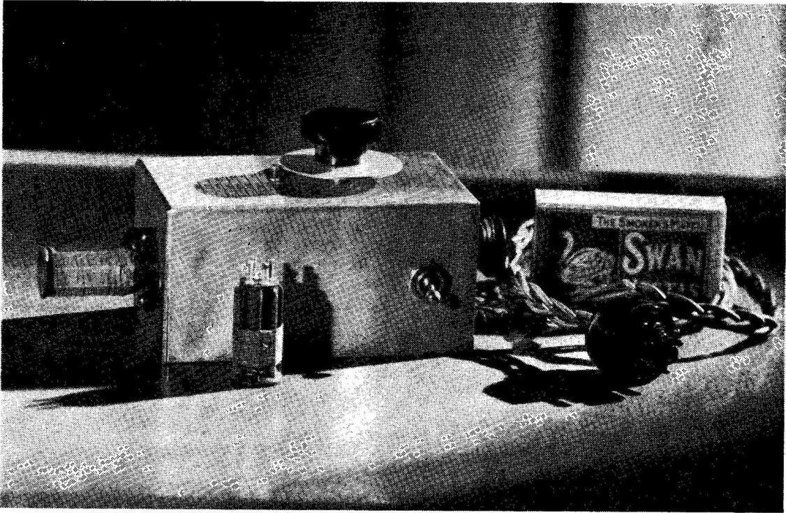
General view of the Beginner's Grid Dip Oscillator, as described in the article. With two coils, the three LF bands are fully covered (160, 80 and 40 metres), with continuous coverage from 1.7 to 7.4 mc. This instrument has a multiplicity of practical uses, as explained in the text, and is an indispensable adjunct to the active amateur station. As designed and illustrated here, it is intended to operate from the Power Pack described in the July issue.
