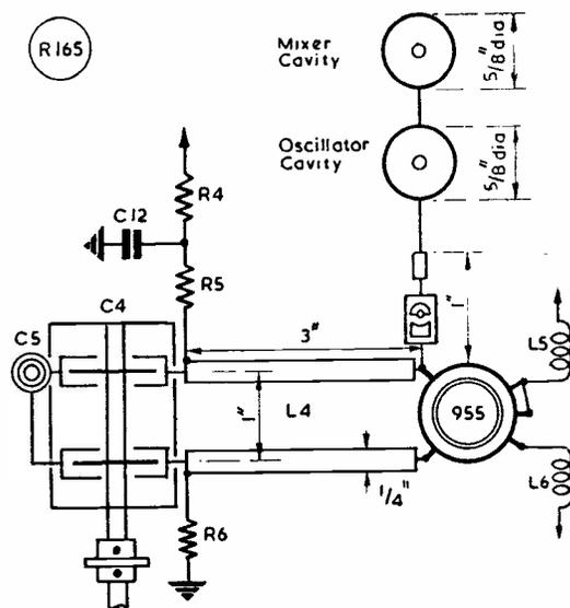
Fig. 5. A 400 mc oscillator is used to give third-harmonic injection in the G3CGQ 25 cm receiver. The layout round the 955, which is an easy and stable oscillator at 400 mc, should be as shown here; L5, L6, are RF chokes (see table of values for winding data) and with a  $5 \times 5 \mu\text{F}$  midget variable at C4 a frequency swing of about 60 mc is obtained on the 25-centimetre band.
