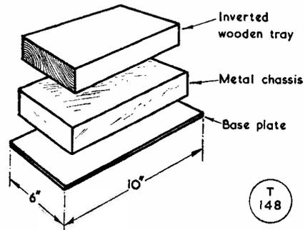
Fig. 2. Mechanical assembly of the portable transmitter/receiver described by G8PG. The metal chassis is fixed to a base plate and the upper part of the chassis is enclosed by a wooden cover. When fitted together, the whole thing can be carried comfortably under one arm.
