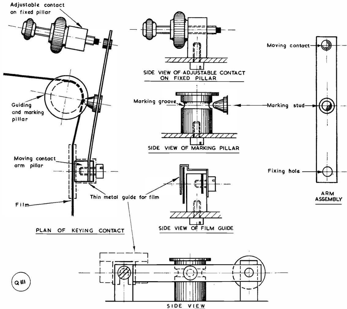
Fig. 2. Arrangement of the keying head, showing how the marking pillar is grooved and the tip of the marking stud rounded to give positive make-and-break at the keying contact; this groove, and the rounding of the marker stud, may be a matter for adjustment, the aim being to obtain sufficient "throw" on the keying arm with no tendency for the marker stud to catch in the tape perforations.
