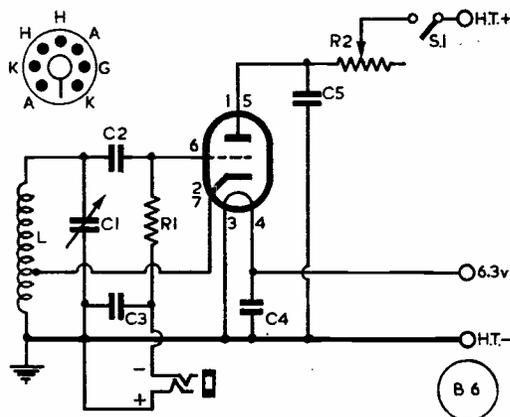
Fig. 1. Circuit of the Grid Dip Oscillator, for which full details for construction, calibration and uses are given in the article. The valve is a 9002 miniature triode, few parts are called for (see table for values) and the circuit is of the simplest — yet it is safe to say that, when it comes to the building of transmitters, without a GDO you can hardly find your way about the bands.
