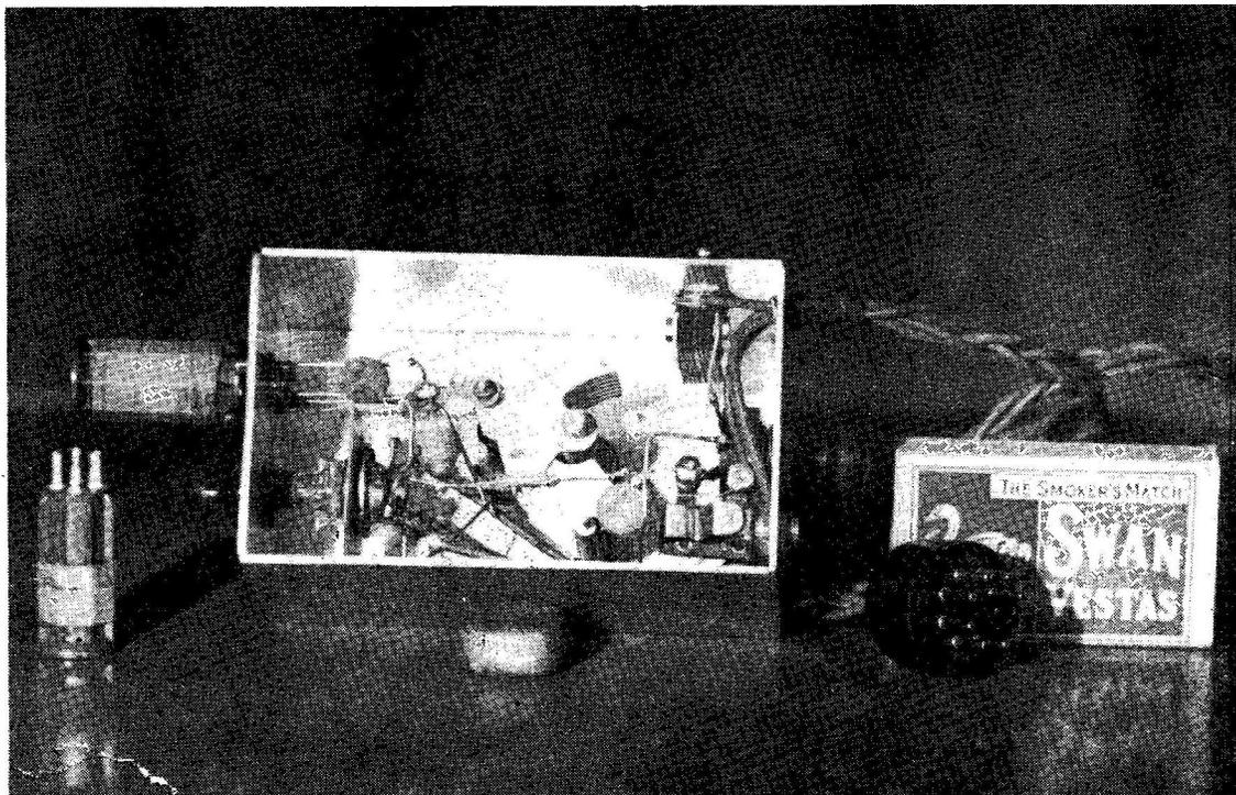
Inside the Grid Dip Oscillator — the valve mounting can be seen lower left, with the tuning condenser (C1 in circuit diagram) at the centre. The octal plug takes HT and LT supplies from one of the sockets seen on the Beginner's Power Pack on p.267 of the July issue.
