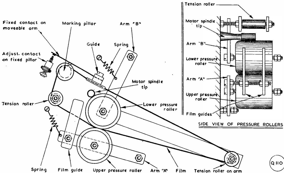
Fig. 1. Detail of the driving mechanism, showing the layout used by G2NS and described in the text. The drive, marked "Motor spindle tip," can be either a (gramophone) spring motor or a small electric motor of the fractional h.p. type. The advantage of using a gramophone motor is that a speed control would probably be already fitted.
