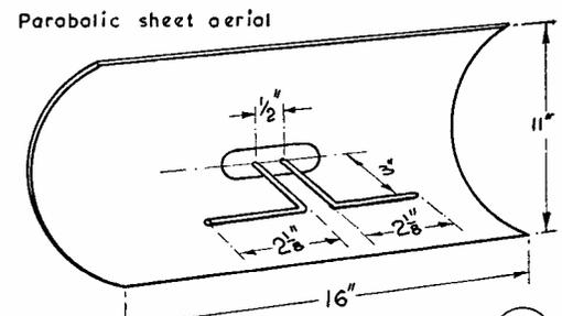
Showing the general layout of the 25-centimetre superhet converter designed by G3CGQ and described in his article. At present, the IF used is 13.5 mc with a Type 194 IF amplifier (Fig. 1). As suggested in Fig. 3, the units form one composite assembly, with the aerial mounted directly on the converter. Fig. 4 gives the dimensions of the cylindrical parabolic sheet reflector, with the detail for the dipole at the focus of the sheet.
