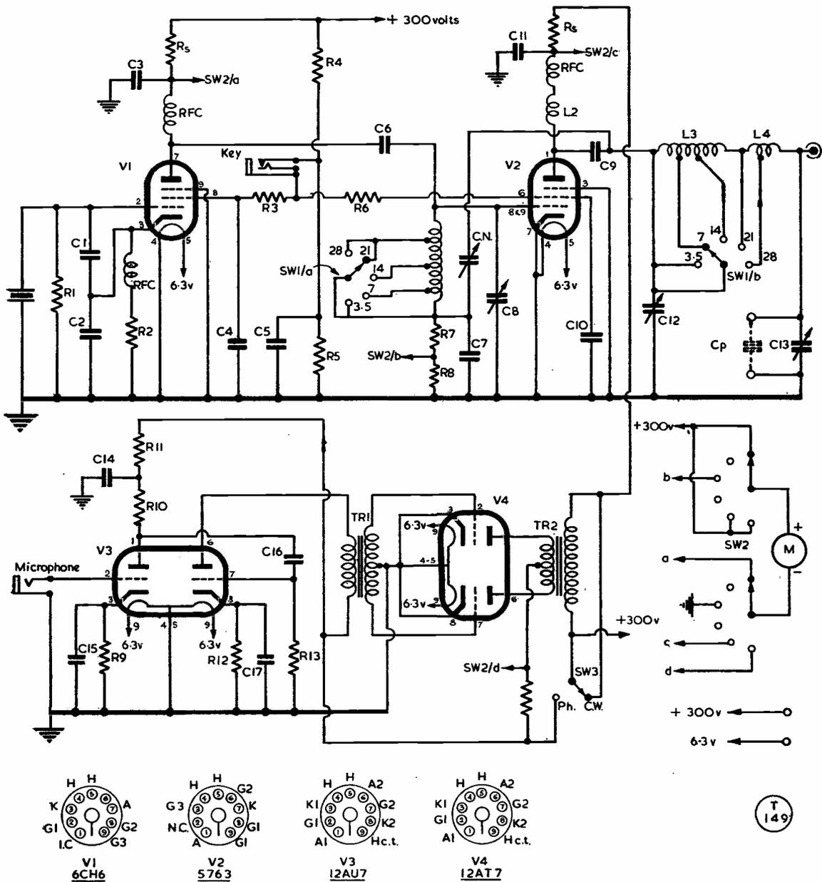
Circuit complete of the portable band-switched CW/Phone transmitter designed and described by G2XX. V1, V2, is the RF section, using a 6CH6 at V1 and a 5763 as PA ; a pi-section tank circuit is used for matching any length of wire on any band. Modulation is by plate-and-screen control, the speech amplifier-modulator section being V3, V4, using miniature twin-triodes. A switched meter, with suitable shunts  $R_s$ , is used for the various current measurements. All values are given in the table.
