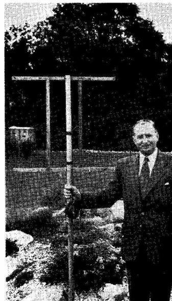
EI2W with the 5/5 for 70 cm he used when making the first EI/G contact on that band, with G5YV on July 14, as reported in our last issue. The elements are carried on the horizontal supports and, being end-on to the camera, do not show up in this view.
