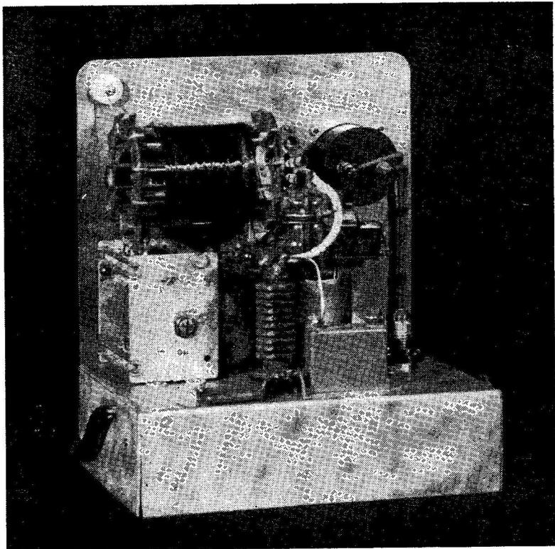
Rear view of the Beginner's Transmitter, showing the general arrangement behind the panel. The tuning inductance L is top left, mounted across C2 (left) and C1. The RF choke, with its sectionalised windings, can be seen mounted vertically beside the 807 oscillator valve, on the near edge of the chassis. The condenser to its immediate right is C6, with the crystal current indicator (a 60 mA flash-lamp bulb) mounted to the right rear.
