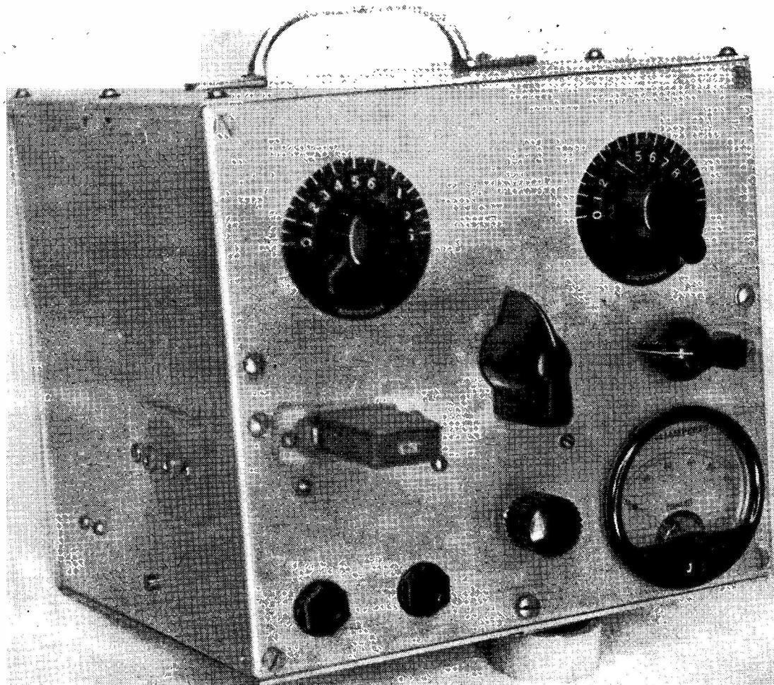
General appearance of the all-band CO-PA "Caravan Transmitter" designed by G2XX. Though approximate dimensions overall of his model are only 7 ins. by 6 ins. by 6 ins., the frequency coverage, band-switched, is 3.5 to 28 mc inclusive, either CW or phone. The Brimar 5763 PA takes up to 15 watts input and the total load on the car battery is about 7 amps. at 12 volts. An external dynamotor power supply is used.
