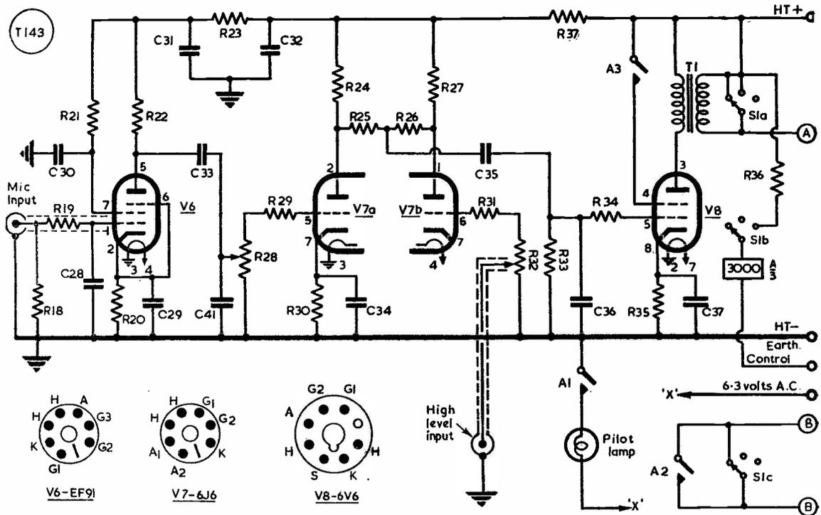
Fig. 4. The modulator circuit for the 160-metre transmitter described in this article. Full control is obtained, with good speech quality, and the circuit is arranged for alternative high-level audio input at V7B, as when "playing back" from a tape recorder or the receiver output. Points A, B-B, connect as shown in the circuit on p.351, September issue.
