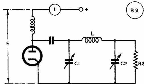
In the formulæ are given the calculations, step by step, for deriving values for a pi-section coupler. This is the circuit arrangement in which all such couplers are used.
