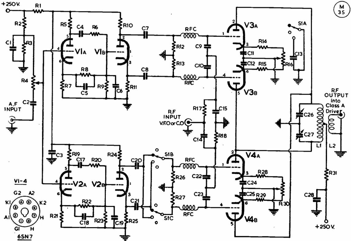
Fig. 2. Circuit complete of the Single-Sideband Exciter described by G3GEN and based upon a standard design. It is of the phasing type, with low-level balanced modulators. The switching provides for A3 (AM phone) carrier when required. Note that the top end of C13 should go to the junction of R14, R16, and that the switching is shown in Posn. 3 of the 4-way switch S1A-S1C.
