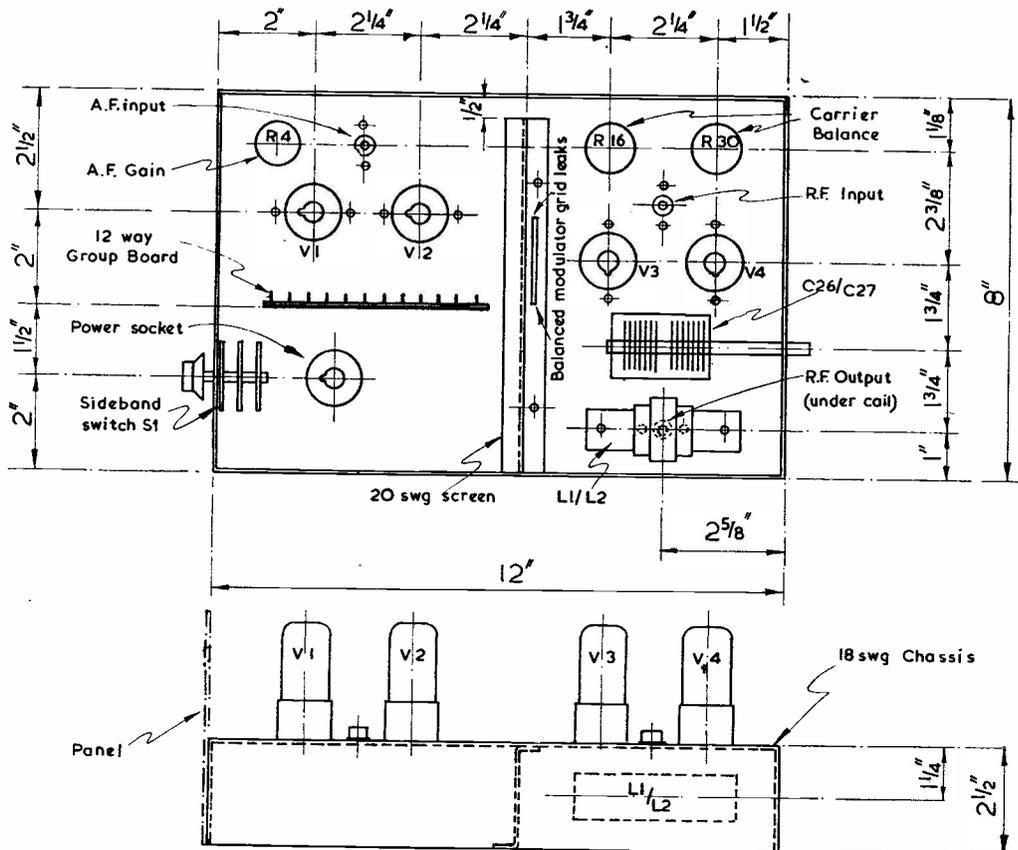
Fig. 3. Chassis layout adopted by G3GEN for the construction of the SSB Exciter described in his article.
