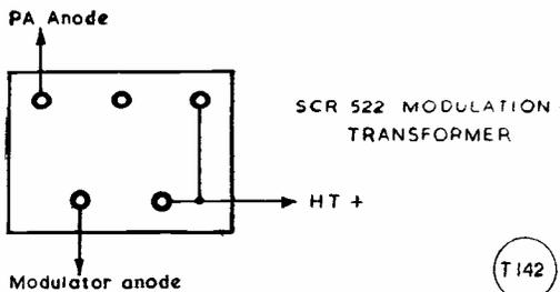
Fig. 3. Connections for the modulation transformer in the G3FRV transmitter with an SCR-522 mod. xformer. When a Woden UMI is used details are: Strap 3/4, 9/10; take HT + to 5/11 strapped; 6V6 anode to 2; QVO4-7 anode to 8.
