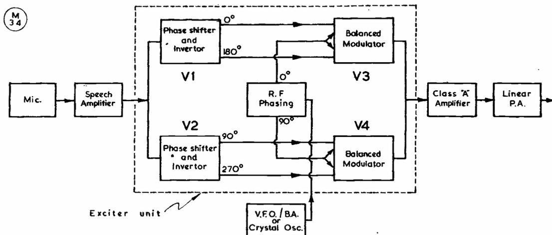
Fig. 1. Block schematic, showing the SSB Exciter in a typical transmitter chain.
