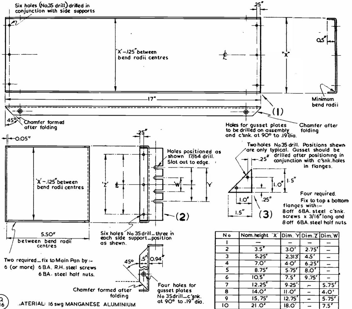
These drawings illustrate the mechanical construction of the chassis units suggested by G3AST. The general arrangement can be followed by a study of the photograph on the opposite page.
