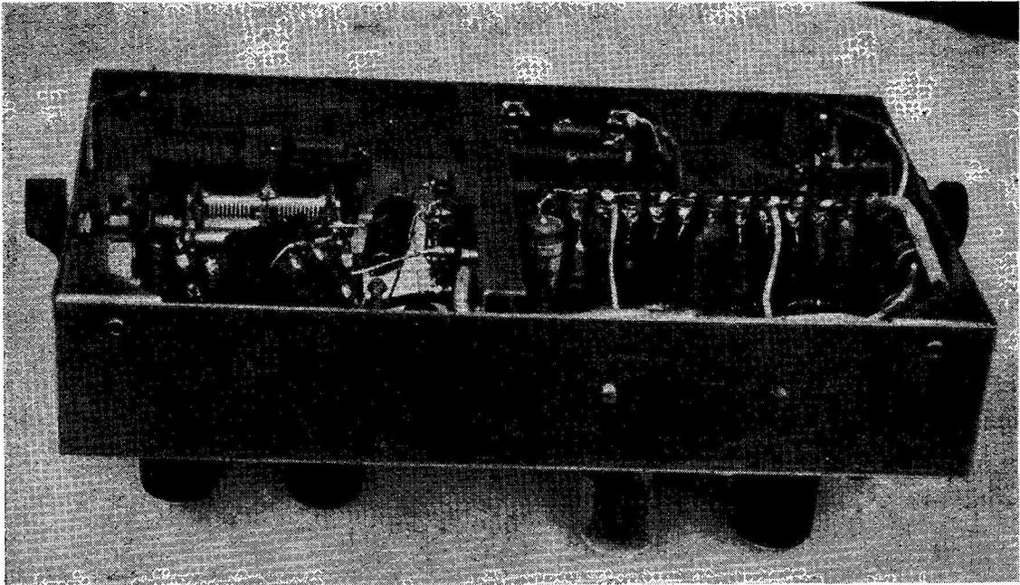
Under-chassis view of the G3GEN SSB modulator. On the left of the central screen are the balanced modulators, V3 and V4 in Fig. 2, with the tuned circuit of L1 at the rear. In the centre of the right-hand section can be seen the group board carrying the twelve audio phase-shift networks.
