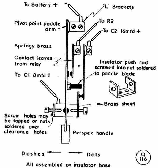
Fig. 2. Electro-mechanical assembly of the auto-key. It should be mounted on a firm, insulating base; if this base is heavy enough and is fitted with rubber feet, the key can be made non-slip in operation.
