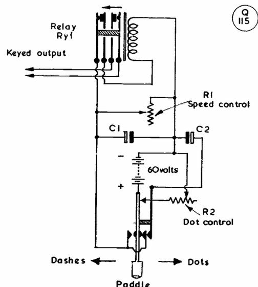
Fig. 1. Circuit of the auto-key described by G3IHH. Using no valves, it is easily put together; the secret of success lies in the adjustment — see text.
