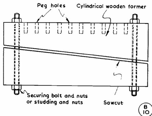
Sectional view of the wooden mandrel which can be made, as described in the text, for the winding of self-supporting transmitter coils. The mandrel collapses by taking out the securing bolts and can then be withdrawn easily after the coil has been formed. Other methods of coil construction are suggested in the text.
