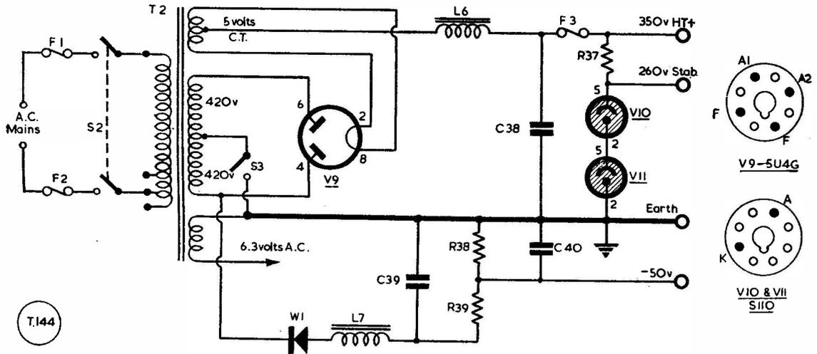
Fig. 5. A suitable power pack, as a separate unit, for the Top Bander designed by G3FRV. All values are given in the table.
