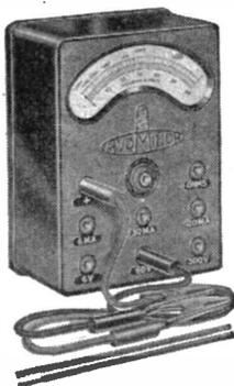
A conveniently compact 2½-inch moving coil precision meter for making D.C. measurements of milliamps, volts and ohms. The total resistance of the meter is 100,000 ohms, and full scale deflection of 300 v. or 600 v. is obtained for a current consumption of 3mA. or 6mA. respectively
