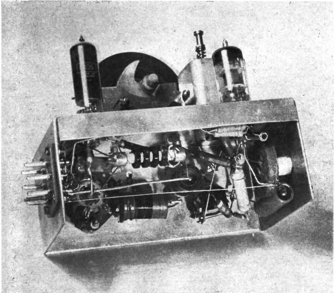
Underside view of the Beginner's VFO. On the left is the plug for coupling in power and taking input; this plug registers with the crystal socket on the chassis drop of the Beginner's Transmitter described in our September issue. At bottom left is S1, and next to it is L3, masking C13. Above is RFC2 and just below and to the right L2, with jack J beneath; RFC3 goes across the jack and was fitted after this photograph was taken.
