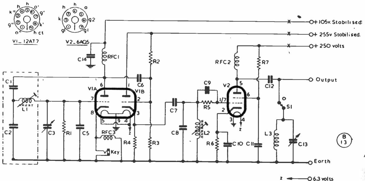
Fig. 1. Circuit of the Beginner's VFO, in which V1a-V1b is the oscillator section with cathode follower output, into V2, the buffer-doubler. The oscillator circuit is the Tesla and the method of keying shown—while allowing for break-in working—does not affect the stability of the oscillator nor the quality of the note. V1a-V1b is a 12AT7 twin-triode and V2 a 6AQ5; both are miniature valves. Ample drive output is given on both 160 and 80 metres, with full band coverage.
