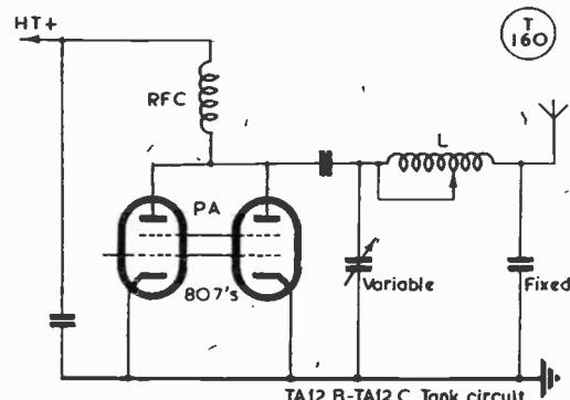
Tank circuit arrangement of the TA-12, which is the same for both "marks," B and C. The PA consists of a pair of 807's in parallel. A separate tank circuit is provided for each of the wave-bands covered. These are 300-600 kc in both, and 3000-7000 kc in the B, but 3000-12000 kc in the TA-12C.
