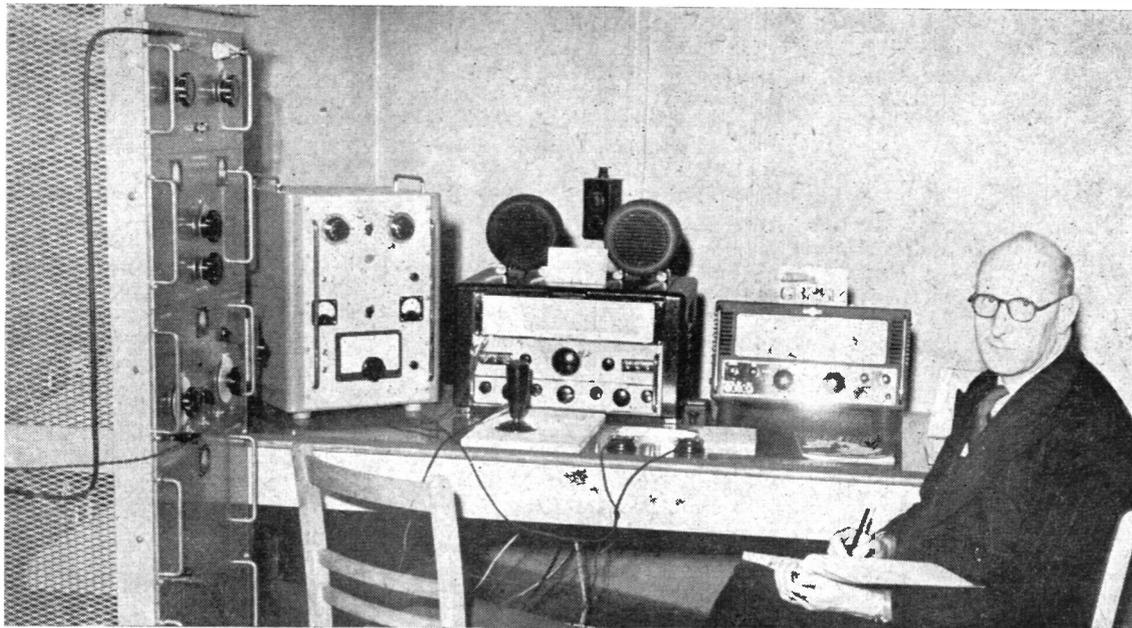
GB2SM at the Science Museum, South Kensington, showing equipment layout. On the left is the rack-and-panel Labgear 150-watt transmitter, with an LG.300 on the operating table. Receivers are a G.E.C. BRT-400E (centre) and an Eddystone 680X. At right is Mr. G. R. M. Garratt, under whose direction GB2SM operates and who is himself G5CS.
