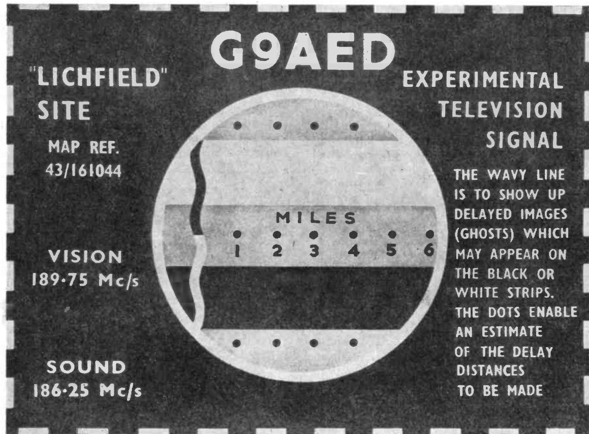
The G9AED Test Card as now being radiated from Lichfield, Staffs., by the Belling-Lee Band III transmitter. All relevant details are given in this photograph. Transmitting periods are: Monday-Friday, 10.0 a.m. to 1.0 p.m., 3.0-6.0 p.m., and 7.30-8.30 p.m.; Saturdays, 10.0 a.m. to 1.0 p.m. There is no other week-end transmission. The G9AED transmitter is rated at 1 kW ERF, peak white.
