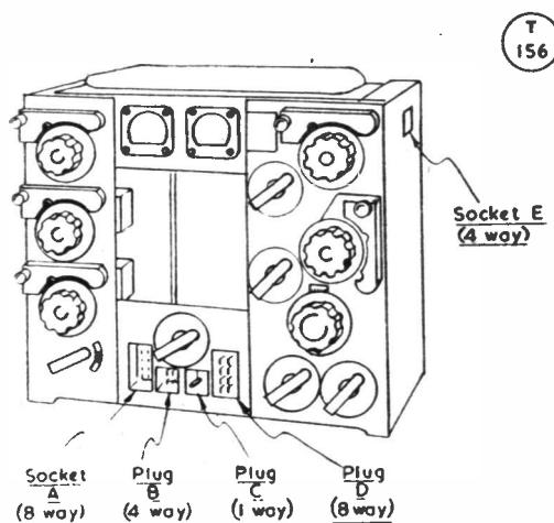
Fig. 3. Outline appearance of the well-known T.1154, to locate the connector points, the key to which is given in Fig. 4.
