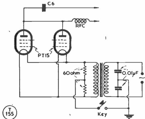
Fig. 2. LT supply and keying circuit for the T.1154 PA. Originally proposed by G2ASY in our December 1953 issue, this gives clean, sharp keying, with a good note, and is a great improvement over the original.
