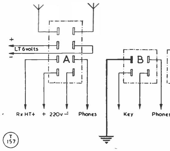
Fig. 4. Detail of the connector system on the T.1154 transmitter—see Fig. 3 for location diagram. By making the connections as emphasised in this sketch, power can be applied direct to the transmitter without involving the receiver inter-connection or control circuitry, which can be ignored.
