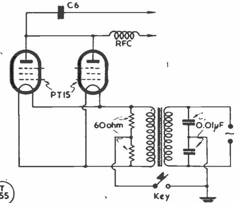
Fig. 2. LT supply and keying circuit for the T.1154 PA. Originally proposed by G2ASY in our December 1953 issue, this gives clean, sharp keying, with a good note, and is a great improvement over the original.
