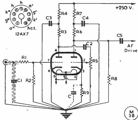
Circuit of the high-gain audio amplifier discussed in the text. It consists of a single Brimar 12AX7 twin-triode and, taking only 2-3 mA at 250v., gives more voltage gain than the conventional 6SJ7-6J5 speech amplifier arrangement.
