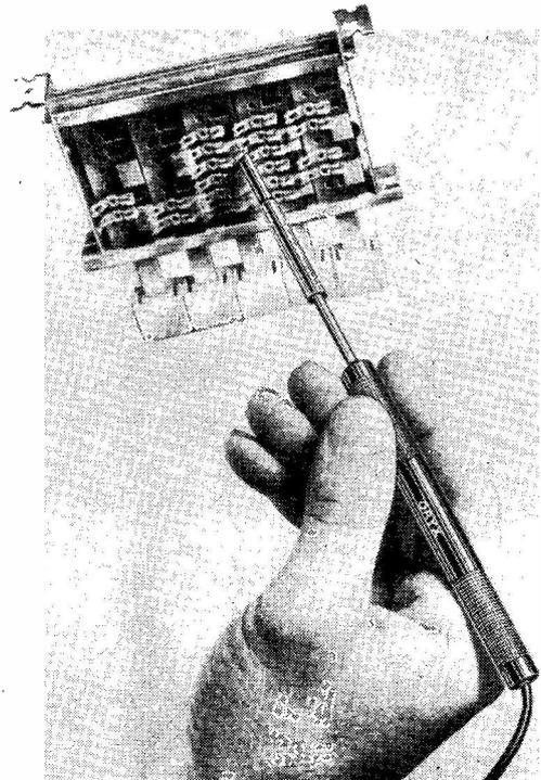
The new Oryx Model 18 low voltage (6-volt) soldering iron has a detachable 3/16-in. bit, specially shaped for small work. The power consumption is less than 20 watts, but the heat capacity is that of an iron of ordinary size. The weight of the Oryx Model 18 is only one ounce, and the construction is simple and robust.
