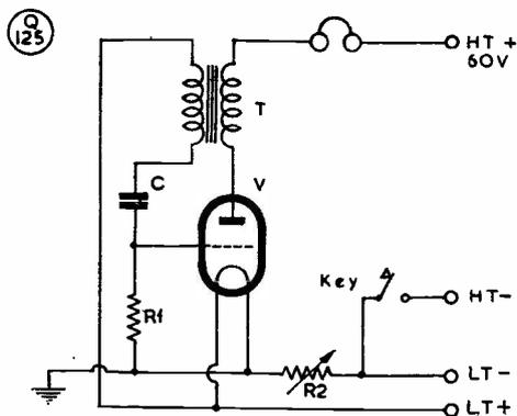
Fig. 7. A simple audio oscillator for Morse sending practice. The key is in the —HT lead and the pitch of the note can be adjusted by variation of the R1 and C values. This oscillator will go off on HT as low as 9v. from a bias battery. Any difficulty in getting it to work is usually because the connections to the transformer are in the wrong sense. If audio oscillation cannot be obtained when the circuit is first set up, the leads on one side of T should be reversed.
