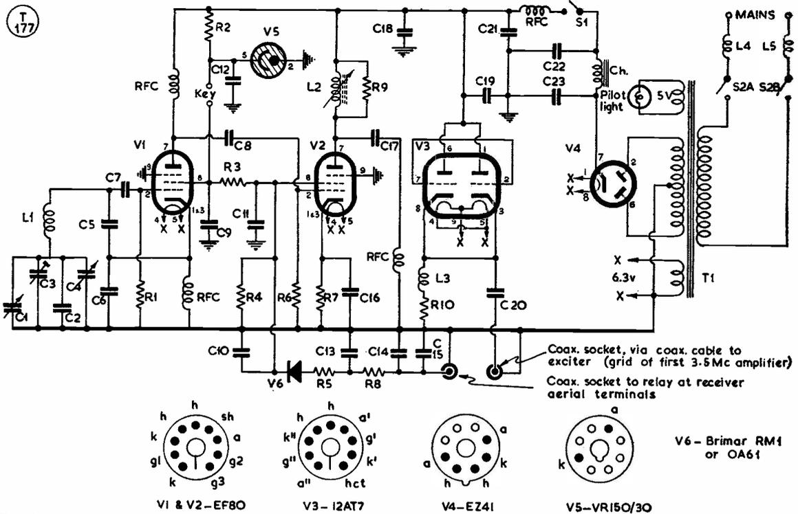
Circuit complete of the self-contained VFO described by G3CNM, the construction of which is illustrated in the accompanying photographs. That part of the circuit identified by V6, R5, R8, C13, C14, C15 is to control a relay to follow the keying; this could be arranged to perform all change-over functions, while permitting BK operation. In the author's case, the relay mutes the receiver. All values are given in the table.
