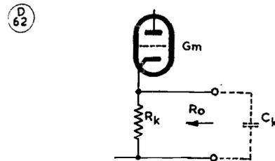
Fig. 2. The pass-band of the cathode follower is determined by the cathode load Rk — see text for discussion.
