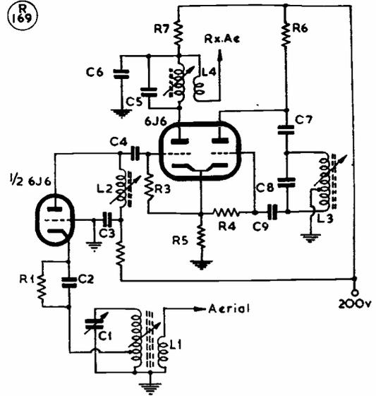
Fig. 1. Circuit for a 10-metre converter for use with any communications receiver which can be tuned across 8 mc. A grounded-grid triode (for convenience, one section of a 6J6) feeds into another 6J6 as mixer-oscillator, the output being taken at L4. If the converter is operated externally to the main receiver, it would be better to use coax feed from the link winding on L4. Values and coil data are given in the tables.
