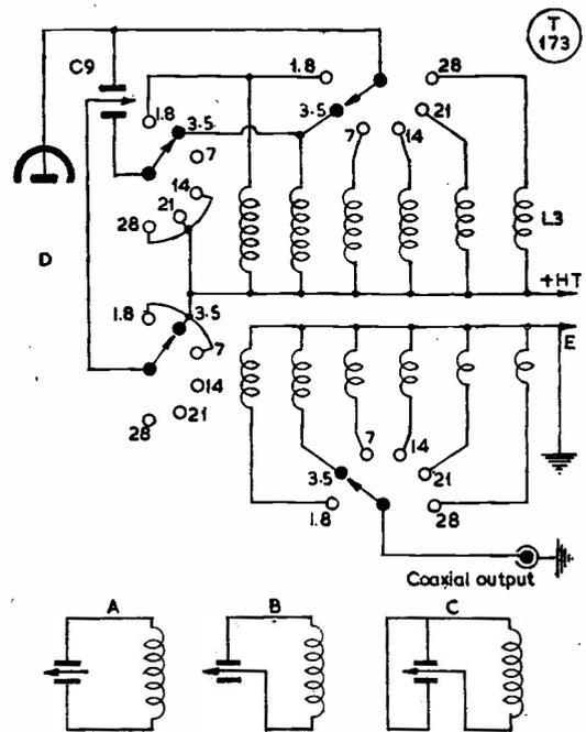
Fig. 5. Amplifier tank switching system, showing (below) how the double section condenser is used on various bands; in A, it is as a split stator on 14, 21, and 28 mc, 37.5  $\mu\mu\text{F}$ ; on 7 mc, B, one stator/rotor section only is used, giving 75  $\mu\mu\text{F}$  maximum capacity; on 3.5 and 1.8 mc, C, the stators are in parallel, equal to 150  $\mu\mu\text{F}$ . Three wafers are used for L2/C8 (not shown), and 4 wafers for C9/L3, with L4.
