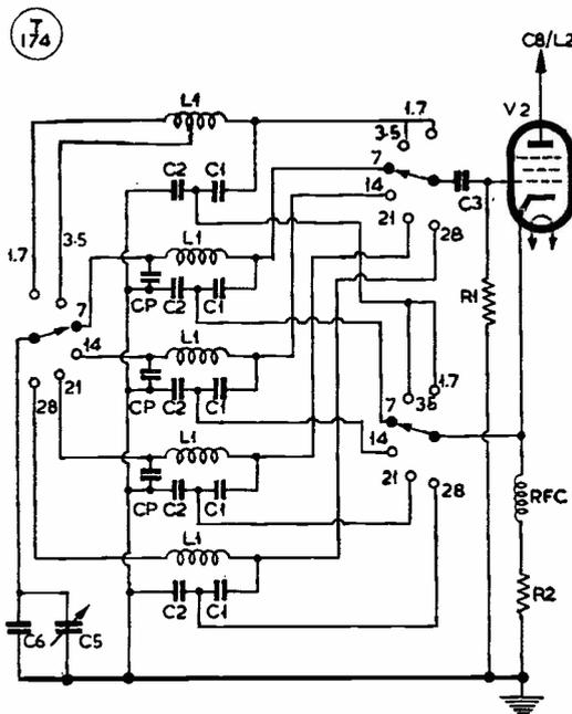
Fig. 6. Oscillator switching layout, with coil values in the table—and see text for discussion.
