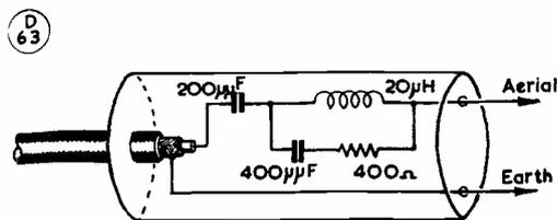
Fig. 3. Arrangement of the "dummy aerial" for the simplified signal generator, as explained in the article.
