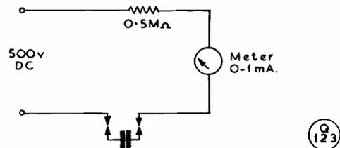
Fig. 2. A simple method of measuring, roughly, the DC resistance of a condenser. The high voltage can usually be derived from a transmitter power unit, taking due care when handling the leads. After the initial switch-on surge, the current flowing should be very small indeed if the condenser is a good one. A steady current of a tenth of one milliamp or more indicates too low a DC resistance for the condenser to be of practical use.
