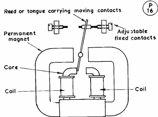
Fig. 2. Basic details of a polarised relay, which can be used in circuits where rapid operation is required.
