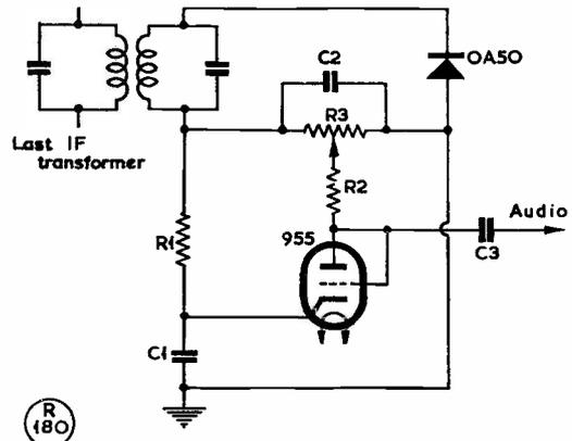
Fig. 3. Modified Noise Limiter Circuit.
