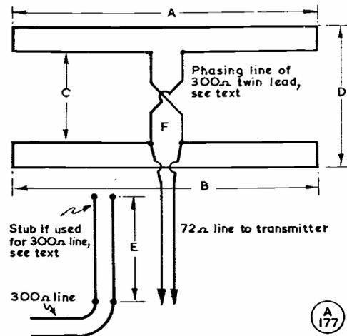
Fig. 3. Electrical layout of the "ZL Special." Dimensions for 10 and 20 metres are given in the table, and those for a 15-metre version can be calculated from the formula in the text. This simple beam, being fully driven, gives a very useful gain in comparison with any parasitic system of similar size.
