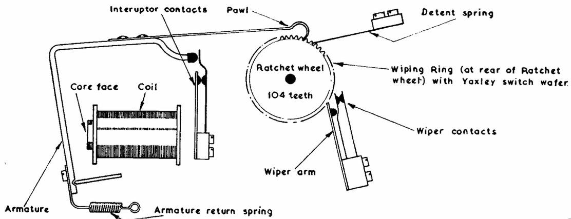
Fig. 3. Electro-mechanical layout of the G.P.O. Uniselecter relay, an interesting and ingenious mechanism which has many useful applications. Each pulse of current in the coil moves the ratchet wheel one tooth, the pulses being produced by the interrupter contacts. The circuit being switched is controlled by the wiper contacts.
