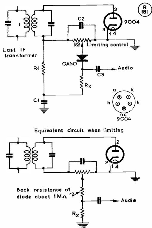
Fig. 4. Noise limiter circuit found most effective, for which values are given in the table, with the "equivalent circuit" when limiting shown below. Very good results are obtained under stringent operating conditions.
