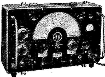
**The "AVO" Wide Band A.M./F.M. Signal Generator (Type T.F.M.)**
