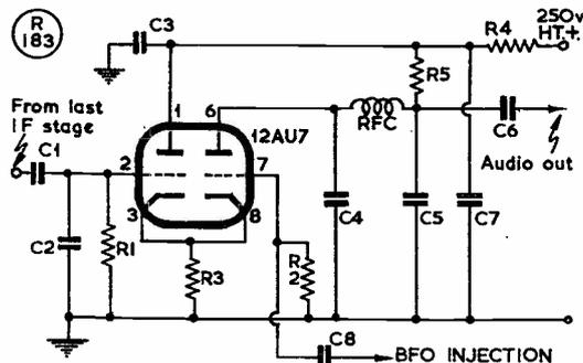
Fig. 1. The product detector circuit incorporated in the Collins 75A4 receiver for SSB reception, as discussed in the text.
