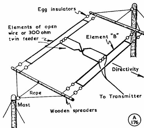
Fig. 2. Layout of the "ZL Special," full design details of which are given in the text—and see Fig. 3. Directivity can be changed simply by swinging the system right over, so that element B lies on the opposite side. At some stations, fully rotatable "ZL Specials" have been installed, to give 360° coverage.
