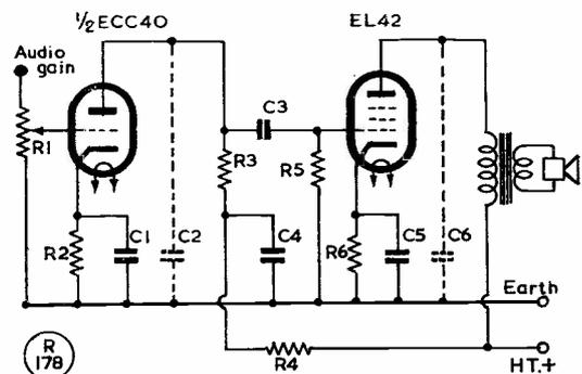
Fig. 1. First experimental circuit, values as in the table. C2, C6, were added to reduce the upper frequency response of the amplifier.
