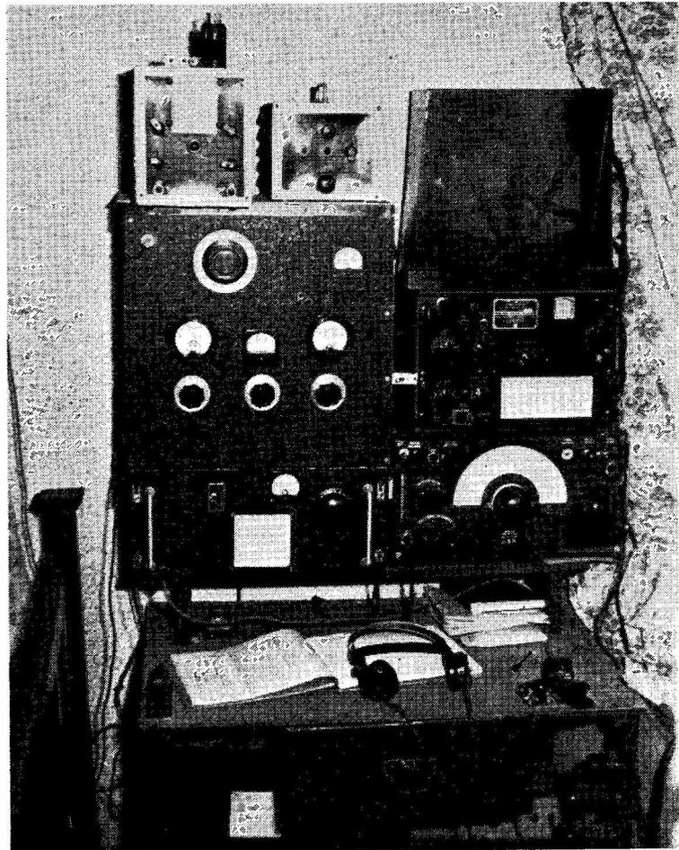
Station of G3JMH, Liverpool, 7, is accommodated in restricted space, both inside and out. Activity is mainly on 80 and 160 metres, into a 66-ft. "multi-bent" aerial (about seven times) finishing up with "one turn round the room"! Nevertheless, even on this unpromising aerial OK has been worked on Top Band, and nearly 350 contacts made on the two LF bands. Construction is in hand for 7 and 14 mc, and G3JMH also operates GW/P.
