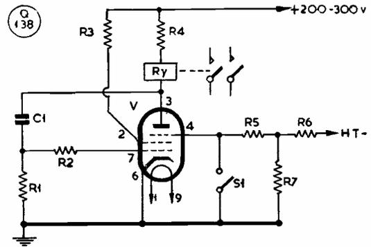
Circuitry for the valve delay system. The delay is controlled by the constants C1, R1 and is variable over wide limits. With the values given, a 40-second pause can be obtained before the relay is actuated.
