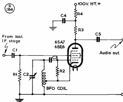
Fig. 2. In the National NC-300 receiver, the product detector circuit for SSB reception is as shown here; values are given in the table.
