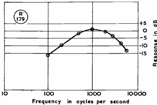
Fig. 2. Response curve of the modified audio amplifier — see text for discussion.
