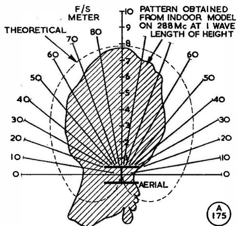
Fig. 1. Horizontal radiation pattern of the "ZL Special" as deduced from a scaled-down model. It compares well with the theoretical polar diagram.
