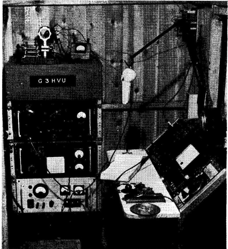
Top Band transmitter, this being switched for use as the driver stages for the 5-band transmitter.
