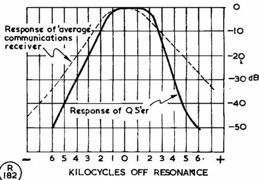
Fig. 5. Response curve (solid) when using a Q5'er, showing the selectivity gain, particularly marked on CW signals.
