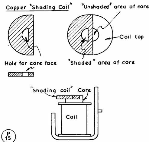
Fig. 1. Construction of an AC relay, which has part of the core "shaded" to maintain the field, as explained in the text.
