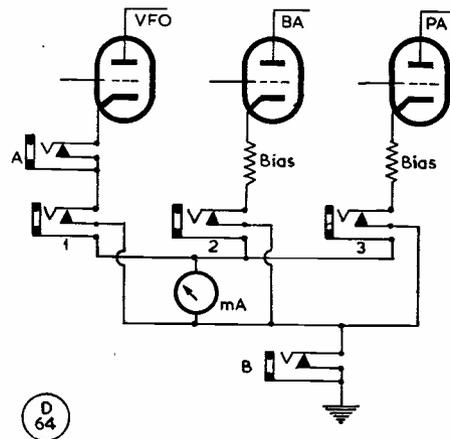
The circuit discussed in the text. With one meter, currents at three points can be measured, either together or separately, and the same jack points can be used for keying. All that is required is one or two shorting plugs.
