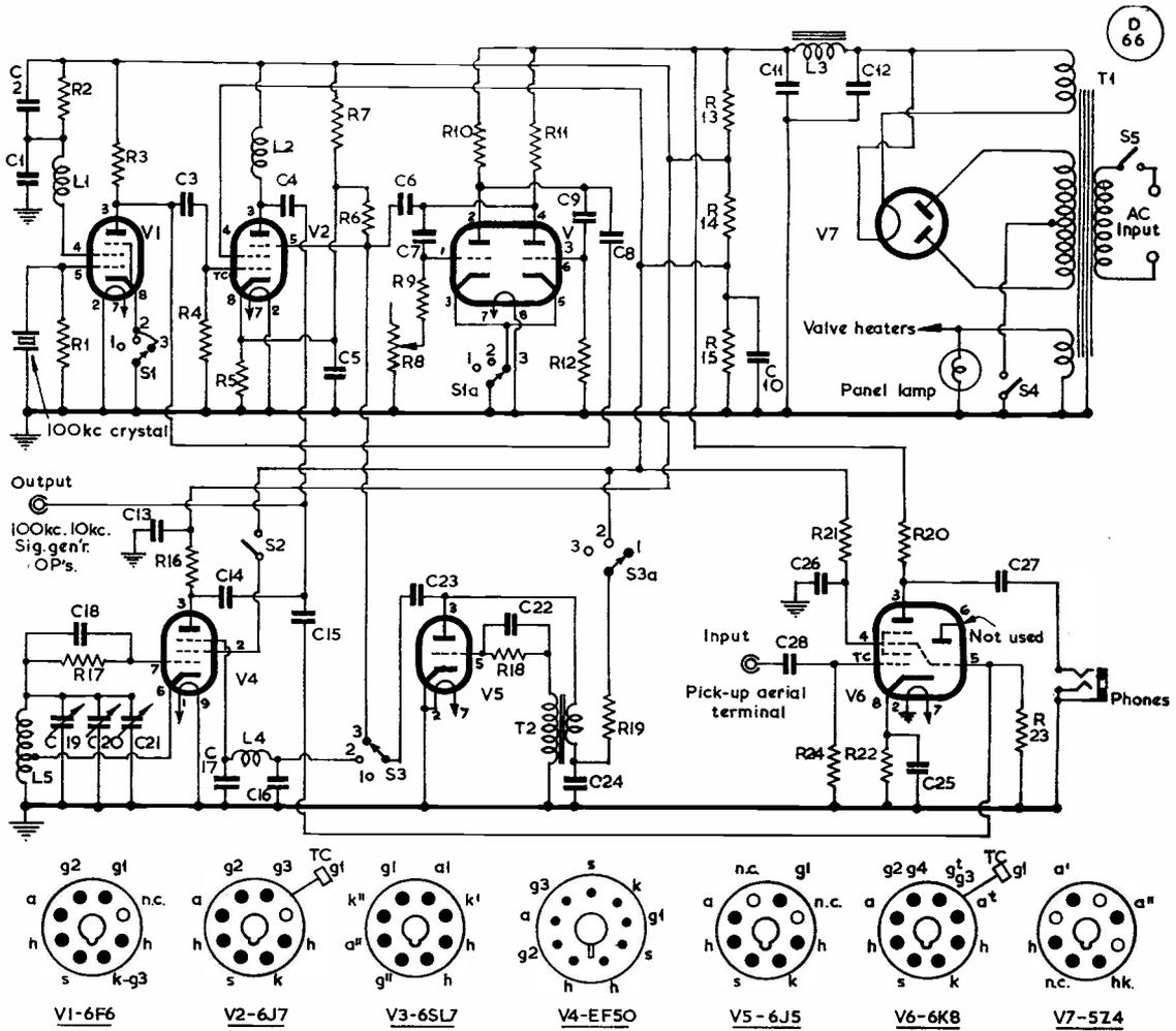
Circuit of the combination signal generator, heterodyne frequency meter and CW/phone monitor described in the text. It is self-contained for power and all values are given in the table.
