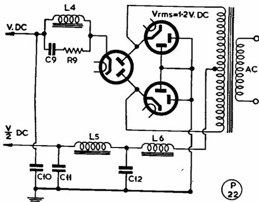
Fig. 3. With this arrangement three full-wave rectifier valves will give two voltage outputs at different current loadings from the one transformer.
