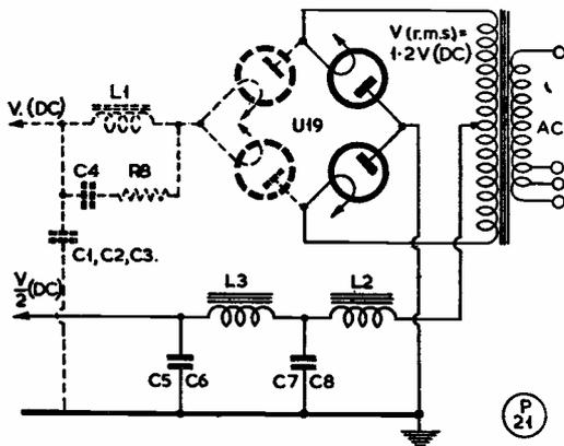
Fig. 2. This drawing divides the two circuits electrically, to show how each operates — see text.
