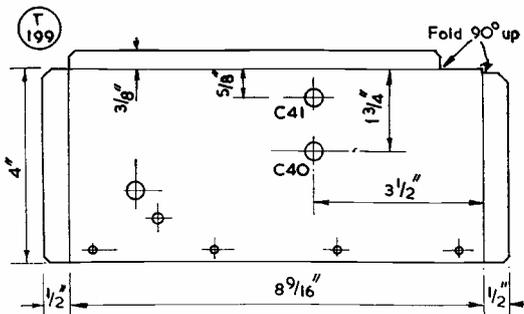
Fig. 5. The apron for the PA chassis, viewed from the rear with the transmitter inverted. The correct positioning of this, and the screens shown in Figs. 3 and 4, will be evident by examination of the actual transmitter chassis.
