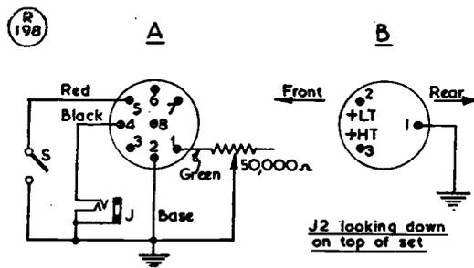
Fig. 3. (A) Circuit diagram of the gain and BFO control wiring, as described in the text. (B) Re-arrangement of connections for the entry J2 in the circuit of Fig. 1.
