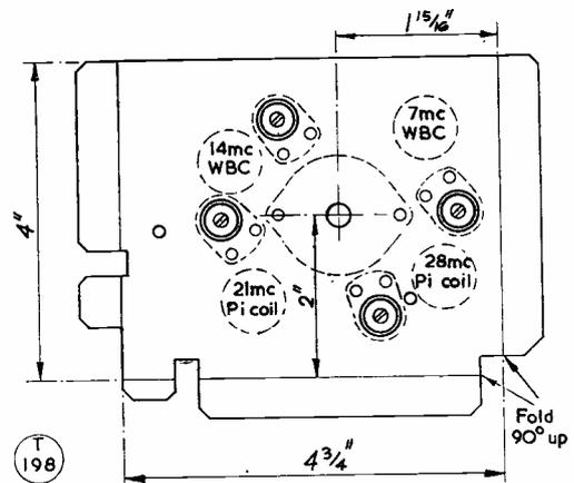
Fig. 4. Under chassis screen seen from the VFO with the transmitter inverted. The components are mounted on the reverse side.
