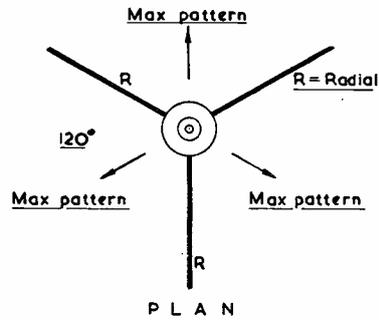
General arrangement of the ground plane transmitting aerial system described by HB9OP. Dimensions are given in metres and millimetres (one metre = 39.4 inches) and from the data, either a multi-band or a single-band ground plane can be designed. As explained in the text, it is essential to make the radial angle with the horizontal 45°. With a 120° plan angle between them, some control over directivity is possible, as shown by the "max. pattern" indication — and see text.
