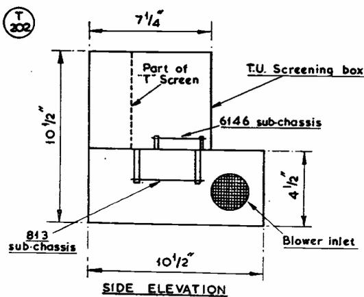
Fig. 2. Simplified drawings showing general arrangement of the chassis and screening compartments, with dimensions, and the placing of main parts. The upper screening box is from a TU unit and the chassis is made from heavy-gauge aluminium. The V1 compartment also serves as a screening box for meter M1.
