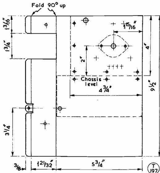
Fig. 3. The large dividing screen, as viewed from the VFO side with the transmitter inverted.
