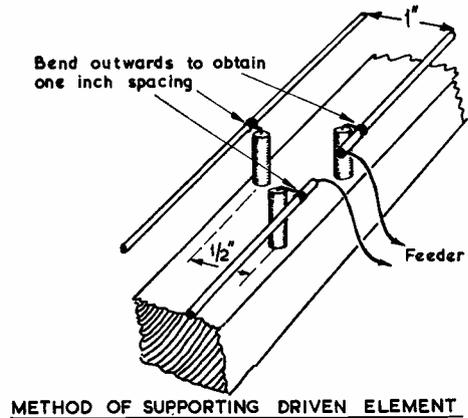
Fig. 5. Detail of the mounting of the elements for the four-metre beam, using the simplified stand-off insulators suggested by G3GVA.
