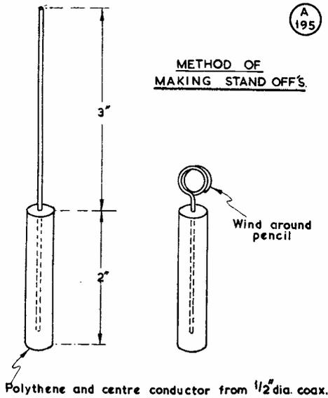
Fig. 3. Construction of the home-made stand-off insulator, from odd pieces of coax. The centre conductor makes the grip for the element.
