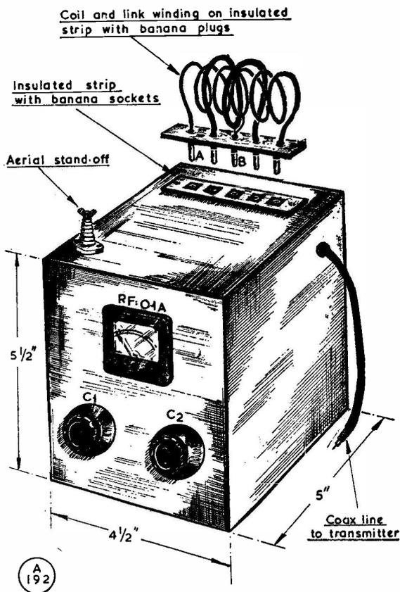
Fig. 2. General impression of the tuner unit as constructed for experimental purposes. The box is of aluminium, and plug-in coils are used to cover the three working bands.
