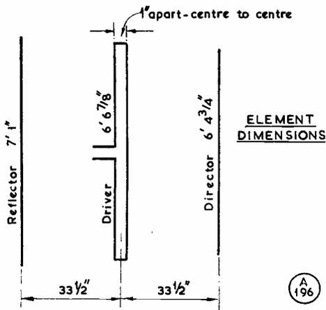
Fig. 4. Dimensions and spacing layout for the elements of the four-metre beam. Lengths are for 70.3 mc and spacing is 0.2 wavelength.
