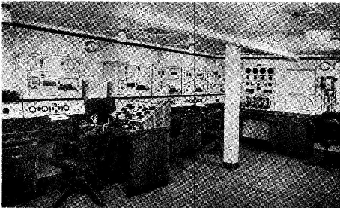
Radio receiving and control room of the R.M.S. "Queen Elizabeth." The transmitter installation is entirely separate and the receiving office is fully screened against interference from the ship's extensive electrical equipment.
