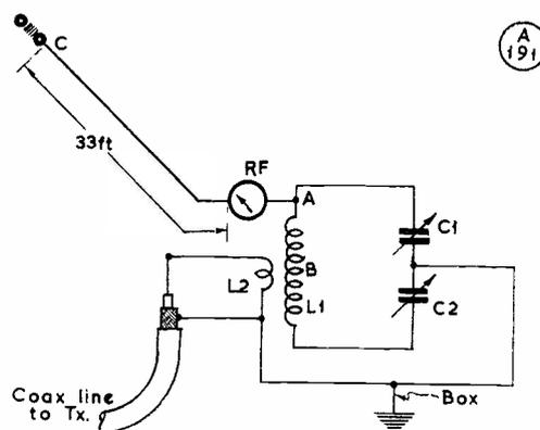
Fig. 1. Circuit of the tuner unit described in the article, the general arrangement being to accommodate a 33 ft. wire which is used half-wave on 14 mc, three-quarter-wave on 21 mc and full-wave on 28 mc. It can be tapped on at either point A or B, with the network L1, C1, C2 resonated at the mid-frequency of the band area, CW or phone, to be covered. For a 100-watt transmitter, the RF meter will need to read 0-1 amp. for safe working on 15 metres.
