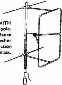
SINGLE SLOT PORTABLE ANTENNA WITH 2 REFLECTORS. Gain 8 DB over a Dipole. Horizontal Beam width 70°. Feed Impedance 75 ohms. Designed for quick assembly, together with the necessary strength for fixed station use. Supplied complete with 5' x 1½" mast. PRICE: £3/10/-.
