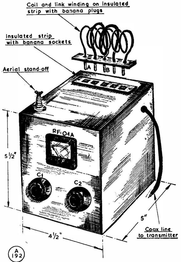
Fig. 2. General impression of the tuner unit as constructed for experimental purposes. The box is of aluminium, and plug-in coils are used to cover the three working bands.
