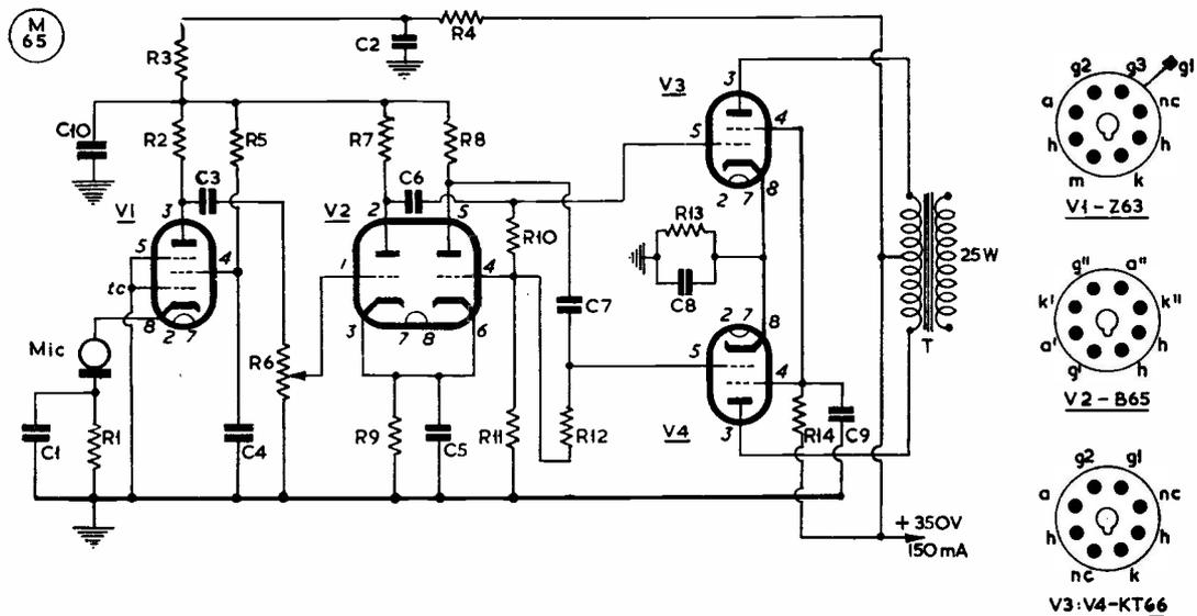
Circuit of the 25-watt modulator. It is intended for a high-output microphone, such as a G.P.O. carbon type, and it will be noted that excitation is by cathode current of the first stage. As it stands, the speech amplifier can be used only with a carbon microphone. For a crystal type, an additional voltage-amplifying stage would be necessary, with a re-arrangement of the V1 circuit. If the power pack will give a good 350v./150 mA, 25 watts of audio should easily be obtained.
