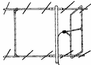
6 OVER 6 SLOT BEAM. Gain 13 DB over a Dipole. Horizontal Beam width 20°. Feed Impedance 75 ohms. Supplied complete with 7' x 1½" mast. PRICE: £7.
