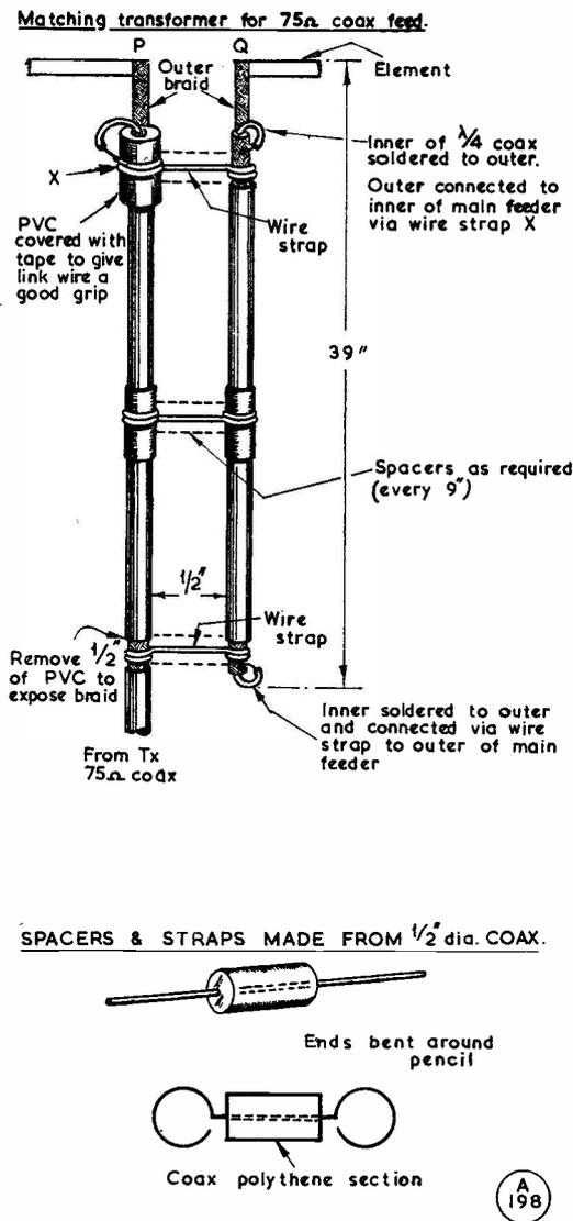
Fig. 6. Matching device for 75-ohm coax feed, balance-to-unbalance converter. The alternative is direct feed at points P-Q using 300-ohm ribbon (or tubular line), with the folded dipole dimensions given in Fig. 2.
