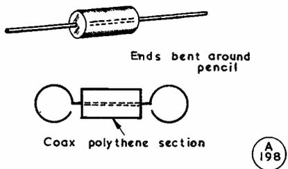
Fig. 6. Matching device for 75-ohm coax feed, balance-to-unbalance converter. The alternative is direct feed at points P-Q using 300-ohm ribbon (or tubular line), with the folded dipole dimensions given in Fig. 2.
