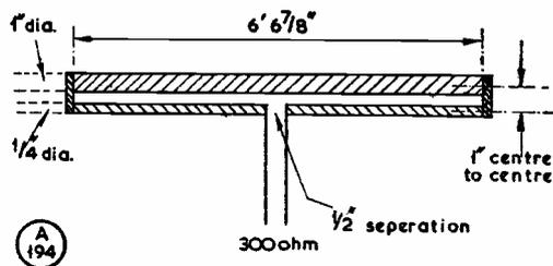
Fig. 2. Dimensions for the folded dipole element. Dissimilar diameters are only necessary if a 4-to-1 ratio is required to match in 300-ohm line (see text).
