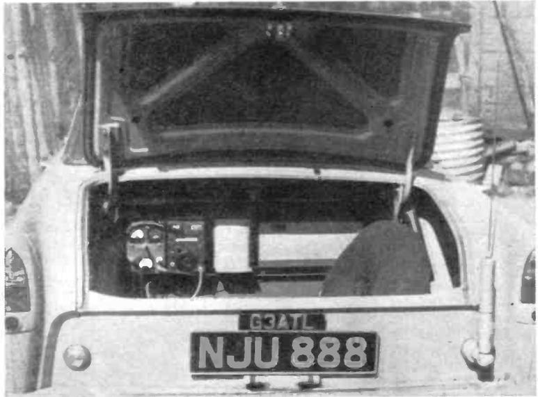
Equipment assembly for mobile working, fitted in the boot of G3ATL's car. Many hundreds of /M contacts have been made on Top Band and Eighty.
