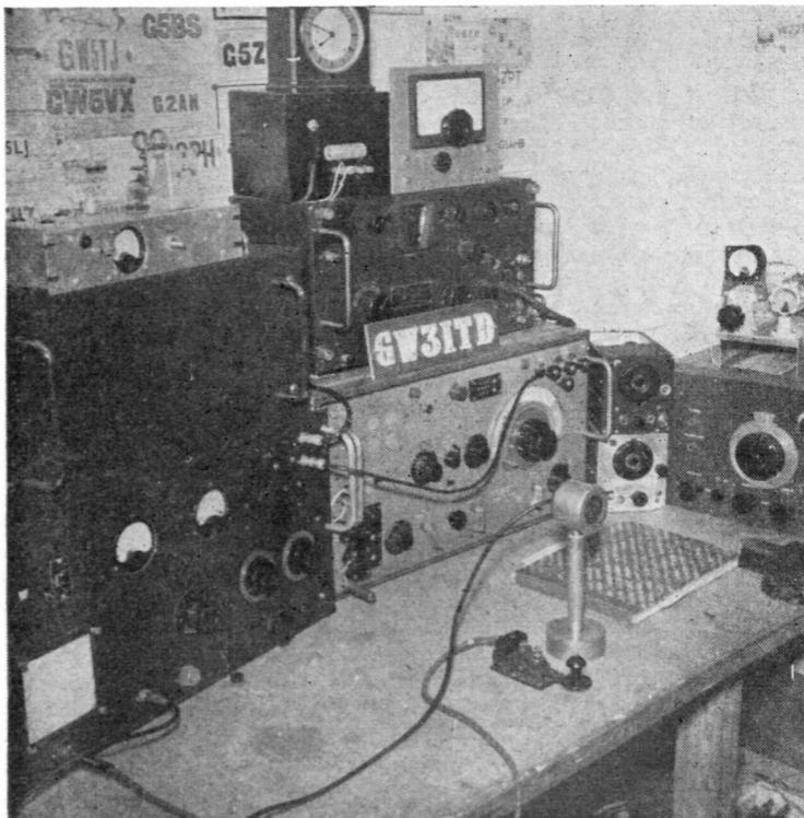
Neat layout at GW3ITD, Llanbyther, Carmarthen, who was first licensed in 1952. The transmitter assembly at left consists of an EF91 Clapp VFO into EF91's as buffers, exciting four 5763's as wide-band amplifiers, into a pair of 807's in parallel; the modulator arrangement is EF91-6J5-6N7 into push-pull 5B/254M's, and is contained with the RF section of the transmitter. Receivers are R.107, BC-312 and an R.1224A for portable work. His aerial is 132 ft., pi-coupled.
