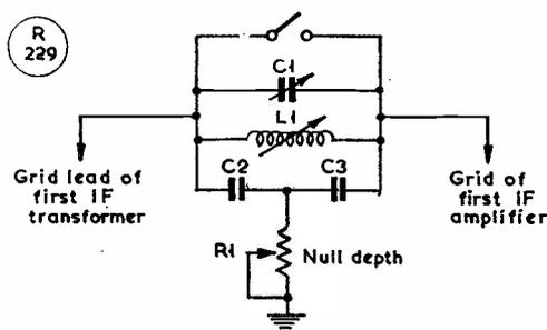
Fig. 3. As suggested in the article, a T-notch rejection filter can be used instead of the "Q-Multiplier." In this circuit, values are: C1, 100  $\mu\text{F}$ ; C2, C3, .003  $\mu\text{F}$ ; R1, 15,000 ohms; L1, 4-5 mH.
