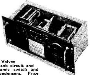
These well known units have Micro Meter dials with 2,500 divisions over 180 degrees rotation giving plenty of mechanical bandspread. Velvet vernier drive, high Q tank circuit and heavy duty 6-way ceramic switch and variable transmitting condensers. Price 14/- each P.P. 4/-.
