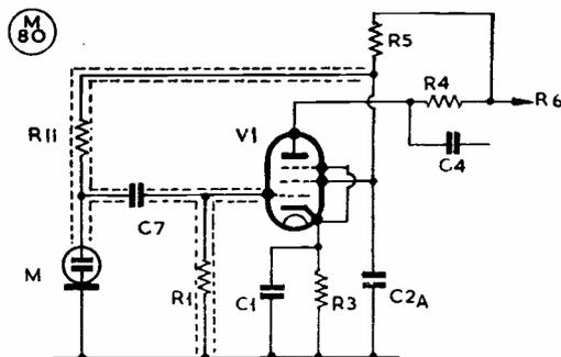
Fig. 2. When using a condenser microphone, the input circuit can be arranged as shown here. C7 is .01  $\mu$ F, 350v. working, and R11 anything from 20 to 40 megohms. Shielded and earthed leads should be used as indicated.
