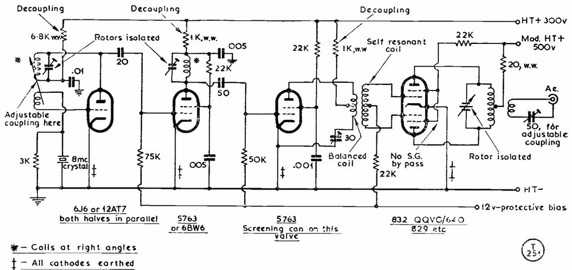
Fig. 11. The points to watch in the layout and construction of a two-metre transmitter, if stable operation is to be obtained under full modulation. The circuit values as shown are correct for the 144-146 mc band, and coils are as normally used; some data are given in the text. It will be noted that for de-coupling, low-value wire-wound resistors are used; the advantage of this is explained in the article. The circuit as shown here represents good modern practice in VHF design and technique.
