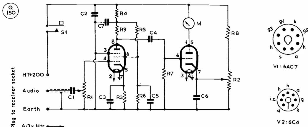
Circuit of the Modulation Meter, designed as an auxiliary unit for any usual type of communications receiver, from which it could take its power. The effectiveness of the arrangement depends upon the accuracy of the initial setting-up procedure, since it is a reference system, as explained in the text. Even if not accurately calibrated, however, it will always compare, reliably, the depth of modulation between different stations on the same band.
