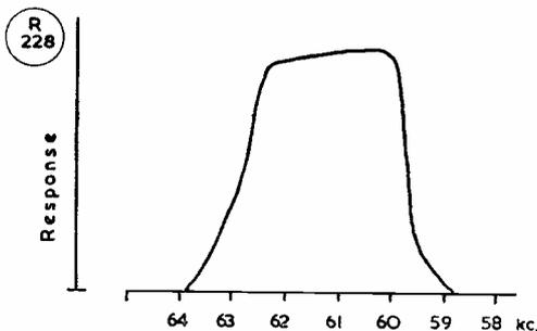
Fig. 2. Response curve obtained on the 60 kc section in the IF/AF Amplifier described by G3KGN.
