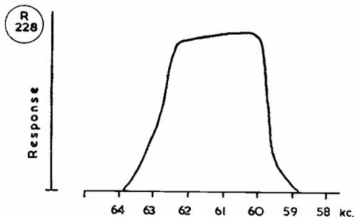
Fig. 2. Response curve obtained on the 60 kc section in the IF/AF Amplifier described by G3RGN.
