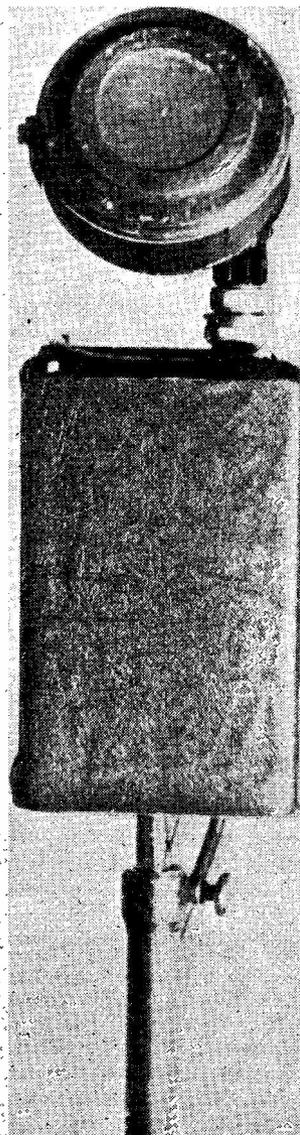
Microphone and head amplifier on its stand, complete, as described in the article. The increased audio gain enables the microphone to be "talked at" in comfort from several feet away, while allowing a connecting lead of any convenient length into the speech amplifier proper.
