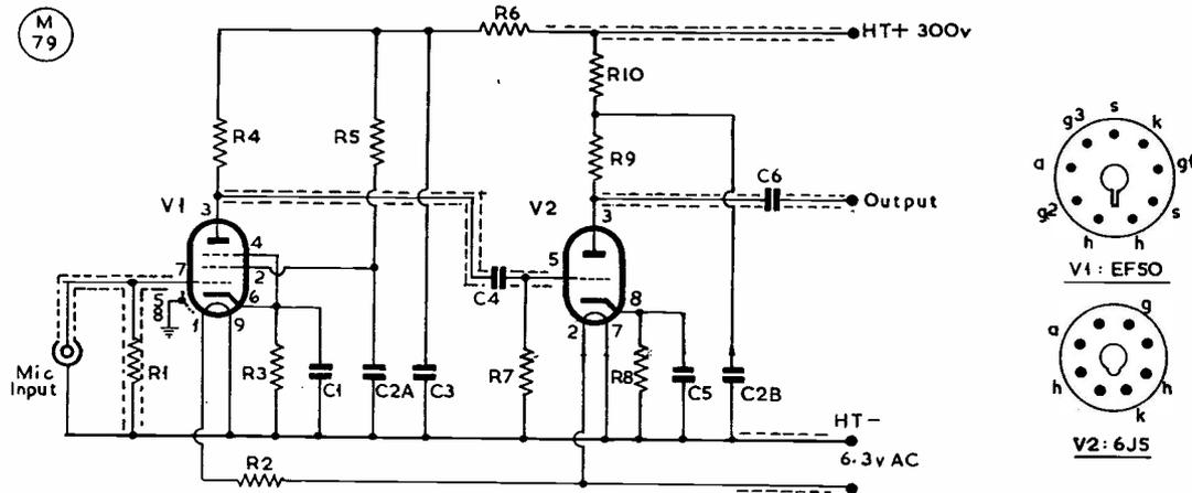
Fig. 1. Circuit of the head amplifier as discussed by G5GQ in the article. An EF50 gives ample voltage gain for the 6J5 in the second stage. To reduce the possibility of hum and because the current drain is very small, the EF50 is run at reduced heater voltage; in this particular application, it does the valve no harm. A condenser microphone is mentioned but a crystal type could be used equally well. The input and output leads should be run in shielded cable.
