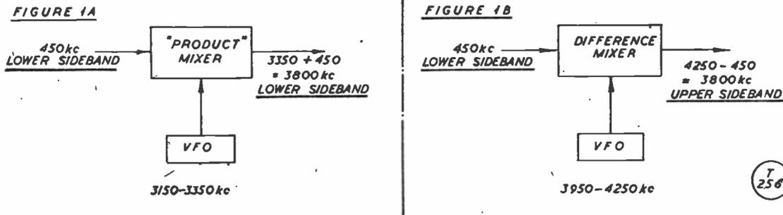
Fig. 1 (A), (B). Showing "product" and "difference" mixing in order to obtain inverted sidebands. The mixer element itself is exactly the same for both systems, the only difference being the VFO injection frequency.
