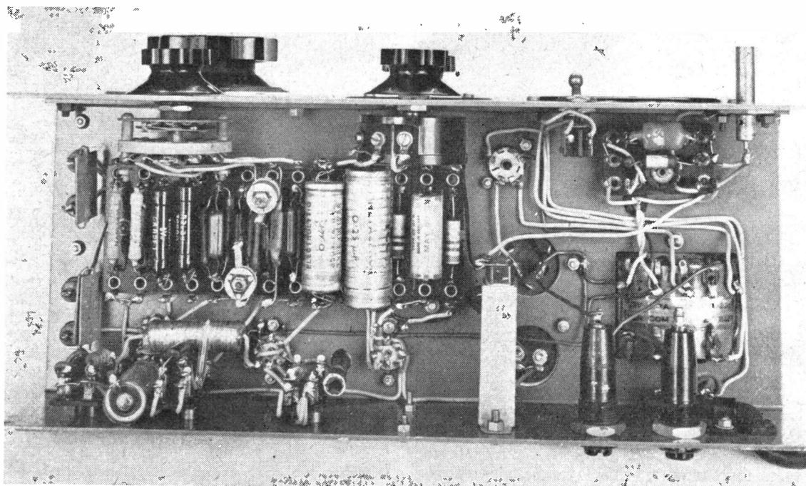
Neat layout under-chassis of the Audio Oscillator constructed by G3AEX, as described. Tag boards are used for grouping resistors and condensers; the decade (range-multiplier) switch is top left, and the fine-control potentiometer RV3 at the centre of the panel drop. As explained in the text, the condensers around the bridge network must be of the close-tolerance type if true decade switching is to be achieved.
