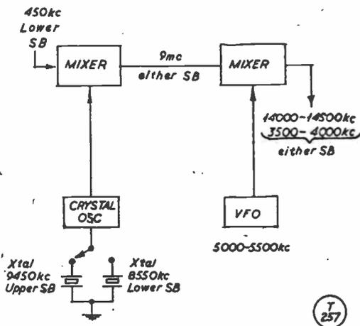
Fig. 2. The double-conversion technique with "product" or "difference" mixing to obtain selectable sideband output. A second IF of 9 mc combined with a 5 mc VFO also provides output on 3.8 or 14 mc, again by using "product" or "difference" mixing.
