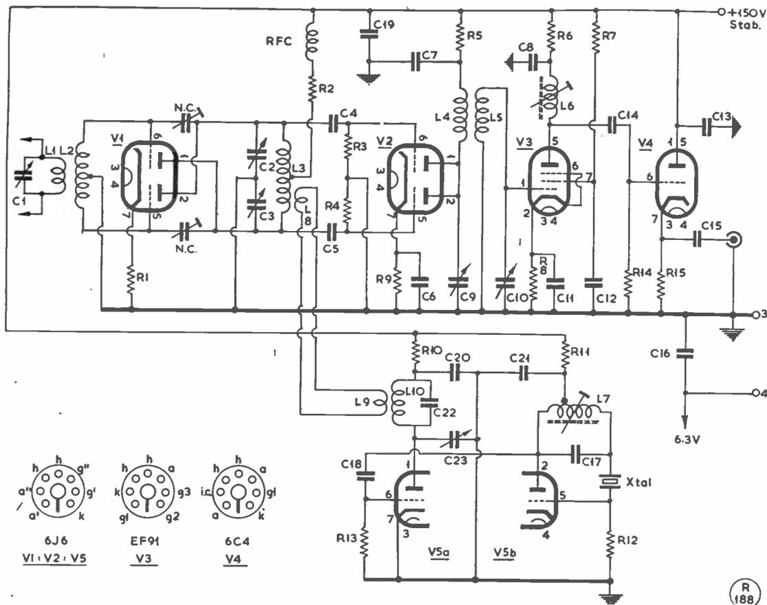
Fig. 2. A crystal-controlled version of the G2IQ converter, as described by G5RZ. It involves an IF amplifier stage V3, and a cathode follower V4. This circuit will not only give a pure T9 beat but also a very strong signal into the main receiver at the IF of 25-27 mc.
