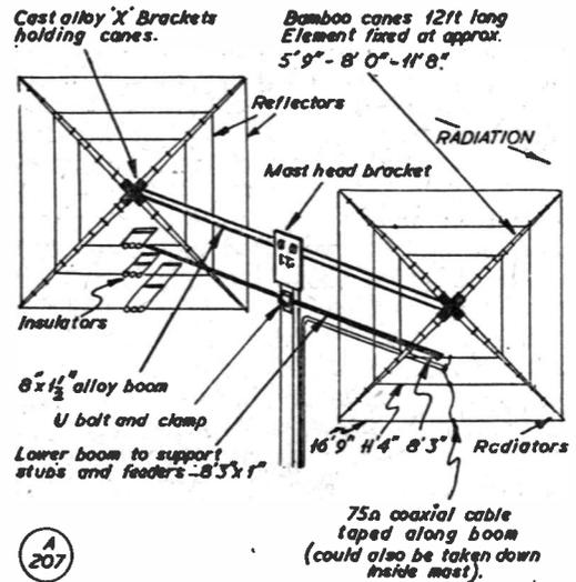
Fig. 4. Full constructional details for the three-band Cubical Quad designed and described by GM3BQA. 14g. wire is used throughout, and the element dimensions given are "each side"; the stub lengths are 25 ins. for 10 metres, 27 ins. for 15 metres, and 54 ins. for 20 metres, and the stubs should be tied back to the boom, out of the way. They can be adjusted to give maximum front-to-back ratio; the gain on each band for the design shown should be about 8 dB.
