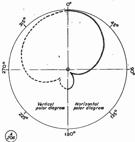
Fig. 3. Polar diagrams obtained on a model of the Cubical Quad for 300-450-600 mc. Only half of each diagram is shown, as they are all symmetrical about the main axis. A full-scale assembly should produce similar patterns.
