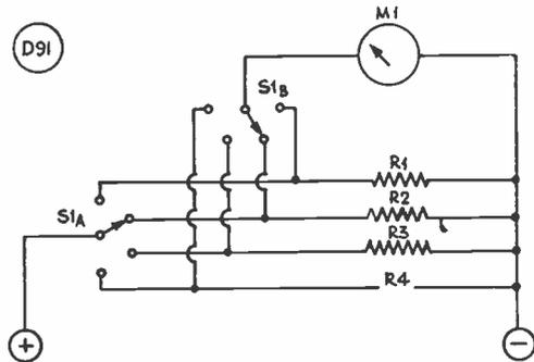
Fig. 3. The meter protective circuit which gives the required shunt facilities without exposing the meter to overload risk.
