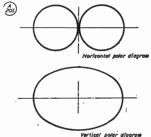
Fig. 2. Polar diagrams for the driven element alone of the Cubical Quad (in free space).
