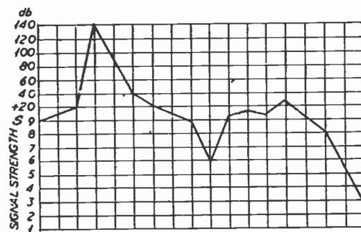
In his observations of the first Satellite, S.I, on its 40 mc channel, G3GGQ obtained these interesting readings. The curves show clearly how the signal level fell off as the batteries ran down. S.II did not last long enough for any useful observations to be made.
