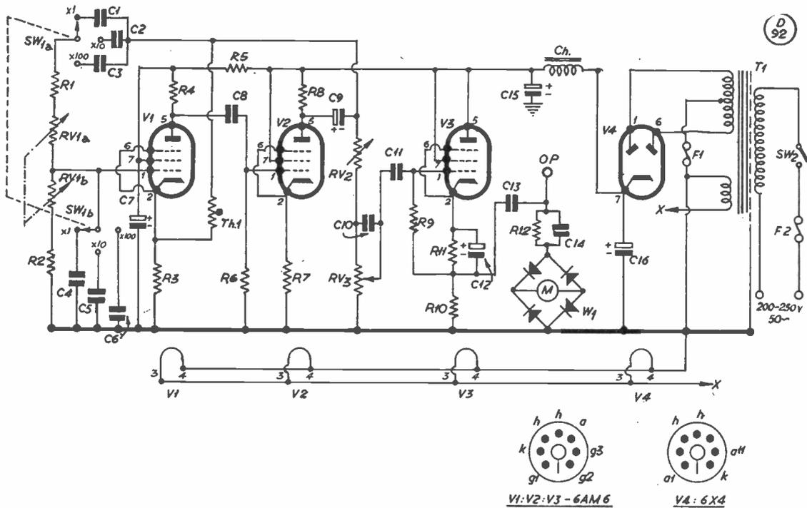
Fig. 1. Circuit of the Audio Oscillator designed and described by G3AEX. By using the specified potentiometer for RV1A-RV1B, the scale calibration given at Fig. 2 could be put on with a reasonable degree of certainty that the output frequencies would be near-enough as marked; alternatively, any suitable linear twin-gang potentiometer can be substituted, in which case the instrument will have to be independently calibrated.
