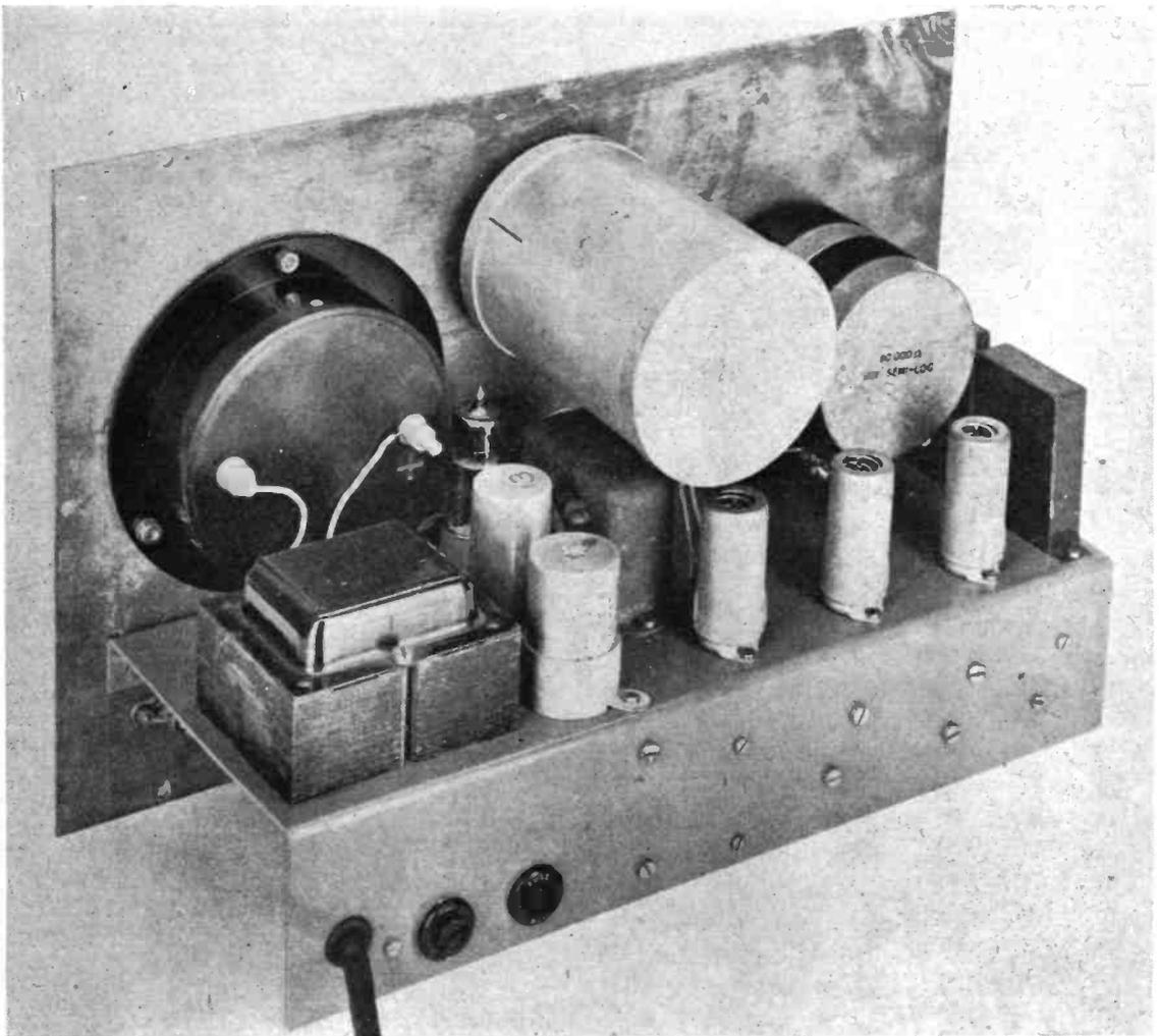
Layout of the Audio Oscillator behind the panel; this is not at all critical, and can be dictated by the parts used and the chassis assembly available. The canned items on the panel beside the meter are the control potentiometers, that on the far right being RV1A-RV1B (see circuit diagram); it is this potentiometer that determines the output frequency and the calibration accuracy of the instrument.
