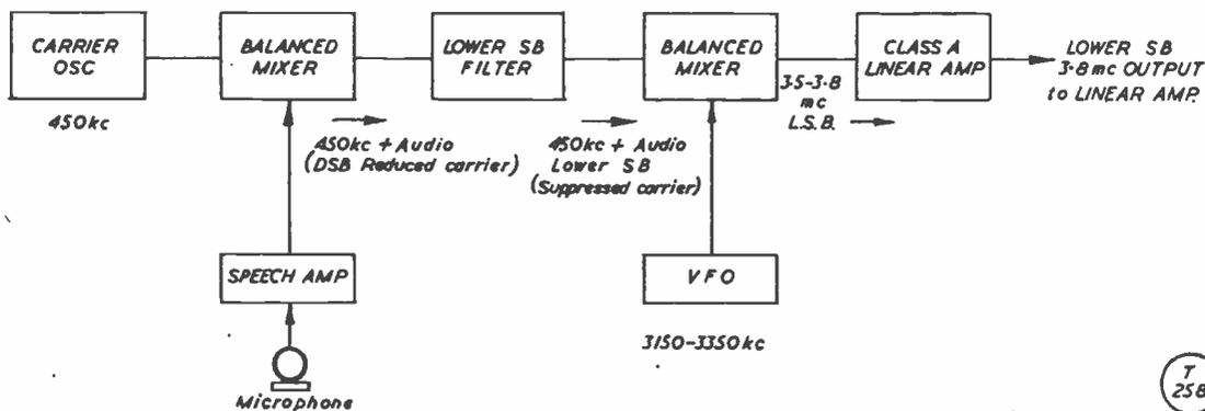
Fig. 3. Block schematic of the G2NH Crystal Filter SSB Exciter, fully discussed in the text. It should be noted that for the purpose of explanation the filter frequency has been taken as 450 kc.
