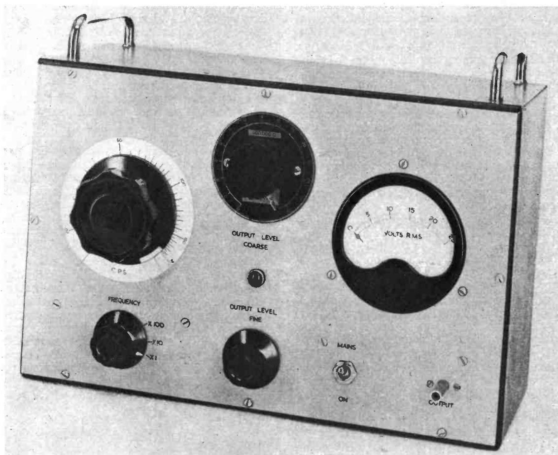
Panel layout of the Audio Oscillator. If the specified potentiometer is used, with the scale shown at Fig. 2., the accuracy of the calibration can be checked by reference to standard-frequency signals; both MSF and WWV radiate audio tones as part of their standard frequency programme. An instrument of the sort described here has many useful applications apart from measuring Doppler shift (for satellite tracking). The output meter has a home-constructed scale, calibrated as explained in the text.
