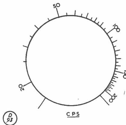
Fig. 2. Actual calibration (half-size scale) obtained by G3AEX on his Audio Oscillator as described in the article. If the specified potentiometer is used for RV1A-RV1B, this calibration can be taken as accurate within reasonable limits.
