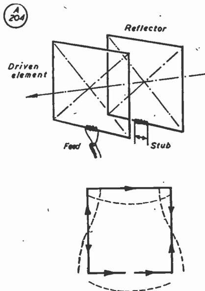
Fig. 1. Layout of the Cubical Quad, and the current distribution in the elements—see text for discussion.
