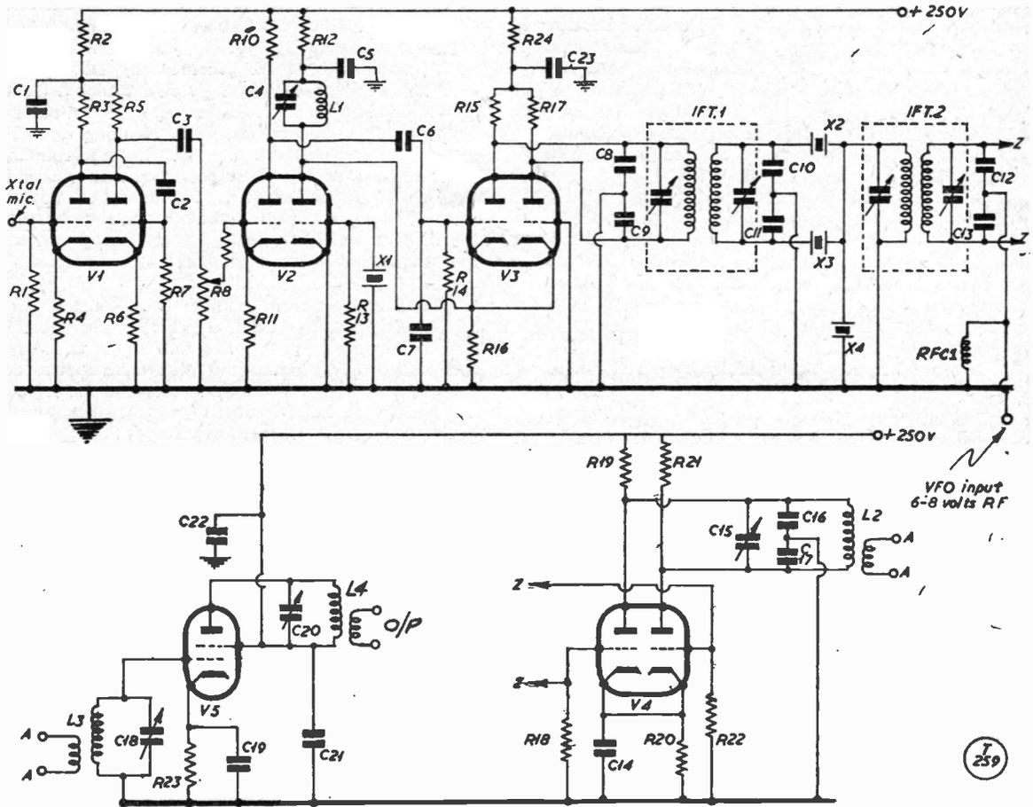
Fig. 4. Circuit complete of the G2NH SSB Exciter, for which all values are given in the table. This diagram should be read with Fig. 3. As mentioned in the article, arrangements have been made for the availability of sets of crystals, X1-X4, for operation with this particular Exciter; suitable crystals from "surplus" sources may also be obtainable, for adjusting to the required frequencies.
