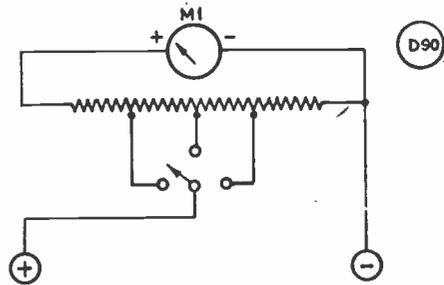
Fig. 2. This shunt arrangement protects the meter but is open to the objections mentioned in the text.
