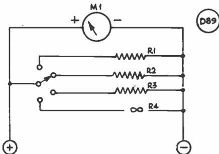
Fig. 1. The usual (and basic) multi-meter circuit, in which R1-R3 are suitable current shunts, R4 gives meter FSD alone, and the meter is a low-current moving coil instrument.
