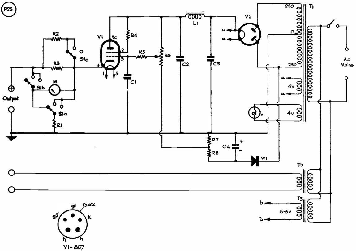
Fig. 6. Circuit diagram of the Variable Voltage Power Supply Unit discussed in the text; some load curves are shown in Fig. 7, from which it can be seen that a useful range of outputs is available. The circuit can be adapted to individual requirements, and the output meter switching arranged for either current or voltage measurements. No particular constructional problems are involved in a unit of this sort.
