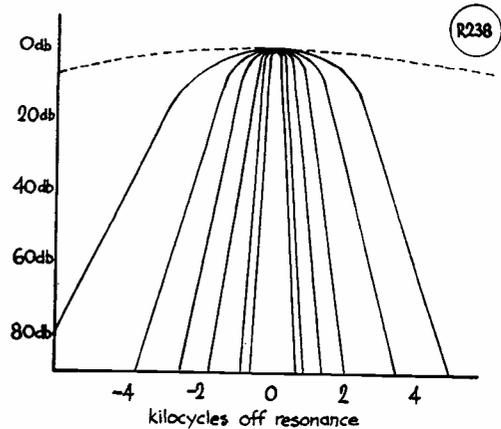
Fig. 4. Selectivity curves on the circuit shown in Fig. 3.
