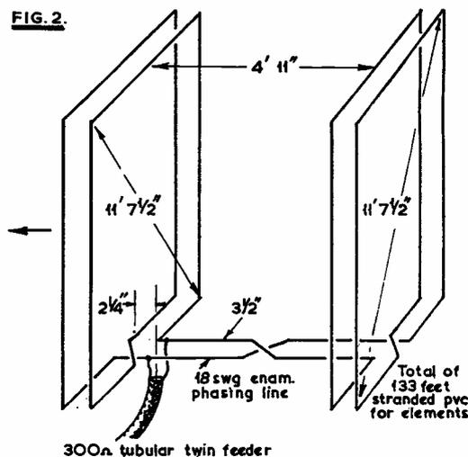
Layout and dimensions of the "Six-TA Special," of which further details are given in the text. The spacing between the elements for each section is one inch (as Fig. 1) secured by the use of the small paxolin corner strips, cut and drilled to the dimensions given in Fig. 1. As explained in the article, the beam is supported on bamboo spreaders fixed to distance-pieces to give a separation of 59 inches between sections. This design is giving very good results on 10 metres.
