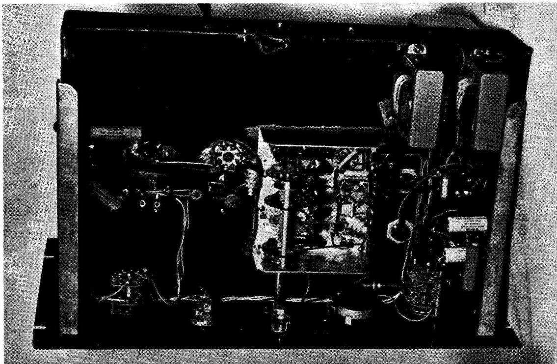
Under-chassis view of the R.A.F. Amateur Radio Society kit transmitter, as wired out ready to go on the air. The smoothing chokes are upper right, and the function switch S3 at lower right. The central assembly is the underside of the Geloso VFO Unit, with the QVO6-20 valveholder to its upper left. The switch below left is the meter change, S2.
