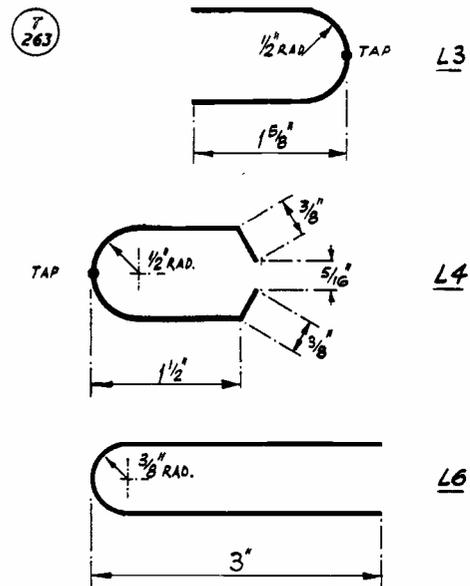
Fig. 2. Dimensions details for the hair-pin inductances in the G3AST 430 mc tripler-PA unit. The wire specified is 17g. Lewmex-M enamelled, which could be substituted by 16g. enamelled copper.
