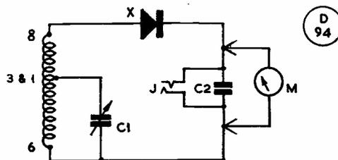
Circuit of the Absorption Wavemeter, using standard Denco plug-in coils. If the indicating microammeter is removed, a headset can be plugged into the jack for telephony monitoring. A piece of apparatus of this sort—costing very little and easier to build than a crystal set—is one of the basic items of test gear in the amateur station.
