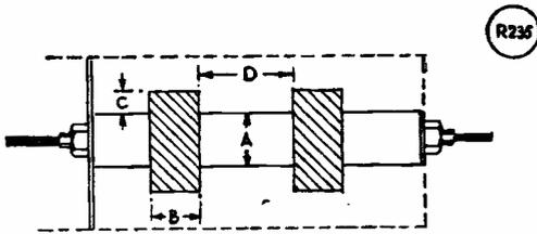
Fig. 1. Diagram of second IF transformers described in text. Approximate dimensions are: A, 0.5 in.; B, 0.4 in.; C, 0.2 in.; and D, 0.85 in. The dotted line represents the screening can.
