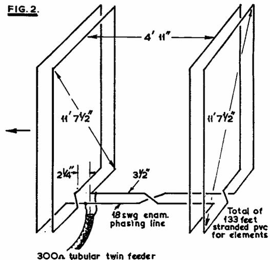
Layout and dimensions of the "Six-TA Special," of which further details are given in the text. The spacing between the elements for each section is one inch (as Fig. 1) secured by the use of the small paxolin corner strips, cut and drilled to the dimensions given in Fig. 1. As explained in the article, the beam is supported on bamboo spreaders fixed to distance-pieces to give a separation of 59 inches between sections. This design is giving very good results on 10 metres.
