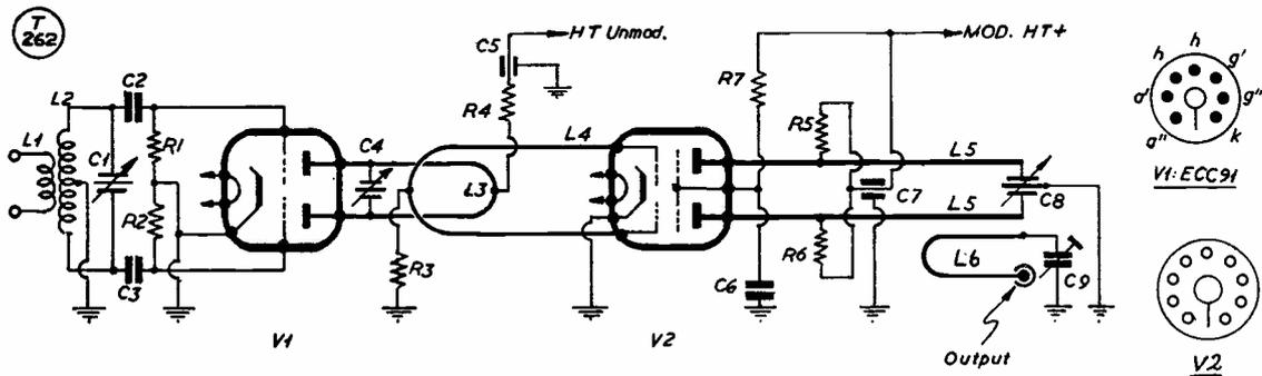
Fig. 1. Circuit of the 70-centimetre tripler-PA unit designed and described by G3AST. The RF output valve is a Mullard QOV02-6, and the general layout arrangement is shown in the under-view photograph. Dimensions for the loop inductances are given in Fig. 2, and all values in the table herewith.
