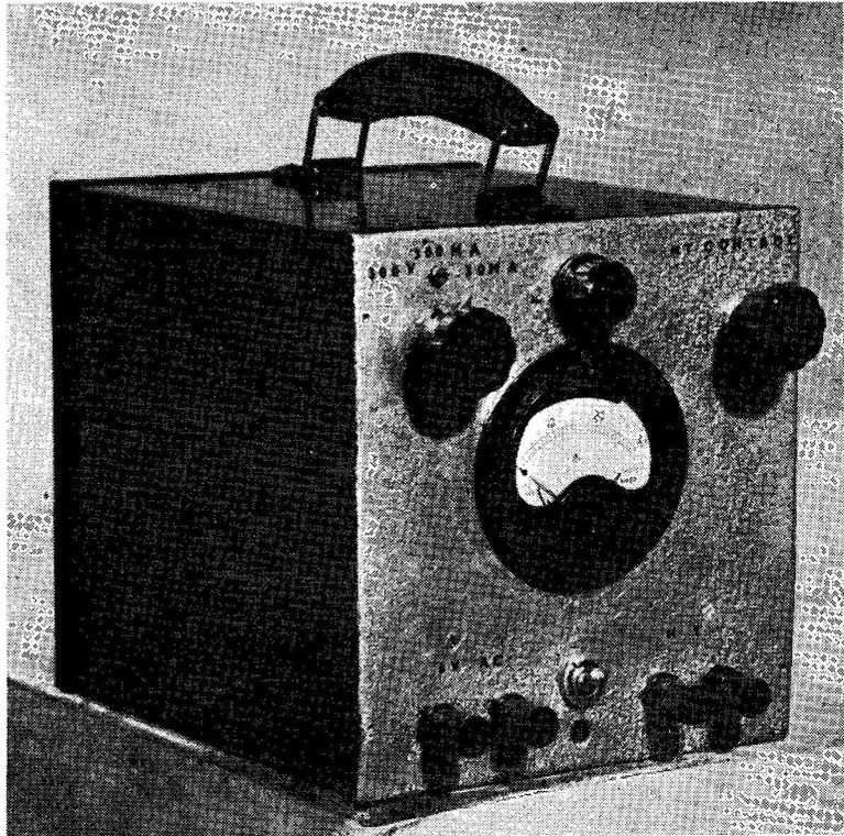
General appearance of the Variable Voltage Power Unit as described in the article. Size can be judged from the fact that the meter is a 2½-inch dial instrument. Output is continuously variable over a wide range by the circuit arrangement shown in Fig. 6.
