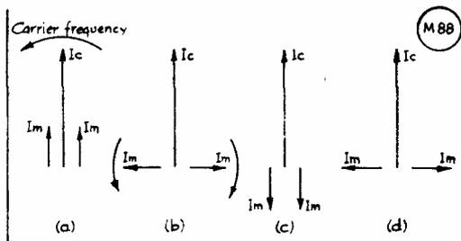
Fig. 1. Showing relative positions of sideband and carrier phases during one cycle of audio frequency with amplitude modulation.  $I_c$  is the carrier amplitude, and  $I_m$  the sideband
