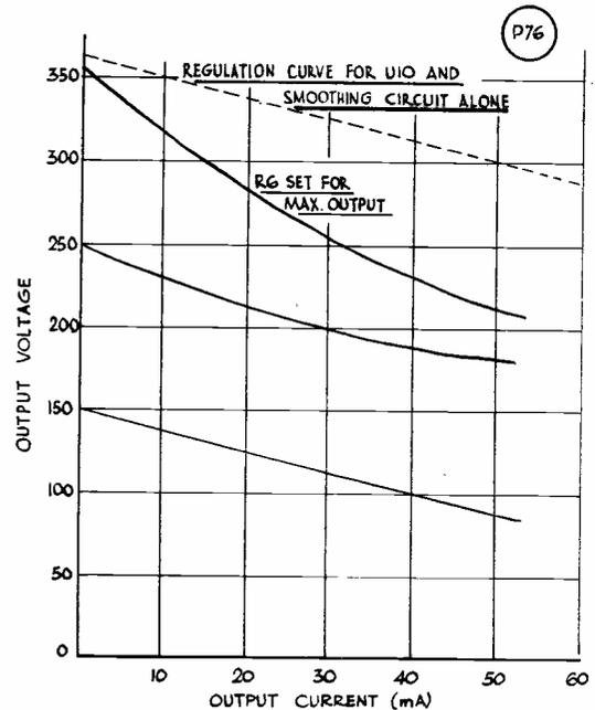
Fig. 7. Output and regulation curves obtained with the circuit of Fig. 6.
