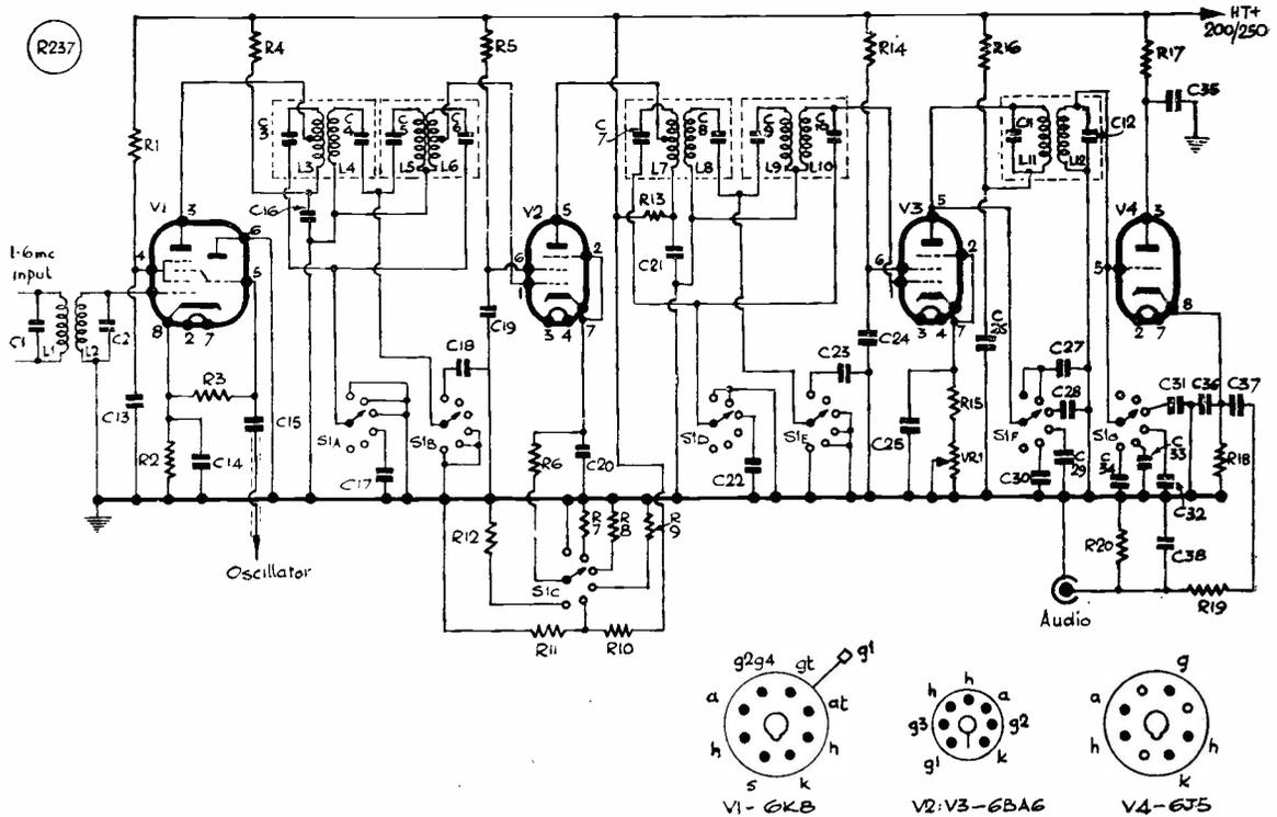
Fig. 3. Finalised circuit proposed for a high-selectivity IF amplifier, for operating at 1.6 mc. Variations on this basic design are possible, as explained in the text ; six different bandwidths are given by the circuit shown here, for which all values are in the table.
