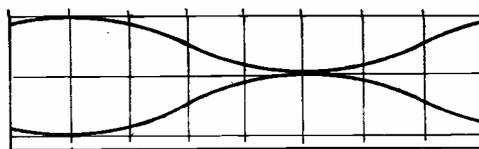
Fig. 2. Carrier and sideband envelope arising from the conditions shown in Fig. 1.
