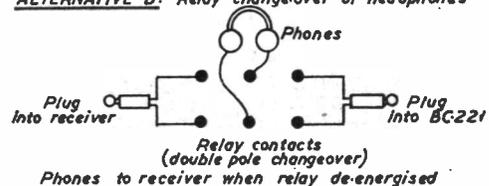
Arrangement suggested by G2NS in order to make full use of a BC-221 as a station CW monitor.
