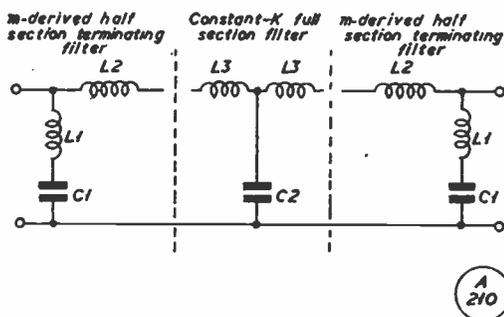
Fig. 1. For this circuit, values would be: C1, 40  $\mu\text{F}$ ; C2, 130  $\mu\text{F}$ ; L1, 0.36  $\mu\text{H}$ ; L2, 0.21  $\mu\text{H}$ ; and L3, 0.345  $\mu\text{H}$ . Fig. 2 shows the practical expression of this arrangement.
