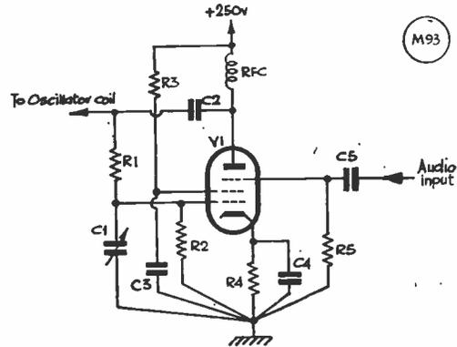
Fig. 7. The difference between this circuit and Fig. 6 is that here the reactance modulator simulates a variable inductance. Values are given in the table, and the valve can be a 6AM6.
