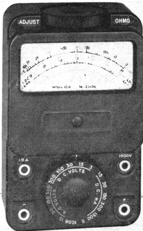
The Taylor Model 122A is a pocket-size multi-range Universal Meter, rated at 5,000 ohms-per-volt, giving 21 AC/DC ranges up to 1500v. AC and 15 amps DC. The Taylor range of test and measuring instruments includes insulation testers, capacity and inductance bridges, valve testers and oscilloscopes.
