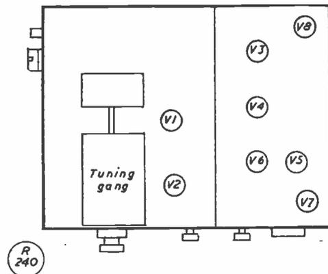
Fig. 2. This sketch is to locate the valve positions and types on the chassis of the CR-300; details of the valves used are given in the article.
