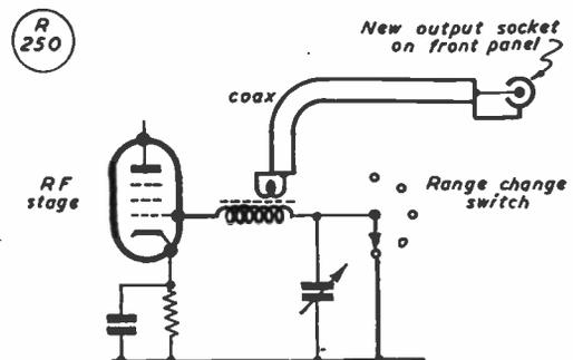
The circuit modification suggested by G3IWL, and applicable to any receiver in which the RF stage coil assembly is accessible. Values are given for the 10-metre band, and the effect is a considerable improvement in sensitivity. The aerial is taken to the additional "output" socket shown.
