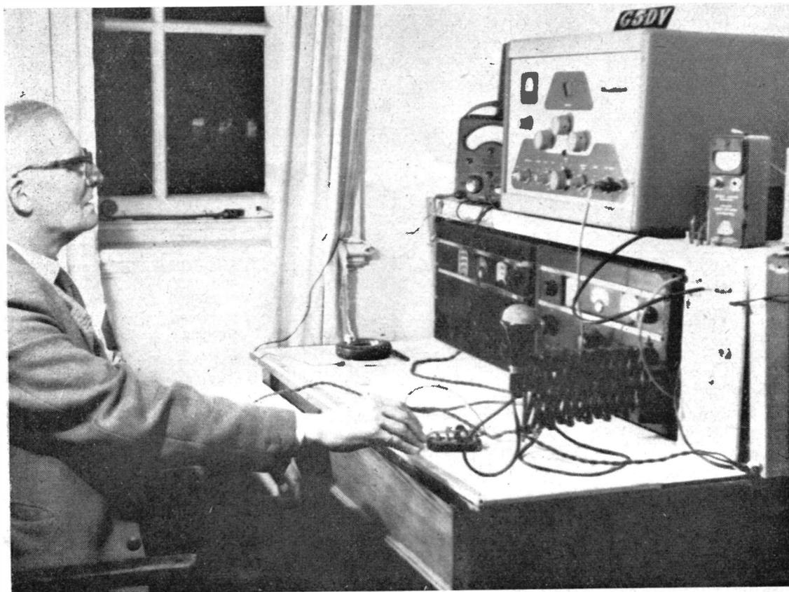
Originally licensed as G5AS more than 25 years ago, the call became G5DV in 1937, and the location is now R.A.F. Upavon, Wilts. The transmitter is a Heathkit DX-100, below which are the two AR88 receivers.
