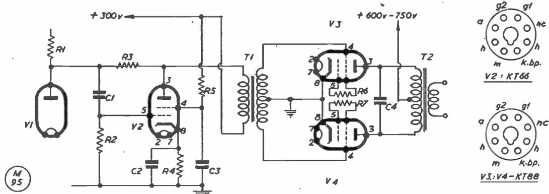
Circuit for the KT88 Class-B modulator, with a KT66 driver stage. With this arrangement, a full 150 watts of audio can be obtained under the conditions stated in the article. The KT66 needs but 15v. grid drive, and in this circuit will produce the necessary 360v. across the grids of the KT88's to drive them to full output. In this application, the G.E.C. KT88 is much superior to the conventional 807, so often featured in Class-B zero-bias modulators.
