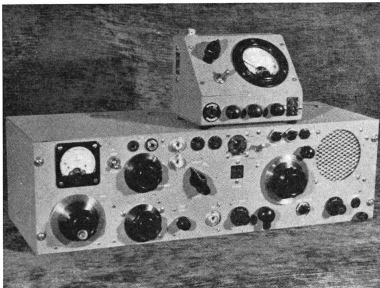
The complete mobile transmitter-receiver-monitor unit installation designed for G3CIM/M, in a Ford Prefect. The monitor box is an important and very useful auxiliary item, the circuit of which is given in Fig. 2. Another photograph shows how the assembly fits into the parcel shelf on the car.
