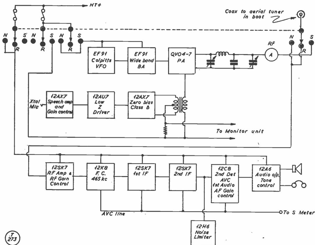
Fig. 1. Block schematic of the G3CIM/M transmitter-receiver layout, showing switching and control circuits. Construction is in unit form (see text and photographs) and the circuitry of the various units of the assembly is conventional. The PA runs up to 7½ watts input, and the receiver section is specially designed for mobile working.
