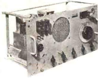
Complete with 6 valves, 2-6K8G, 2-EF39, 6Q7G and 6V6G. Internal mains and 6v. vibrator pack. Built-in 6 1/2" P.M. speaker. Muir-head slow motion drive. B.F.O. and R.F. stage. Provision for Phones and Muting and 600 ohms line combined input, 100/250v. A.C. and 6v. D.C. All sets in new condition and air tested.
