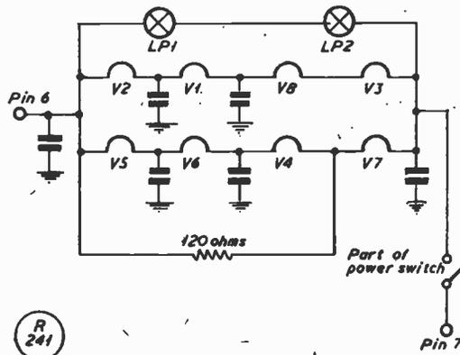
Fig. 3. This is the dial-lamp and heater circuit modification suggested by G8PG, to enable the receiver to be run from a normal LT supply; it is designed for 24v. operation.
