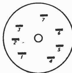
Fig. 4. Sketch to locate the pin connections on the multi-way socket, when viewed from the front.
