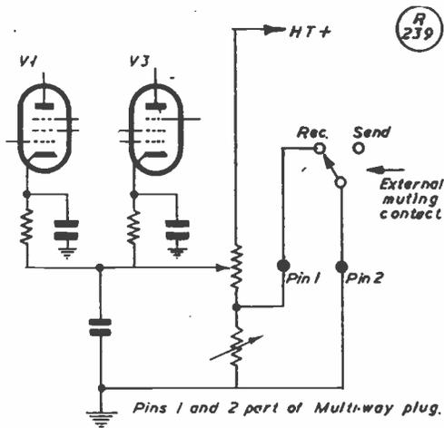
Fig. 1. The "de-sensitising" circuit used in the CR-300, enabling the receiver to be operated near a high-power transmitter; this part of the circuit can be pre-set for monitoring pick-up.
