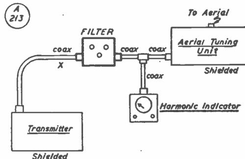
Fig. 4. Connecting the low-pass filter into the transmission line, fully explained in the text. It is necessary to be able to check on the harmonic content in order to adjust the filter correctly.
