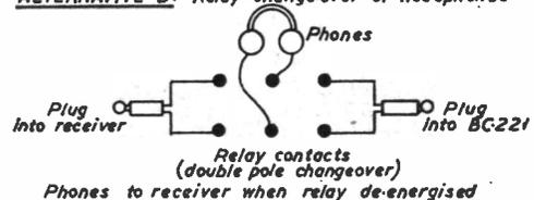
Arrangement suggested by G2NS in order to make full use of a BC-221 as a station CW monitor.
