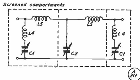
Fig. 2. A practical low-pass filter, as designed by G2HKU. For C1, use a 50  $\mu\text{F}$  air-spaced variable, pre-set, to get 40  $\mu\text{F}$ ; for C2, a 100  $\mu\text{F}$  air-spaced pre-set variable, with a 50  $\mu\text{F}$  ceramic fixed condenser in parallel, to get 130  $\mu\text{F}$ ; L4 is 0.31  $\mu\text{H}$ , which can be 7 turns of 16g. ½-in. diameter by 1-1/16 in. long; and L5 is 0.50  $\mu\text{H}$ , 9 turns as L4.
