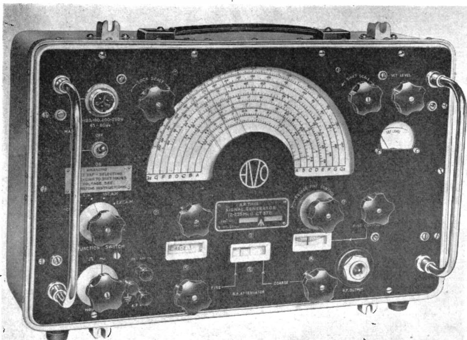
The AVO Signal Generator Type 378 is a CW/AM RF instrument covering the wide range of 2-225 mc; it employs modulation on the post-oscillator stage and provides an amplitude modulated RF signal with negligible FM effect. The Type 378 is ideal for use with AM receivers.
