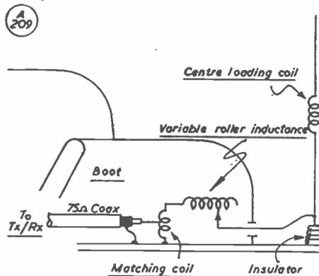
Fig. 3. Electrical layout of the G3CIM/M aerial system, showing arrangement of the loading and matching coils. The variable inductance is roller-tuned by remote control from the operating position.
