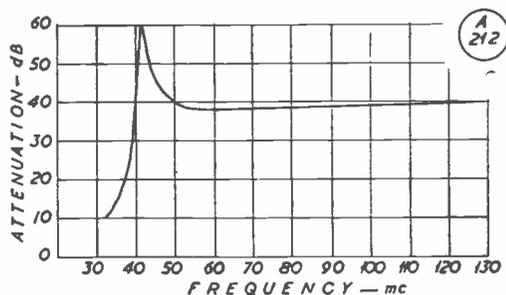
Fig. 3. Approximate theoretical attenuation curve for the design shown in Fig. 2 and the photograph. It has quite a useful cut-off right into the VHF region.
