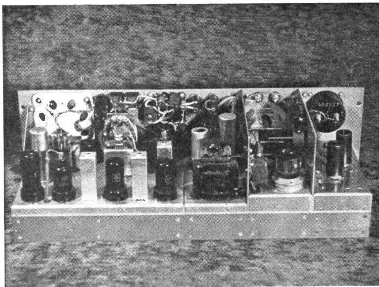
General construction behind the panel of the G3CIM/M transmitter-receiver ; the PA section is second from the right. The receiver runs 12v. valves (see Fig. 1), incorporates a noise limiter, and itself involves seven of the 14 valves used in the complete installation.
