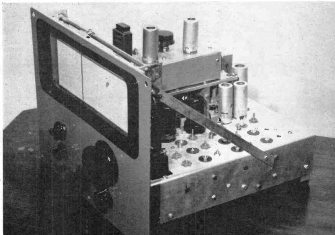
The RF Front End unit designed by G3KGN, to go with his IF/AF Amplifier described in September 1957. The panel controls are RF gain, oscillator set frequency, switch S2, band-change switch S1, the main tuning capacity and aerial trimming condenser C5. Stages V7, V8 are on the sub-chassis above the tuning gang. The dial had not been calibrated when this photograph was taken.
