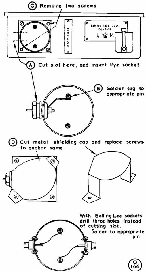
Fig. 2. The switch Type 77A is a useful item for aerial control and change-over in the amateur station. Designed for 24v. operation, it can be adapted as shown here and explained in the text.
