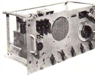
Complete with 6 valves, 2-6K8G, 2-BF39, 6Q7G and 6V6G. Internal mains and 6v. vibrator pack. Built-in 6 1/2" P.M. speaker. Muir-head slow motion drive. B.F.O. and R.F. stage. Provision for 'Phones and Muting and 600 ohms line combined input, 100/250v. A.C. and 6v. D.C. All sets in new condition and air tested.
