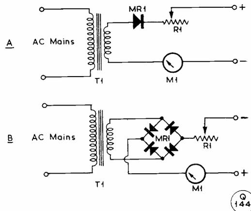
Fig. 1. Alternative circuits for charging 2 to 12 volt accumulators at up to 5 amps. T1 should have a 15v. 5 amp secondary. MR1 is a 5 amp metal rectifier (charging type), R1 is 8 ohms rated 30 watts, and M1 can be an 0.5 amp moving-iron meter for adjusting the charge rate.
