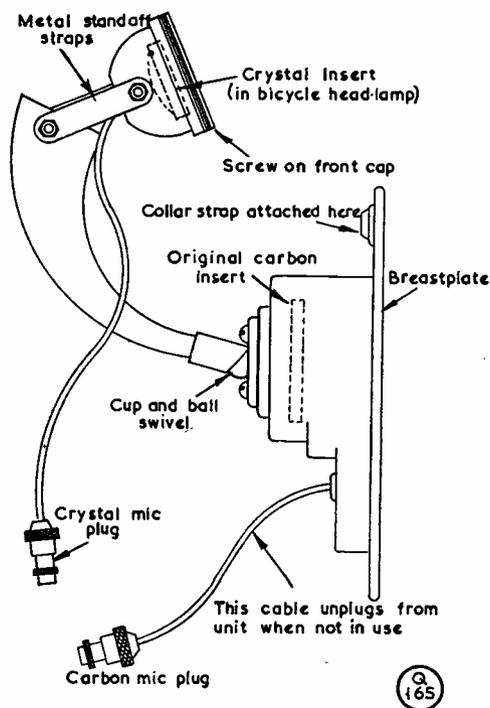
Fig. 1. Adapting a breast-microphone assembly—of the type frequently advertised as "surplus"—to make a mounting for a crystal microphone insert. This arrangement, which retains the original carbon microphone for use if required, makes a convenient and flexible microphone set for general use, either for mobile operation or about the station.
