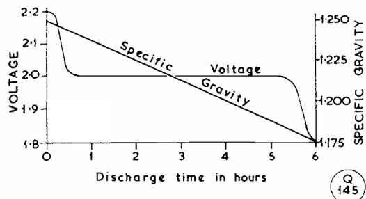
Fig. 2. Typical curves showing how voltage and specific gravity of an accumulator vary during discharge. The article discusses correct charging procedures and general maintenance.
