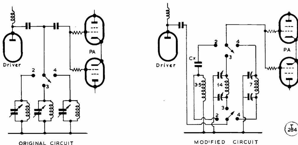
Fig. 2. The recommended modifications for the PA grid stage of the TA-12, to ensure TVI-proofing. If this is not a problem, the grid side can remain as in the original (at left above) except that certain coil changes are desirable, as explained in the text. The value of the condenser Cx in the right-hand circuit is 25  $\mu$ F, and for 7 mc the pi-tank capacities are 80  $\mu$ F each; for 14 mc they are 40  $\mu$ F.
