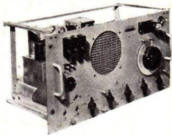
Complete with 6 valves, 2-6K8G, 2-EF59, 6Q7G and 6V6G. Internal mains and 6v. vibrator pack. Built-in 6 1/2" P.M. speaker. Muir-head slow motion drive. B.F.O. and R.F. stage. Provision for 'Phones and Muting and 400 ohms line combined input, 100/250v. A.C. or 6v. D.C. All sets in new condition and air tested.
