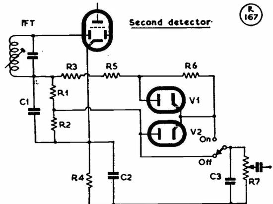
Fig. 1. The noise limiter circuit suggested by G3JBU for incorporation in a BC-342 (or BC-312, which is the same thing except for the power supply). Good results are claimed for this limiter under practical operating conditions.
