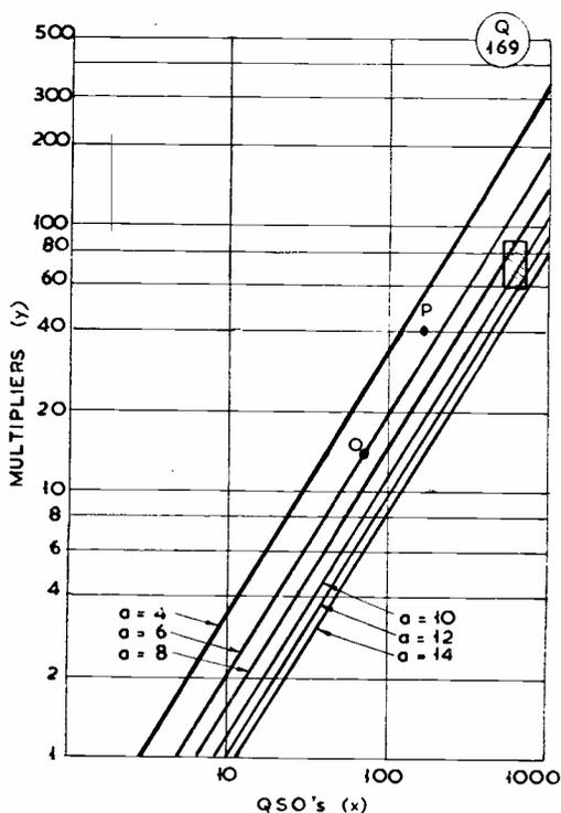
The graphical ready-reckoner evolved by G3HCL to enable one to check progress in a contest; once his argument is grasped, the whole thing becomes perfectly clear, and it is possible to extract the necessary information merely by laying a straight edge on the graph.
