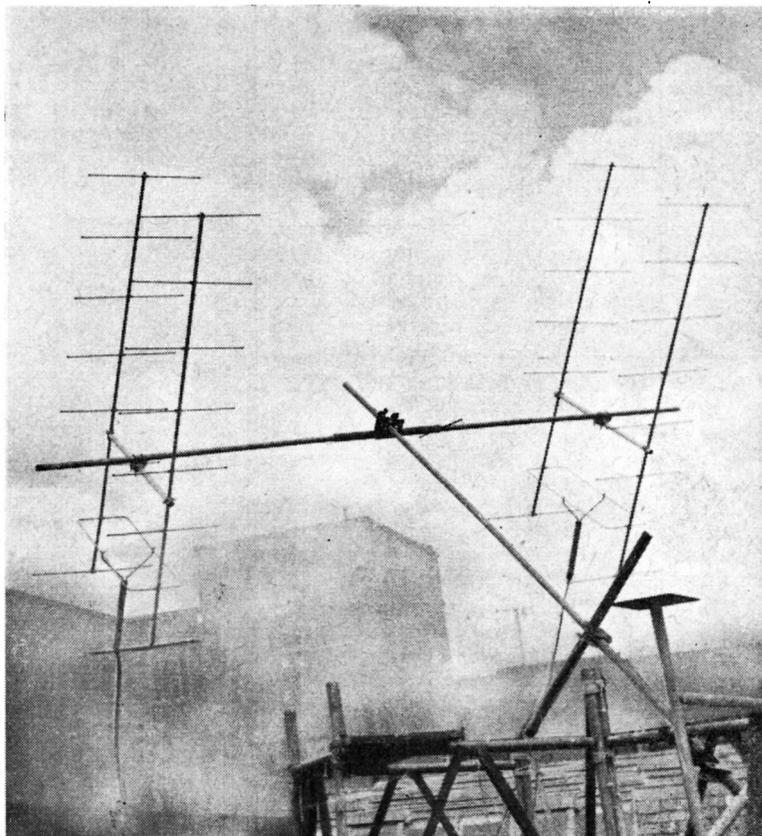
General impression of the radio telescope at Stowe School, Bucks., built up by G3HMO for operation on 200 mc. The array is set on an equatorial mounting, so that the sun can be followed round without any adjustment in elevation being necessary. The aerial system itself is described in the article. Very good results are being obtained, and large "noise signals" have been recorded when the sun is normally active. Noise has also been received from the Milky Way.
