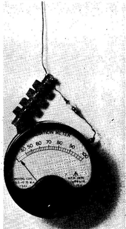
There is virtually no construction involved in the indicating device discussed by G5GQ — but he shows that it has many useful practical applications. The circuit is given in the diagram; it is simpler even than a crystal set, as there is nothing to tune.
