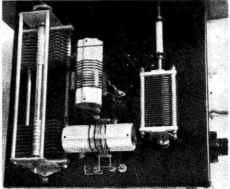
Chassis layout of the Z-Match Unit designed by GW3LJS. The large two-section condenser on the left can be fabricated from a readily available "surplus" type, as described in the text. The L1, L2 assembly and the 80-ohm dummy load resistor R3 — see circuit Fig. 2 — are mounted sub-chassis. The unit is intended for high-voltage operation at full power; for inputs of 75-80 watts with up to 800v. plate HT, condenser spacings could be scaled down.
