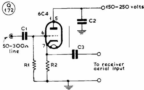
Fig. 2. A cathode-follower T-R switch. Resistors are 1-watt non-inductive, and the input and output circuits should be screened to prevent feed-through coupling. Values are: C1, 50  $\mu$ F, 500v.; C2, .005-.01  $\mu$ F; C3, .01  $\mu$ F; R1, 1 megohm; and R2, 500 ohms.
