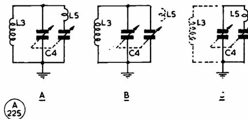
Fig. 1. Basic circuitry of the RF tank section of the Z-Match Unit. (A) is the ATU circuit, with link couplings omitted; (B) is the ATU equivalent circuit for the range 3.5 to 7.0 mc; and (C) is the configuration for 14-30 mc.
