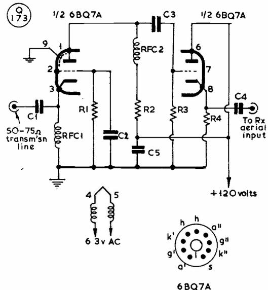
Fig. 3. A much more refined type of T-R switch, using a twin-triode. Values are: C1, 500  $\mu$ F; C2, C4, .01  $\mu$ F; C3, C5, .001  $\mu$ F; R1, 1 megohm; R2, 1000 ohms; R3, 50,000 ohms; R4, 100 ohms; RFC1, 2.5 mH; RFC2, 21  $\mu$ H (10-metre) RF choke; Htr. 4/5, bi-filar wound. All resistors are  $\frac{1}{2}$ -watt non-inductive. RFC2 is a single-layer VHF-type RF choke, and is not critical; the special bi-filar choke, in the heater leads, is explained in the text.
