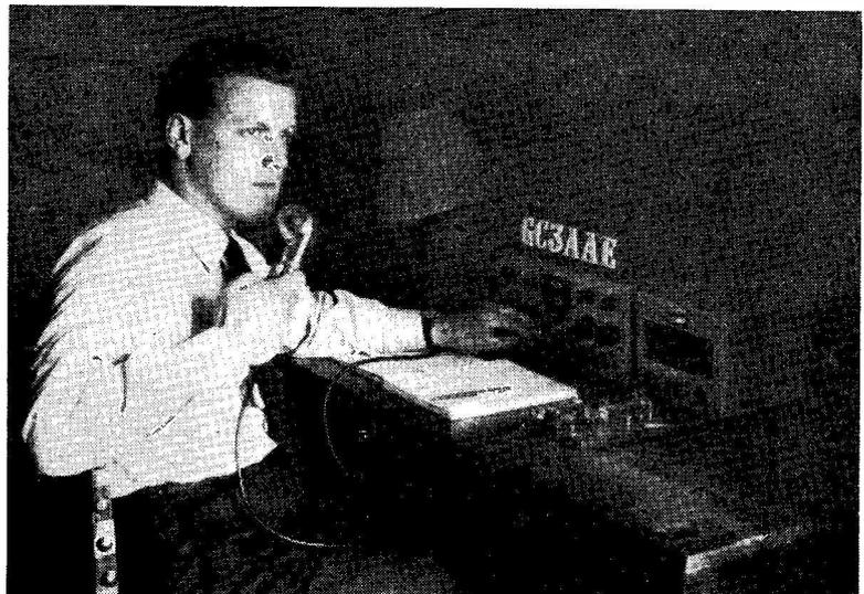
G3AAE when signing GC3AAE on the SSB expedition to Alderney, Channel Islands, during the latter part of May this year. With G3BQR, G3IFB and G3JUL to assist, GC3AAE was kept on the air 24 hours a day for a fortnight, using a Collins KWM-1 transceiver with 150w. input, the aerial being a G8KW multi-band system. Between them, the four operators made more than 2,000 contacts in 112 countries on the 14-21 mc bands.
