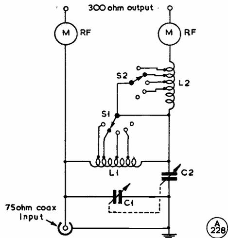
Fig. 2. A practical expression of Fig. 1, for which values are given in the table.. M are 2 amp. RF ammeters.
