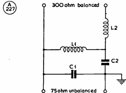
Fig. 1. Basic circuit of the balancing network, for 75 ohms into 300 ohms.
