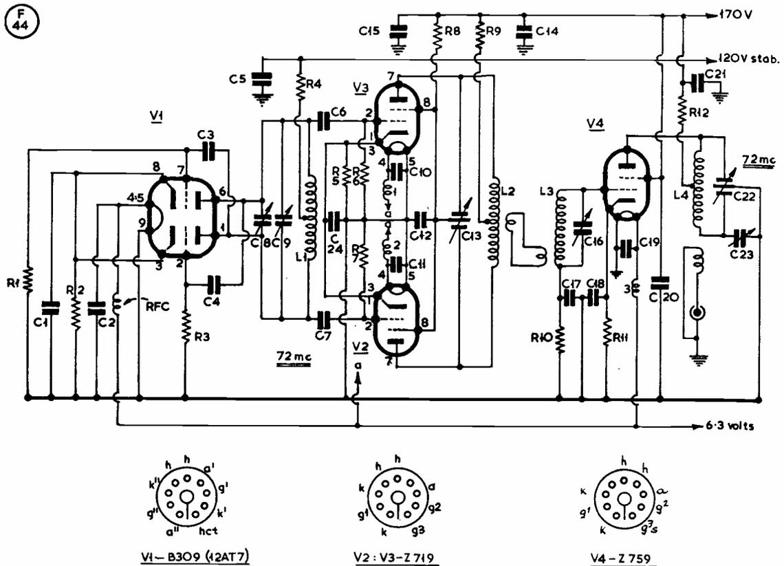
Fig. 1. Circuit of the 70-72 mc VFO unit designed and described by G2JF. A Kallitron oscillator is used to generate the fundamental frequency, the other two stages being buffer-isolators. All three stages are on the same frequency, very loose coupling and careful screening being used between stages. An RF output of about one watt is available for doubling into the two-metre transmitter, with excellent stability. A stabilised HT supply should be used for V1.
