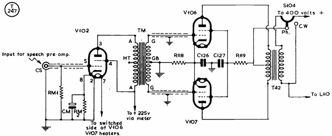
Fig. 3. The original crystal oscillator V102 is modified to serve as the modulator driver, so that a crystal microphone can be used. The original switch S104, intended for CO crystal selection, is rewired to work as the Phone/CW change-over in place of the relay K101.
