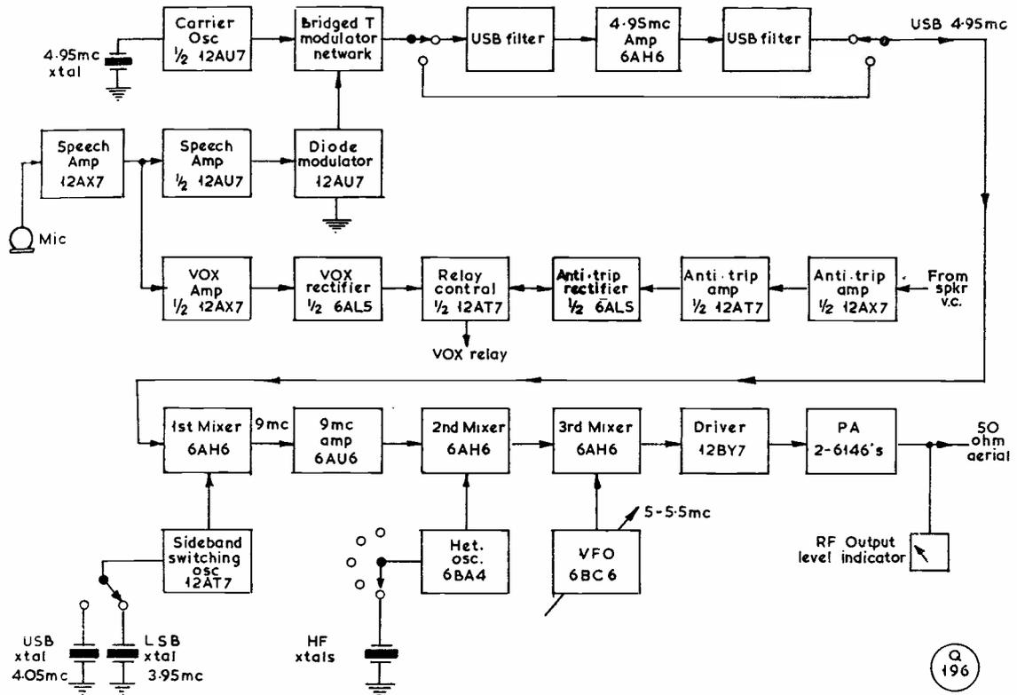
Fig. 6. Simplified block diagram of the Hallicrafters Model HT-32 transmitter-exciter. This equipment will operate in the 80, 40, 20, 15 and 10 metre bands, on either SSB, DSB or CW. An HF crystal sideband filter of unusual design, working on 4.95 mc, is a feature of the HT-32.
