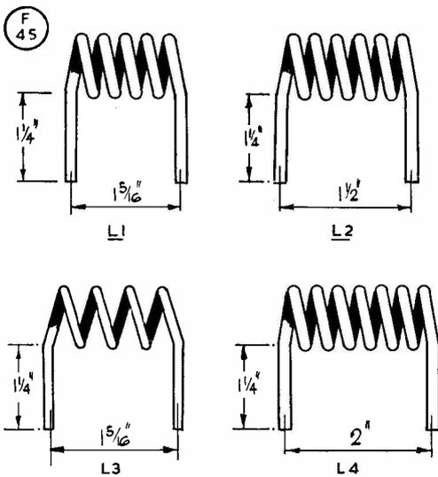
Fig. 2. Detail of the coil windings for the VHF VFO, the sizes for which are given above.
