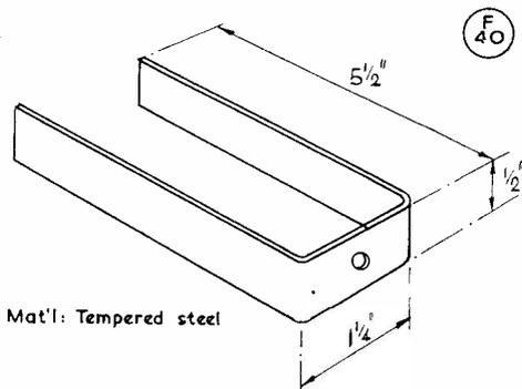
Fig. 2. Dimensions of the tuning fork used by G3BST. The total length is  $13\frac{3}{4}$  inches, with  $\frac{5}{8}$ -in. allowed for the bends. The mounting is shown in one of the photographs. It can easily be home-made—see text.
