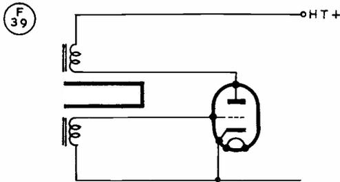
Fig. 1. The basic tuning-fork oscillator circuit. With careful construction and setting up, a high degree of frequency stability can be attained.
