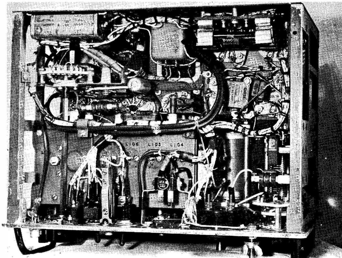
Under-chassis view, after modification. Compared with the original it will be seen that the wiring has been considerably simplified. The 4-point power plug, replacing the original 16-point power and inter-connection plug, is at bottom centre. The grid leads for the modulators V106, V107 are in coax and go to the DT1 driver transformer on the upper side of the chassis.
