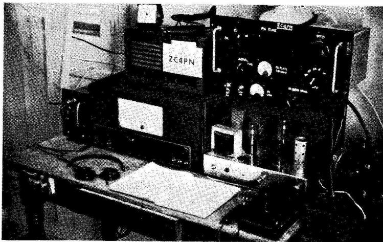
ZC4PN, Nicosia, Cyprus is G3ICH and has also been DL2SU. He started up under the ZC4 call in November 57, running a Gelson VFO with an 807 PA on the 7-28 mc bands, and an Eddystone S.640 receiver; aeriels are dipoles for each band, with a 2-ele beam for 10 metres. In about a year's not-too-concentrated operating, 100 countries have been worked.
