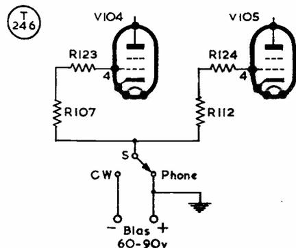
Fig. 2. The protective bias arrangement for the PA stage; in the phone position the bias voltage is removed and R107, R112 are connected direct to earth. Switch S is a SPDT toggle.
