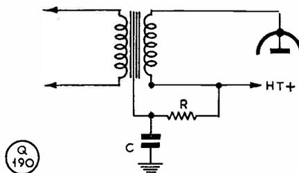
By this simple circuit arrangement the core of an audio transformer can be brought up to an HT potential approaching the voltages being generated across the winding nearest the core, thus reducing considerably the danger of breakdown. Suitable values are: R, 100,000 ohms; and C, anything from 1 to 8  $\mu$ F.
