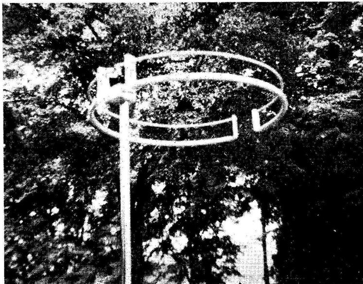
The two-metre halo now being used by G6VX/M, Cheltenham. This is an interesting design and is most effective, London stations having been worked from the hills above Cheltenham. The feed impedance is 75 ohms and some further details are given in the text.
