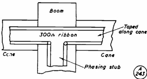
Fig. 3. The beam elements consist of lengths of 300-ohm ribbon, to the dimensions of Fig. 4, taped to the bamboo spreaders.
