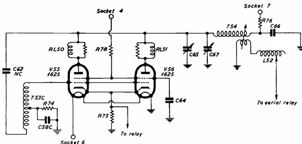
Fig. 2. The PA side of the CCT-52232 Command transmitter, running a pair of 1625's (12v. 807's). For the Top Band modification, the only alterations needed are the removal of one 1625 and the shorting of its heater connections; the removal of L52; and an increase in capacity on C67. The work involved in getting the CCT-52232 Command Tx on to 160 metres can actually be done in about an hour.
