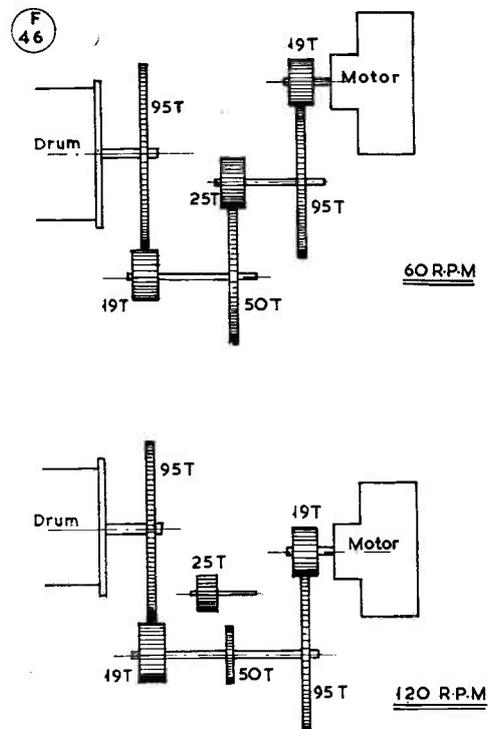
Fig. 6. Sketch showing gear layout and tooth ratios to get correct turning speeds — see text.
