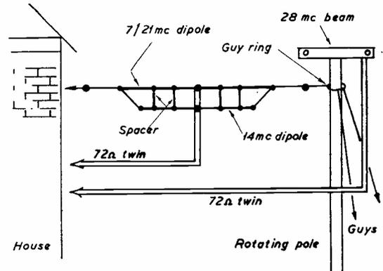
Fig. 1. General layout, showing the 7/21 mc dipole (half-wave on 7 mc, into three half-wave on 21 mc), with the 14 mc dipole physically "in parallel." The 10-metre ZL Special is on the rotatable pole, the dipole array acting as a horizontal guy. A sleeve or ring at the top of the mast is the termination for all three guys; the pole rotates in this ring and in a drain-pipe support at the foot. The 10-metre beam is fixed to the top of the pole at the point of balance.
