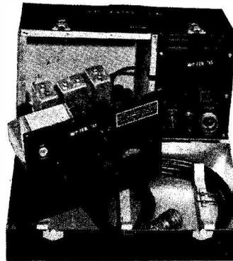
115 volt 6X5G power pack in separate compartment of attractive light-weight black crackle case.
