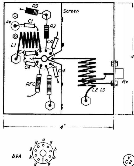
Fig. 2. Physical layout sketch for the RF pre-amplifier, as constructed by G6TA. It should be noted that by using a tinned metal chassis, good ground connections can be made; in the model, the screen is soldered to the shell at four points, and also to the spigot of the valveholder; note that four by-pass capacities C4 are used. All other details are given in the text.
