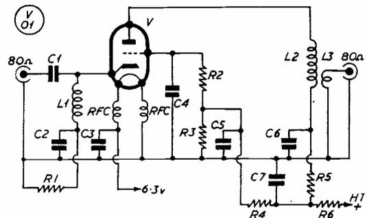
Fig. 1. Circuit of the RF pre-amplifier for two metres, described by G6TA, using a GEC A2521 UHF triode. This valve is capable of high gain with excellent stability. A suggested form of construction for the amplifier is shown in Fig. 2.
