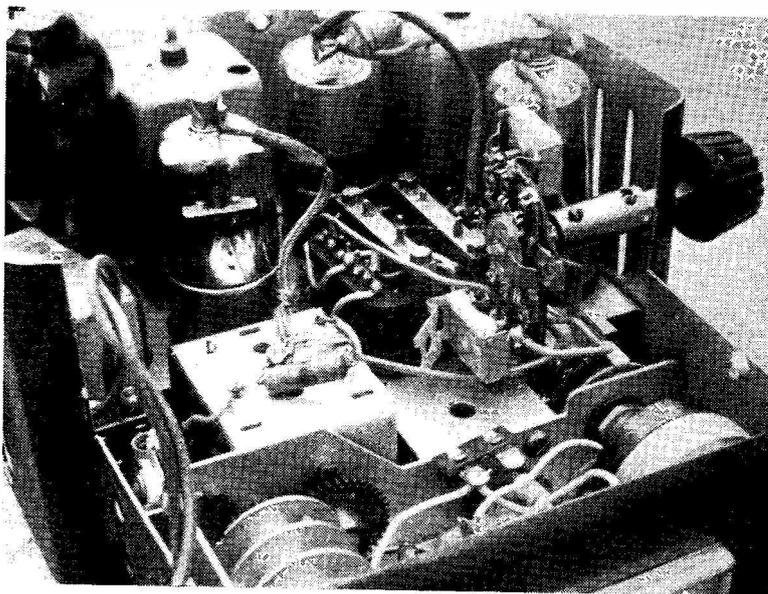
The modification devised by G2FWA to get the Masteradio model 700/701 car radio receiver on to Top Band. The only additional items are the switch, the trimmers (one shown opened out) and the resistor seen on the tuning condenser gang, this being to provide a grid return for the mixer. The view is looking into the receiver with its panel to the front of the photograph.
