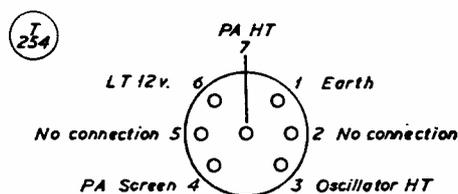
Fig. 3. The power socket for the CCT-52232 Command transmitter, viewed from the rear. No external connections are made to pins 2, 5, but internally pin 2 is connected to the centre-tap of the PA grid coil, and pin 5 to the two relays (which are either removed or made inoperative).
