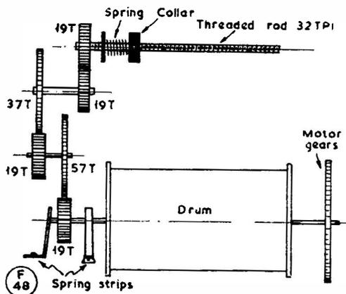
Fig. 8. The gear-train layout for the drum and the transverse drive for the stylus.
