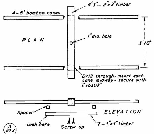
Fig. 2. Construction of the frame for the 10-metre "ZL Special." The cane lengths on which the dipole elements (made up of 300-ohm ribbon) are supported are themselves secured by a 4 ft. length of 1-in. by 1-in. wood strip, as shown in the elevation.
