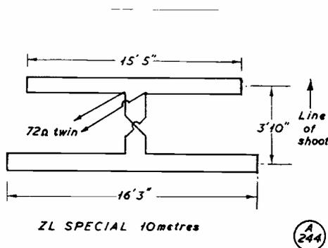
Fig. 4. Element layout for the 10-metre ZL Special, using 300-ohm ribbon feeder throughout. The transposition, or cross-over for the phasing line, is obtained merely by twisting the 46-in. length of ribbon connecting the centres of the sections.
