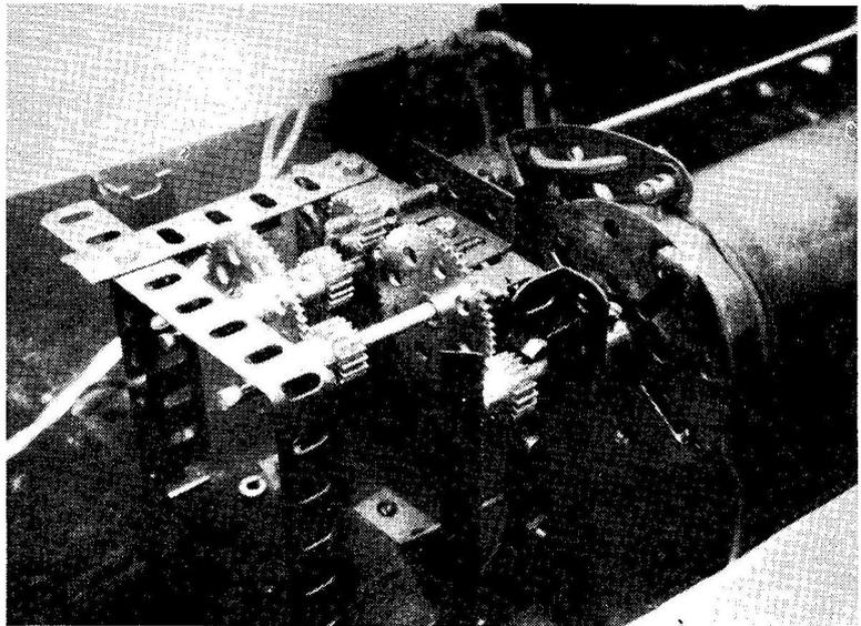
The Meccano gear-train used for processing the stylus across the drum in the facsimile receiver designed and constructed by G3BST. Good charts are produced from Met. stations in many parts of the world, the degree of transcription error being so small as to be negligible.
