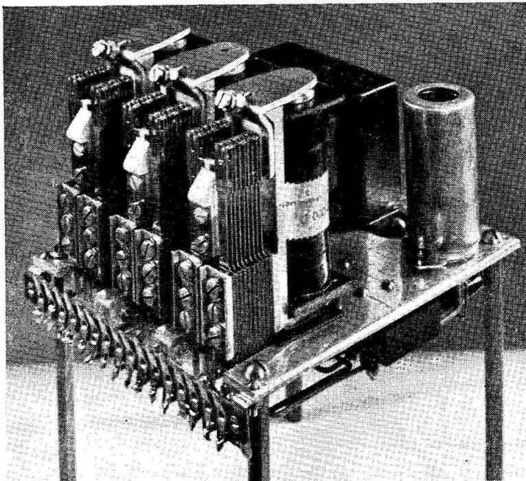
The transistor control circuit assembly, discussed in the text. The valve on the right supplies 36v. for the transistors, but has since been replaced by a small silicon rectifier. All connections for the control circuitry are made to the tag strip at the front of the chassis.
