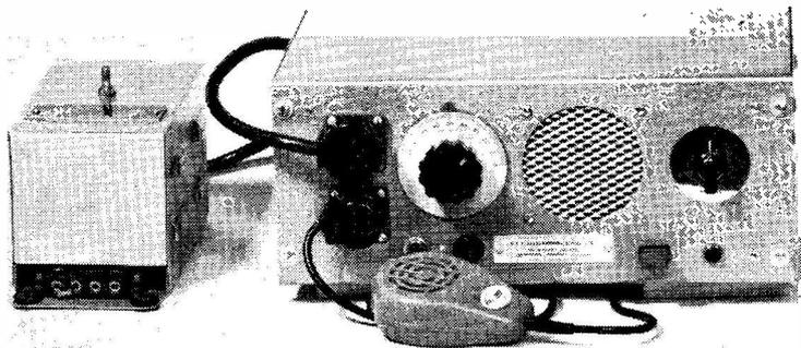
The new R.E.E. Communicator Mk. II is a VHF transceiver specially designed for mobile operation on two metres. The receiver section is a double-superhet, tuning 143-147 mc, with noise limiting. The RF power amplifier in the transmitter is a QQVO3-10A, screen modulated by a 6BW6. Size overall is 5½ ins. high x 13 ins. wide x 8 ins., deep.
