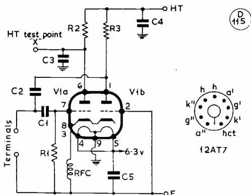
Fig. 1. Basic circuit of the test unit described by G5JU, which has several very useful applications.
