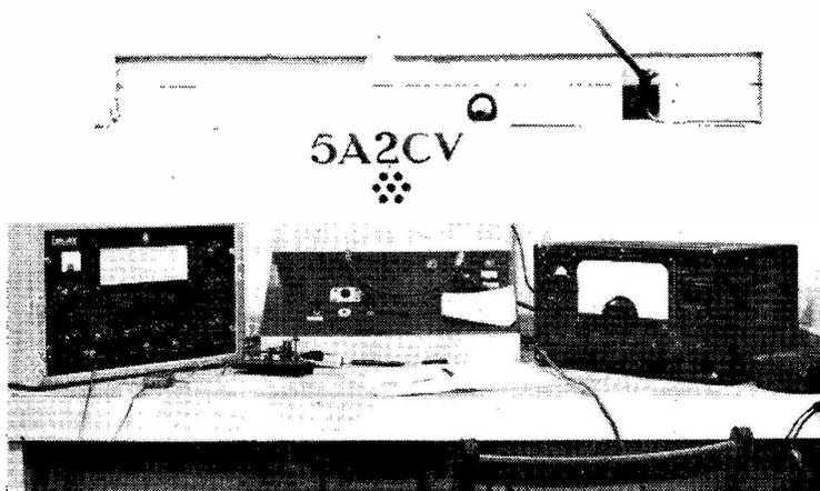
5A2CV, Tobruk, is an RAF-ARS club station, where they run a Panda Explorer as transmitter, with a Radiovision Commander receiver. Bands worked are 40-10 metres, CW and phone, and the 5A2CV boys are always glad of a call from U.K. stations. This winter, they hope to be on 1,825 kc with a half-wave aerial positioned for Top Band working in this direction. For those fortunate enough to QSO, it will be a new country and another continent.
