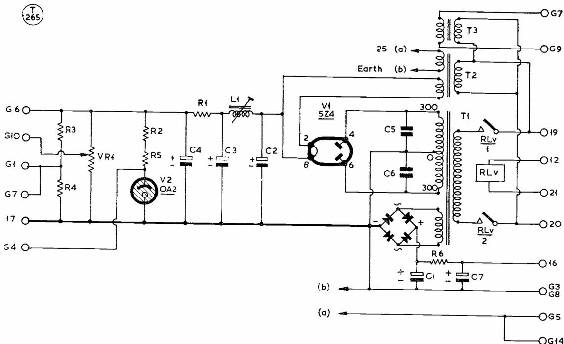
Fig. 5. Circuit of the low-voltage power supply unit for the all-band transmitter. Numbered connection points key with the other circuit diagrams.
