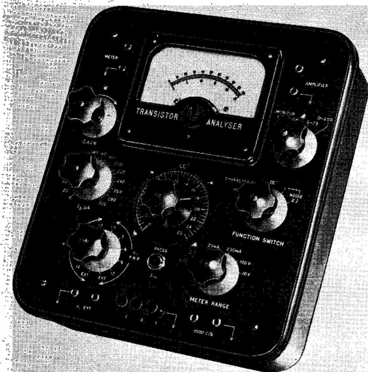
The new AVO Transistor Analyser is a battery-operated instrument suitable for testing small and medium n-p-n or p-n-p transistors. Provision is made for the measurement of transistor noise by comparing peak noise against an equivalent signal calibrated from the internal 1000 c/s oscillator. The Analyser can also be used as a multi-range test meter for servicing transistorised apparatus.
