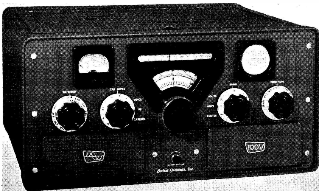
A new phasing-type exciter-transmitter, the Central Electronics 100V, for which the block diagram is shown in Fig. 7. The main dial is for VFO control, and is calibrated 1 kc per division. A 2-in. oscilloscope is incorporated for output monitoring. All adjusting controls (such as audio gain, balancing potentiometers and bias setting) which once set up are seldom touched, are mounted behind the lower escutcheon doors; these are held closed by magnetic locks.
