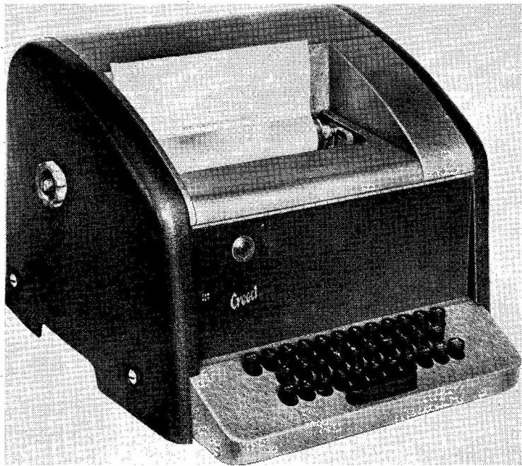
The Creed Model 75 page-printer is a fine example of a modern teleprinter instrument, produced by a British firm with a world-wide reputation for high-grade telegraph apparatus. The Creed 75 is not yet to be found at "the average amateur RTTY station" but is the sort of machine to which all keen radio teleprinter operators will aspire, nevertheless!
