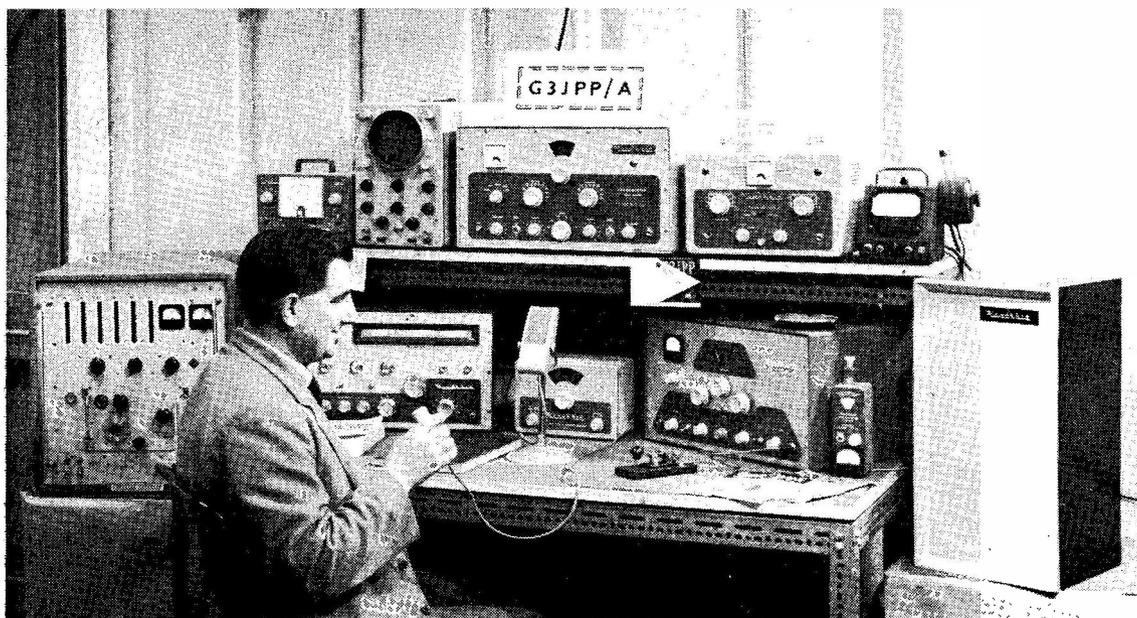
The all-Heathkit station established at the Daystrom Factory just outside Gloucester, on the Bristol road. Signing G3JPP/A, the gear includes a Heathkit DX-40U, a DX-100U, a Heathkit Mohawk receiver (at left, on the table) and various items of test gear and measuring equipment. The DX-100U as supplied in the U.K. is the central piece on the upper shelf.
