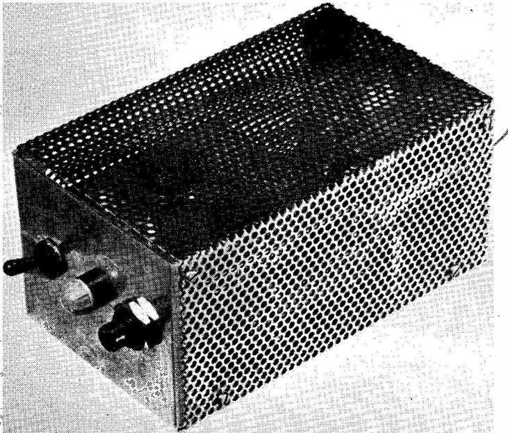
Neat finish and construction of the DC converter described in the article, using power transistors in the primary switching circuit, to give outputs up to 30 watts at 300 volts, at high efficiency.
