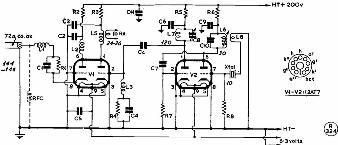
Fig. 3. A double twin-triode crystal-controlled converter circuit, using a pair of 12AT7's, and designed for a receiver tuning 24-26 mc to cover the two-metre band. Injection is at 120 mc, and the mixer output is peaked at 25 mc. A circuit of this kind, built as a small unit to fit inside the main receiver, could take power from it and would extend the range of almost any communications-type receiver into the two-metre band.
