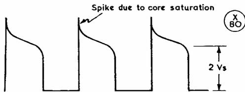
Fig. 2. The emitter waveform with a switching time of about  $30 \mu\text{S}$  — see text for discussion.
