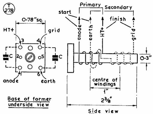
Fig. 2. Dimensions of former and winding details for the wide band couplers described in the article.
