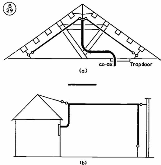
Fig. 1 (a). Layout for an indoor aerial, which can give very good results if installed as suggested in the text. The roof-space is always a suitable location for HF aerials if no outside arrangement is convenient or possible.
