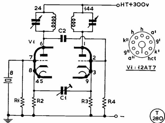
Fig. 1. About the simplest possible circuit for a two-metre crystal oscillator. The RF output at 144 mc will not be much, but it will be in the band. An 8 mc crystal is multiplied up in the sequence shown, and values are given in the table. The valve is a 12AT7.
