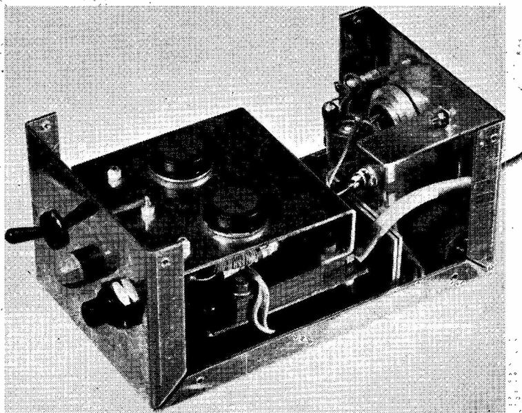
Upper chassis view of the transistor power unit designed and built by G3KUM, showing mounting of the power transistors and the general component layout. The final size is only 3 ins. by 3 ins. by 4 1/2 ins. overall.
