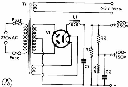
Fig. 2. Circuit of a simple general-purpose power pack, suitable for most receiver applications and for general work round the station. It can be built in a metal box, or on an open metal chassis with adequate protection, and in either case must be properly earthed.
