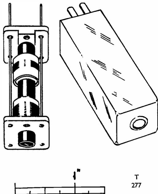
Fig. 1. Finished appearance of a typical coupler unit, with enclosing can.
