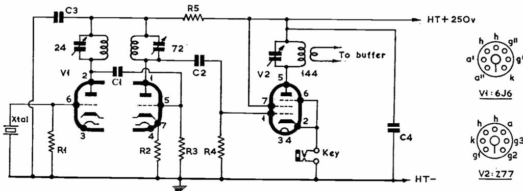
Fig. 2. Using a 6J6 and Z77 to get output at 144 mc from an 8 mc crystal. The multiplication sequence is 8-24-72-144 mc and there would be enough RF drive for a small buffer stage.
