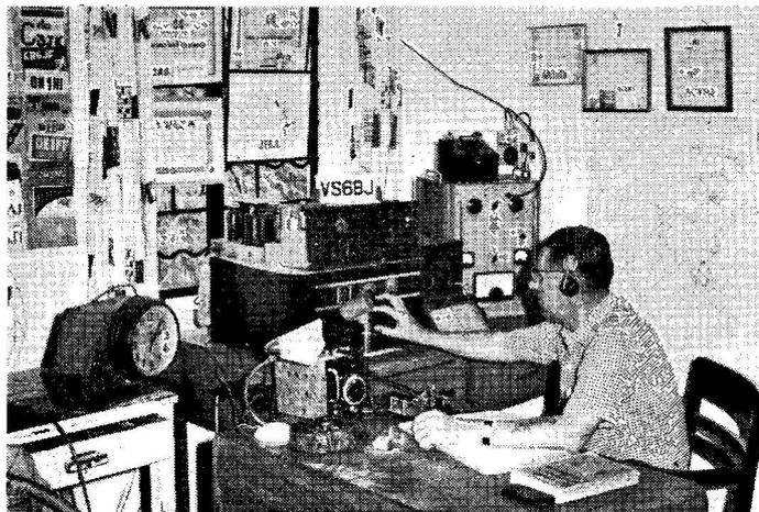
VS6BJ is one of the Hong-Kong group, located at Kowloon, and has an interesting station. The receiver is an AR88 and the transmitter a Labgear LG.300. For SSB working, he has a home-constructed half-lattice exciter with an 829B as PA.
