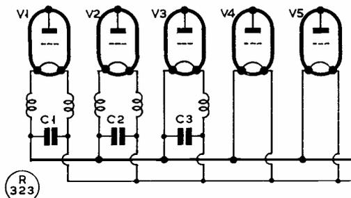
Fig. 5. Heater by-passing for the circuit shown in Fig. 4. C1, C2 are each .003  $\mu$ F and C3 is 270  $\mu$ F. Values for the heater chokes are given with the coil table.
