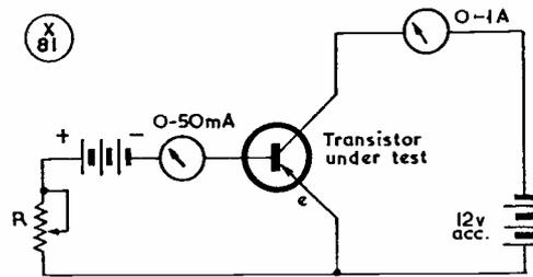
Fig. 3. It is desirable that well-matched transistors be used for TR1, TR2. This is a circuit for checking the beta-gain of transistors — see text. The resistance is 1,000 ohms wire-wound.
