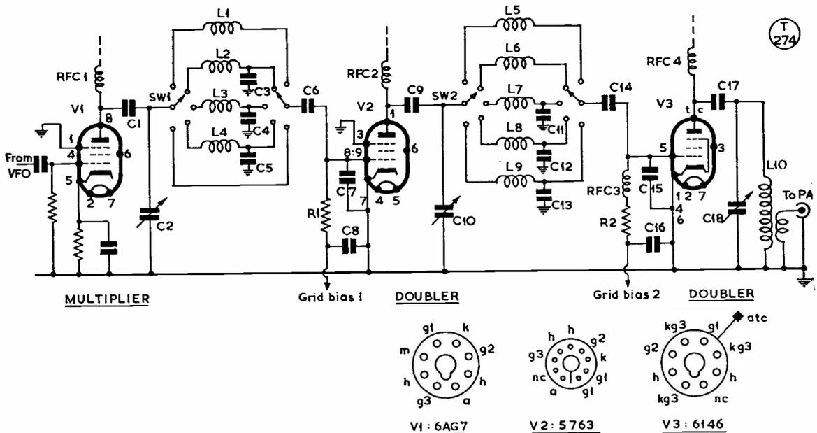
Fig. 2. The circuit arrangement as used by GM31AA. V1 is a buffer or frequency multiplier, and V2/V3 are doublers. In the fifth position of the switch SW1, V2 operates as a buffer with C2 at minimum; this would permit operation on 3.5 mc, as ample drive is available. The anode of V3 is conventional, drive to the PA grids being by coax cable and link coupling. In this circuit, screen connections and all wiring not relevant to the method of inter-stage coupling have been omitted.
