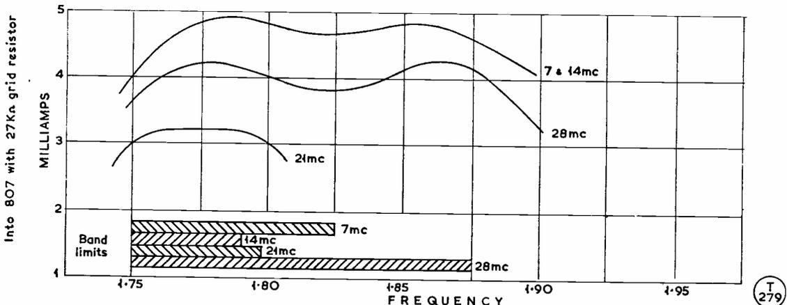
Fig. 3. Performance curves of the wide-band couplers described and illustrated in the article. These couplers are easy to make and full details are given in the text.
