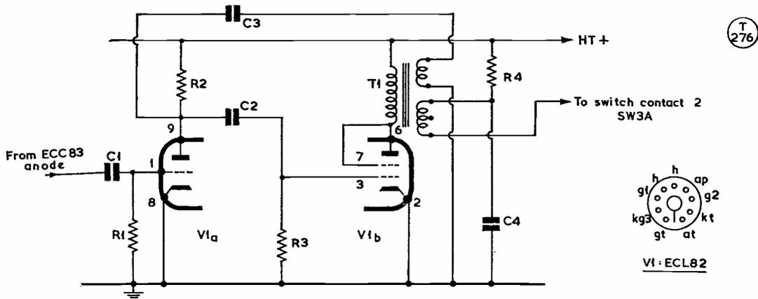
Fig. 2. Circuit modification suggested by G3MMW for improving phone working on the Heathkit DX-40U transmitter — and see Fig. 1. As explained in the text, no very drastic alterations are involved and G3MMW obtains better modulation characteristics using this arrangement than with the circuit specified for the transmitter.
