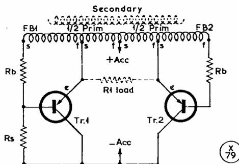
Fig. 1. The switching circuit used by G3KUM, giving a 400-cycle frequency for the primary side of the unit. TR1 and TR2 are power transistors, and when running up the temporary load R1 must be connected — see text. Rb is 2-5 ohms, using Eureka wire for the winding, and Rs is found experimentally, as explained in the article.
