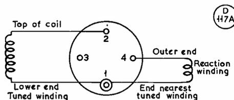
Circuit of the GDO described in the article; it is a great deal more sensitive than the usual arrangement because the second triode is used as a meter amplifier. The coil connections are shown below, pin 1 being the earth point, pin 2 the grid connection, and pin 4 the C3 end of the reaction winding. The former is the Eddystone No. 763 4-pin miniature.
