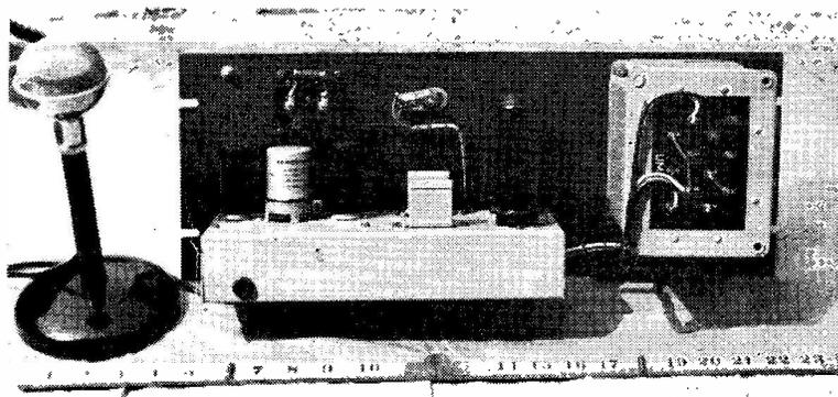
Impression of the general layout above chassis of the speech-amplifier/modulator described by G3MVY in the accompanying article. Provided the input side is properly screened, and layout of the parts approximates to the circuit diagram, any convenient form of construction may be adopted for apparatus of this sort.
