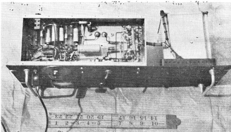
As constructed by G3MVY, the 25-watt modulator unit is mounted on a standard 19 ins. by 7 ins. rack; this view is with the bottom cover removed. Other forms of construction are possible, such as the open chassis with or without a screening cover, and this is always a matter of individual preference.
