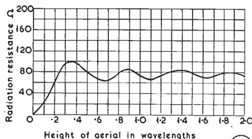
The well-known diagram showing the effect of aerial height on radiation resistance. A half-wave aerial is assumed.
