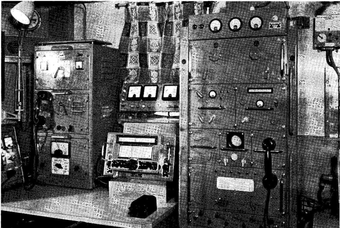
Radio room of the G.P.O. cable-ship "Monarch," fitted with the latest Marconi Marine equipment. In the assembly at left is the "Albatross" transmitter/receiver for local VHF R/T working, with the "Electra" receiver at centre. Above this is the remote control and indicating panel for the NT203 wideband RF amplifier; the cabinet on the right contains the NT201 ISB transmitter. Note the Morse key; most of the traffic with deep-sea ships is still worked by CW telegraphy.
