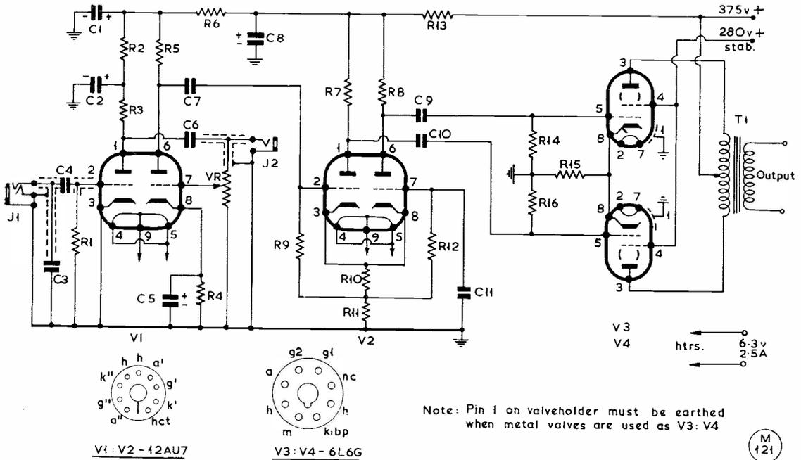
Note: Pin 1 on valveholder must be earthed when metal valves are used as V3: V4
