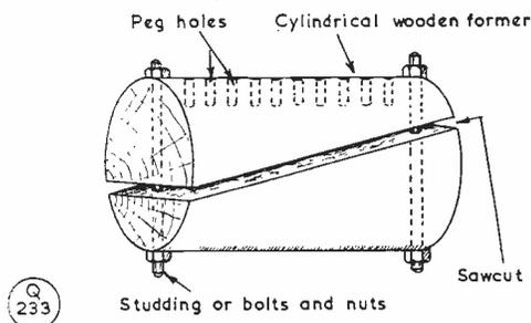
Fig. 1. Construction of a wooden mandrel, as described in the text, for winding transmitting coils. This is a re-usable former, and coils of different turns value can be wound up on it as and when required, the size being limited only by the length of the former.
