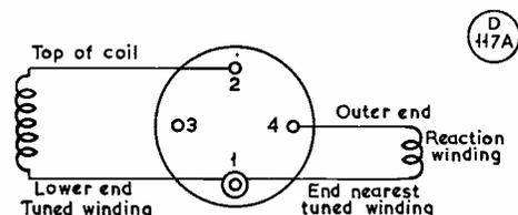
Circuit of the GDO described in the article; it is a great deal more sensitive than the usual arrangement because the second triode is used as a meter amplifier. The coil connections are shown below, pin 1 being the earth point, pin 2 the grid connection, and pin 4 the C3 end of the reaction winding. The former is the Eddystone No. 763 4-pin miniature.
