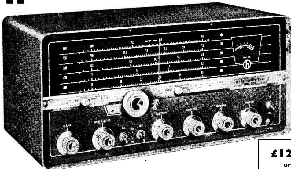
The SX-III is an exceptional communication receiver retaining most of the outstanding features of Hallicrafters SX-101. It has a sensitivity of 1 micro-volt on all bands and 5 steps of selectivity from 500 to 5,000 CPS. This dual conversion, selectable sideband receiver covers 80, 40, 20, 15 and 10 metres in 5 individual bands with a sixth band tunable to 10 mc for crystal calibrator calibration with WWV. High degree of mechanical and electrical stability is included with its high performance.
