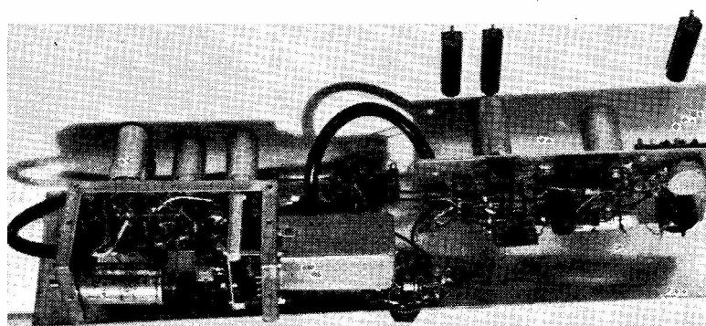
The GM3GOC SSB receiving adaptor is built on a chassis to fit the rack panel above the receiver with which it is used. It is shown here opened out for inspection; this unit is constructed to the circuit of Fig. 2.
