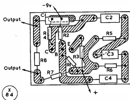
Fig. 2. Layout of the circuit of Fig. 1 on a home-made printed circuit board 3 1/2 ins. by 2 1/2 ins. Compare with photograph.
