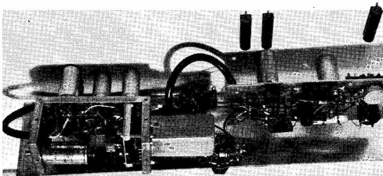
The GM3GOC SSB receiving adaptor is built on a chassis to fit the rack panel above the receiver with which it is used. It is shown here opened out for inspection; this unit is constructed to the circuit of Fig. 2.
