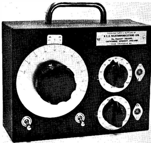
The new R.E.E. "Telecomm" VHF Signal Generator, in the Model B version, covers 100-150 mc, and is fully transistorised. The modulation is variable, and a 9-position attenuator gives a 90 dB change in output signal level from the minimum of approximately 1 microvolt. Tuning is by a slow-motion dial and the cabinet size is 8 ins. by 6 ins. by 3 ins. Other models are available covering 40-70 mc (Model A) and 70-72 mc with 85-87 mc (Model C). Other VHF ranges can be provided to special order.
