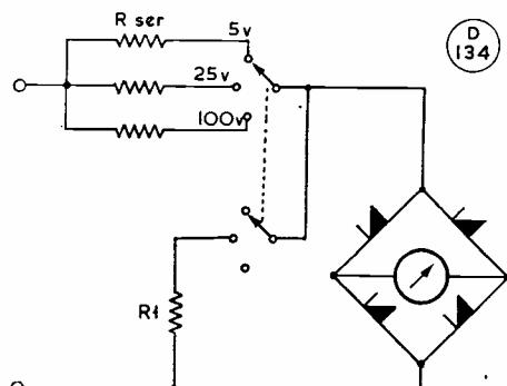
Fig. 2. Circuit arrangement of a rectifier voltmeter to read over the same scale for different ranges.
