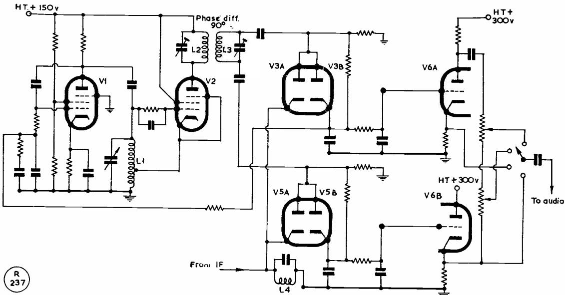
Fig. 1. Experimental SSB receiving adaptor circuit developed by GM3GOC. As explained in the text, there were difficulties in getting this working satisfactorily, but it was the basic design from which the circuit of Fig. 2 was evolved.
