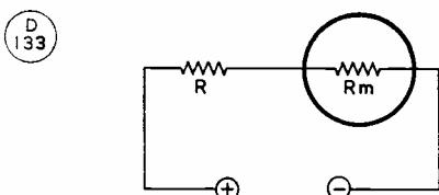
Fig. 1. Basic circuit of a voltmeter—see text.
