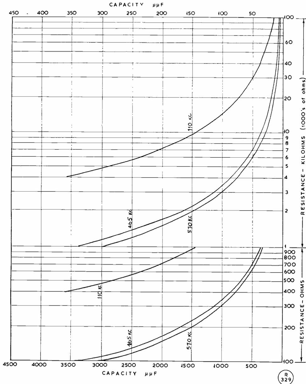
Fig. 3. Curves relating commonly used receiver intermediate frequencies (IF) with resistance-capacity values. From these graphs 90° phase-shift networks can be arrived at, cross-checked by the formulae given in the Appendix on p.462.
