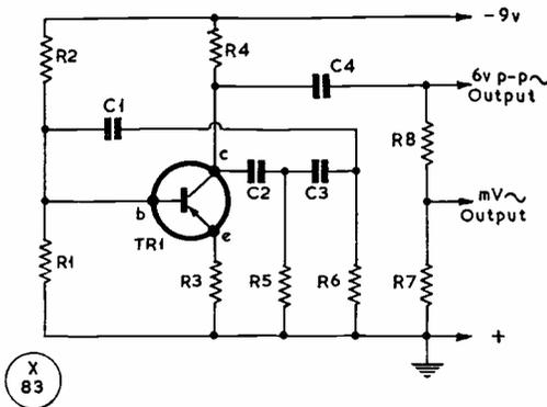
Fig. 1. Circuit of the audio oscillator, using a Mullard OC76 transistor. Values are: C1, C2, C3, C4, .01  $\mu$ F; R1, 15,000 ohms; R2, 390,000 ohms; R3, 12 ohms; R4, R5, R6, 4,700 ohms; R7, 220 ohms; R8, 220,000 ohms. All resistors can be rated  $\frac{1}{2}$ w. The values of R7, R8 may be changed to increase or decrease the low-level output, simulating a crystal microphone. With the values given the audio frequency will be about 1,000 cycles.
