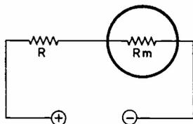
Fig. 1. Basic circuit of a voltmeter — see text.
