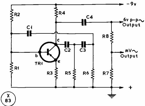
Fig. 1. Circuit of the audio oscillator, using a Mullard OC76 transistor. Values are : C1, C2, C3, .01  $\mu$ F ; R1, 15,000 ohms ; R2, 390,000 ohms ; R3, 12 ohms ; R4, R5, R6, 4,700 ohms ; R7, 220 ohms ; R8, 220,000 ohms. All resistors can be rated 1w. The values of R7, R8 may be changed to increase or decrease the low-level output, simulating a crystal microphone. With the values given the audio frequency will be about 1,000 cycles.
