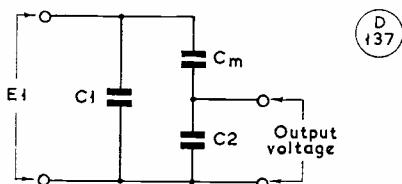
Fig. 5. An attenuator arrangement for the electrostatic voltmeter.
