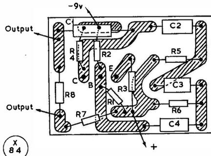
Fig. 2. Layout of the circuit of Fig. 1 on a home-made printed circuit board 3 1/2 ins. by 2 1/2 ins. Compare with photograph.
