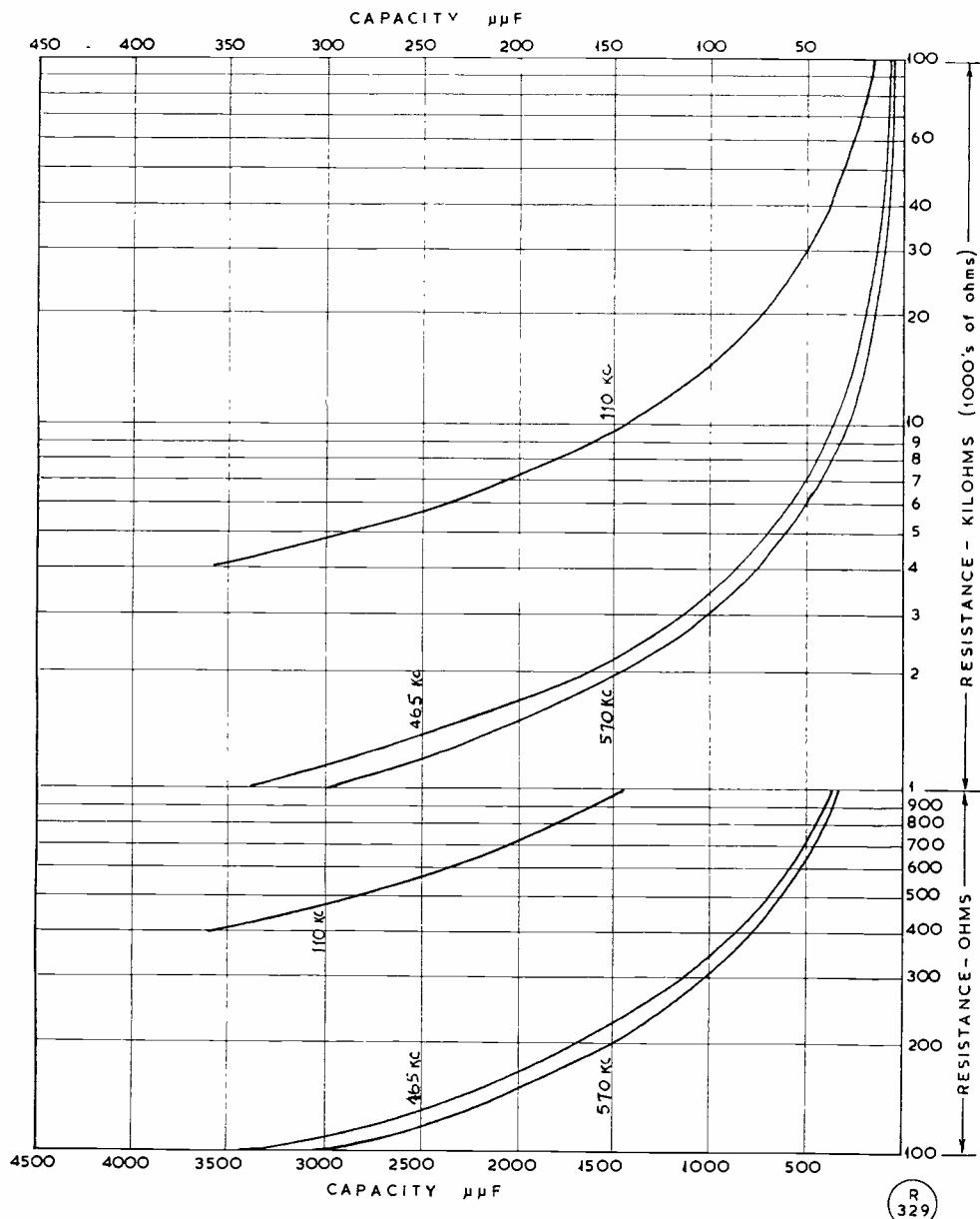
Fig. 3. Curves relating commonly used receiver intermediate frequencies (IF) with resistance-capacity values. From these graphs 90° phase-shift networks can be arrived at, cross-checked by the formulae given in the Appendix on p.462.
