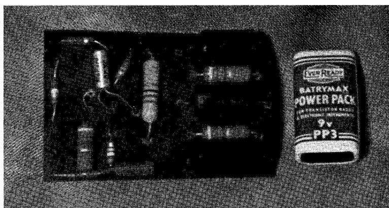
The transistorised audio oscillator constructed by G3MEO is on a home-made printed circuit board. Chemicals and laminated board for printed circuit work can be obtained in kit form.
