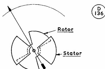
Fig. 4. Basic principle of the electrostatic voltmeter, normally used for continuous high-voltage readings.
