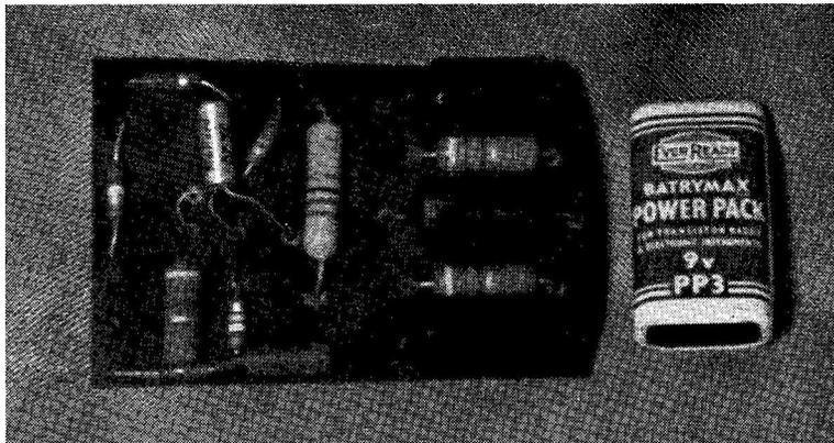
The transistorised audio oscillator constructed by G3MEO is on a home-made printed circuit board. Chemicals and laminated board for printed circuit work can be obtained in kit form.
