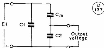
Fig. 5. An attenuator arrangement for the electrostatic voltmeter.
