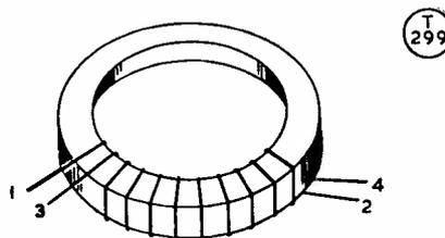
Fig. 4. Winding the toroid coil LT; the leads marked 1, 4 are connected to earth.
