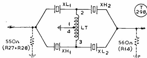
Fig. 3. The crystal filter for the Transceiver; it comprises two half-lattice sections back-to-back, tightly coupled by the winding LT, a home-made toroidal bifilar coil. The crystals are two identical pairs, XH1/XH2 being etched 1.5 kc higher than XL1/XL2, which have a nominal frequency of 8,400 kc. The filter input and output leads are shunted by 550-ohm resistors, essential to achieve correct filter characteristics.
