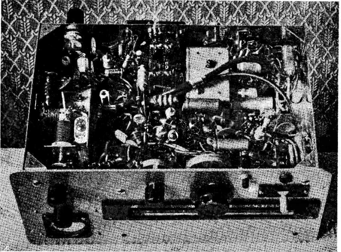
Underside view of the SSB Transceiver designed and built by G3BDQ.
