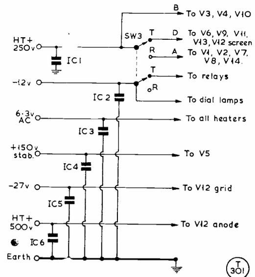
Fig. 6. A GPO type key-switch is used for SW3, the transmit-receive selector switch on the front panel — see photograph. SW3 switches HT to the appropriate sections of the equipment and also operates the IF and aerial relays. IC1-IC5 are  $.01 \mu\text{F}$  disc ceramics at the input sockets; IC6 is a  $.0018 \mu\text{F}$  disc ceramic rated at 1,200v. The negative 27v. bias for the PA is obtained from three 9v. dry batteries.
