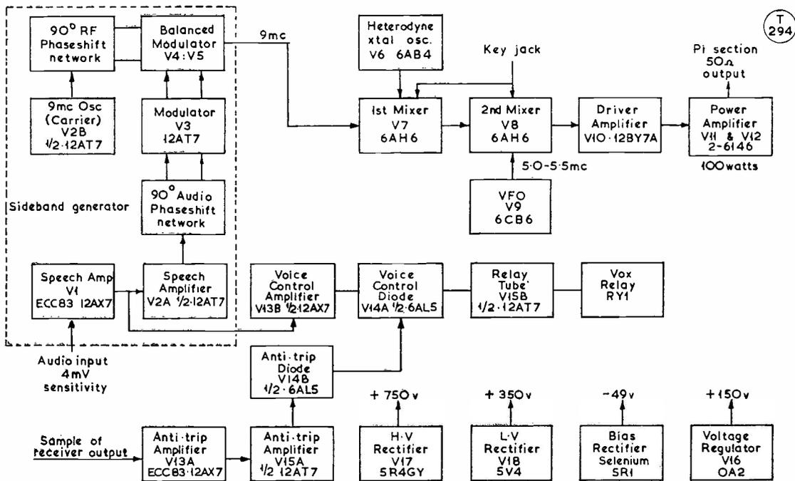
Fig. 4. General arrangement of the Hallicrafters HT-37 all-band SSB transmitter, and including all relevant circuitry. It will be noticed that in this design, carrier generation is at 9 mc with the VFO swinging across 5.0 to 5.5 mc. As in the K.W. Viceroy, the PA takes a pair of 6146's, and in both the output circuit is designed for a low-impedance load.
