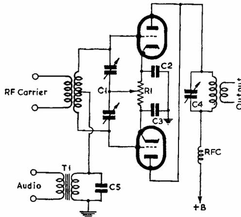
Fig. 2. Push-push balanced modulator, in which grid and anode circuits are both resonated at the carrier frequency. The RF excitation is applied to the grids in push-pull, and the audio in parallel, but the RF is suppressed in the parallel output tank. R1 is set for minimum carrier, and the two groups of sidebands again appear at the output terminals—see note in text regarding even harmonics.
