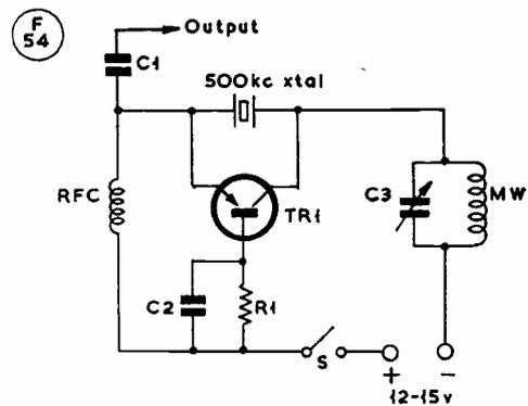
Circuit of a 500 kc marker unit in a transistor oscillator circuit, as described in the text. At this frequency, standard BC components can be used for the tuned circuit C3, MW.
