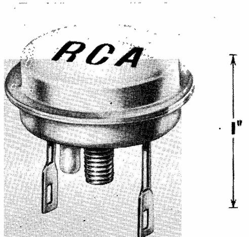
The new RCA 2N2015/2N2016 silicon power transistors are rated at 150 watts dissipation and operate at voltages of 100-130v. They are diffused-junction n-p-n types, and have a wide variety of applications in LF circuitry, the cut-off frequency being 25 kc.
