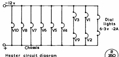
Fig. 3. Heater line connection for the six-band mobile receiver designed by G3GMN, for a 12-volt DC supply.
