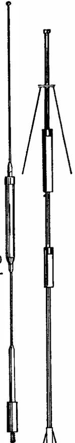
Vertical Aerial, 10 thru 40 no bandswitching is necessary.
