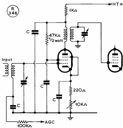
Fig. 1. A typical RF amplifier showing the values of resistor suitable for most valve types used in this position. Optimum values are shown in the Table.
