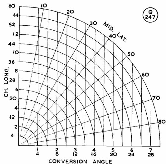
Fig. 2. G3MCY has worked out this chart so that the Conversion Angle (C.A.) can be read off quickly. For larger values of Ch. Long. the outer set of figures should be used, and the conversion angle taken from the outer scale.
