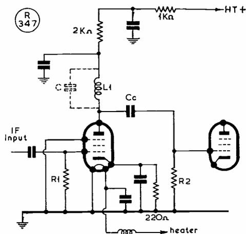
Fig. 2. A broad-band IF amplifier for use at high frequencies, notes on which are given in the text.
