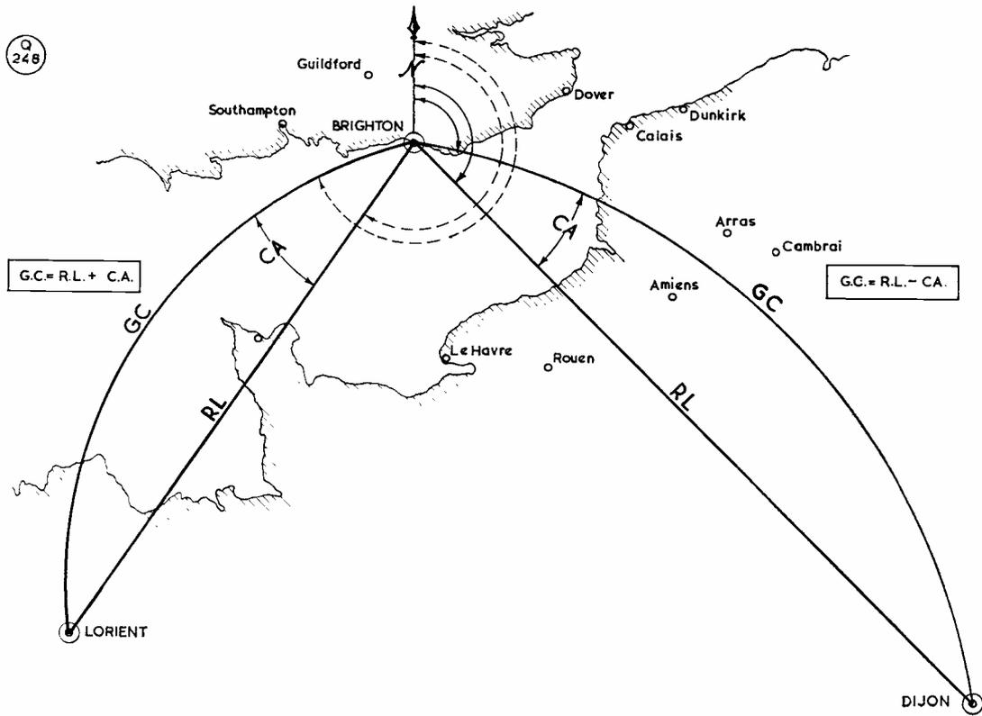
Fig. 3. Outline map showing application of the method of great-circle computation from a Mercator's chart, as explained by G3MCY in his article. It should be noted that all measurements are made clock-wise from the north point.
