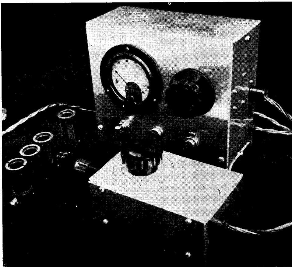
The instrument complete as described in the article; it can be used either as a grid dip oscillator or as a sensitive absorption wavemeter. In both cases, resonance tune is indicated on the panel instrument. The tuned circuit and the detector/oscillator valve are contained in the box in the foreground, which is used as the "test probe." The plug-in coils are the Eddystone miniature type, and are wound to cover a wide frequency range—see table below.
