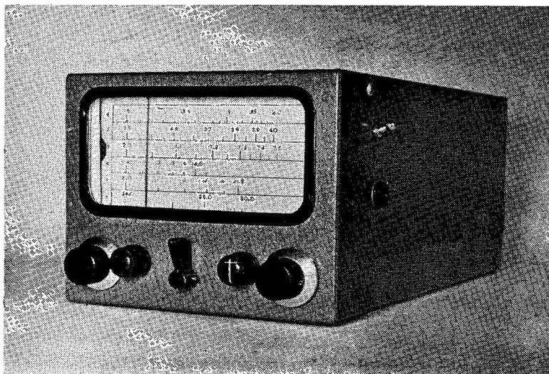
General view of the six-band mobile receiver designed and constructed by G3GMN. This is a double-conversion superhet (see circuit Fig. 1) and the size overall of the prototype as described and illustrated here is 6 ins. wide by 4½ ins. high by 12 ins. depth behind panel. The constructional layout is shown in the accompanying photographs.
