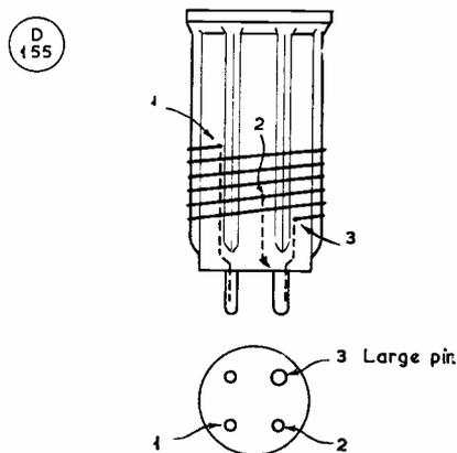
Fig. 3. Coil winding procedure for the GDO/Wavemeter. Turns data are given in the table, on p. 345, with approximate frequency coverage.
