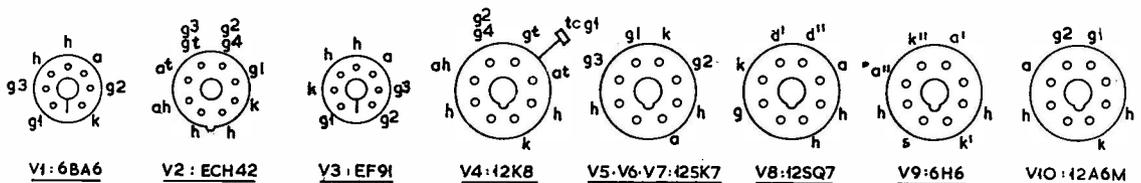
Fig. 2. Base connections for the valves used in the G3GMN 6-band double superhet receiver. They are all readily available types.
