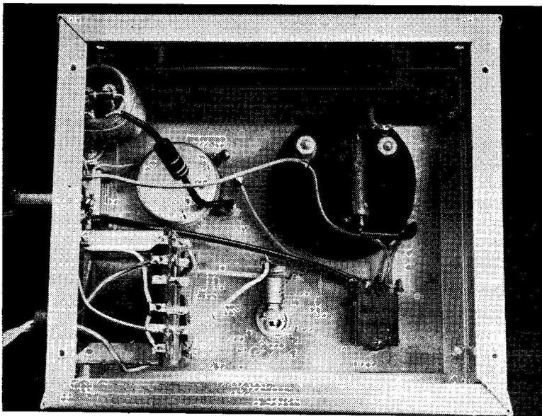
Construction of the meter box, which also incorporates the power supply for the instrument. The inter-connecting lead consists of a 4-way cable, long enough to give the probe end of the device its mobility.
