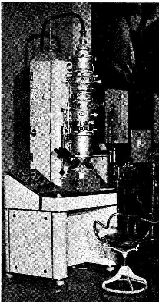
One of the scientific instruments shown at the recent Soviet Exhibition at Earl's Court was an electron microscope giving a magnification of 200,000 times. A specially designed filter protects bacteria under observation from being affected by the action of the microscope.
