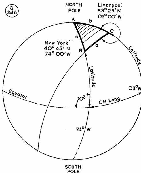
Fig. 1. The data upon which the calculations given in the text are based. The accuracy of the method is limited only by the exactitude with which the lat./long. is known of the points to be joined. C is the bearing angle.
