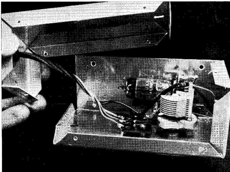
Inside the tuning box of the GDO/Absorption Wavemeter, showing the general construction. The valve is a 6C4, and power is fed in by a loose lead to enable the instrument to be freely used. The switching for GDO to Absorption is on the meter box, which also contains the power supply.
