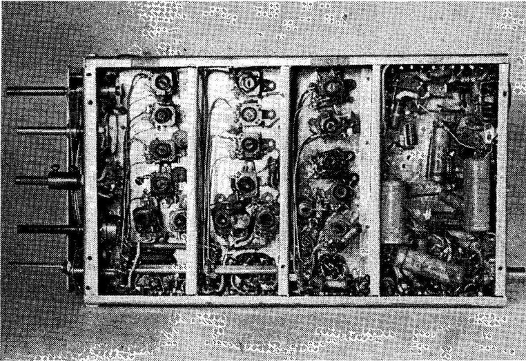
Under-chassis view of the six-band amateur receiver for mobile operation. Left, RF section; second compartment from left, mixer stage; third compartment, oscillator section; the fourth compartment from the left is the IF assembly.
