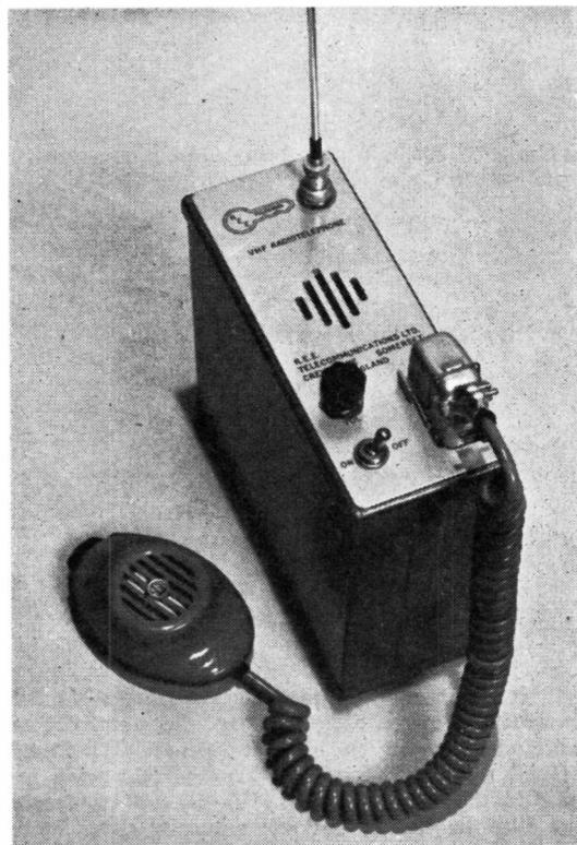
The R.E.E. Telecomm VHF/AM portable radio-telephone Type TRT/2 is fully transistorised in both receiver and transmitter; is designed for single-channel working in the range 50-100 mc; the aerial is a  $\frac{1}{2}$ -wave whip; and the power output 180 mW. The transmitter output transistor is a Mullard AFY10, and the power supply two 6-volt Mallory mercury cells.
