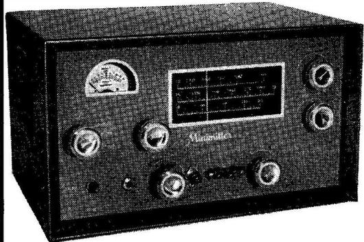
An extremely compact, efficient 24 watt transmitter for lower frequency bands: 1.8, 3.5, 7.0 Mc/s. Completely Self-Contained, with built-in Aerial, change-over and control relays — Input and Output monitoring — V.F.O. and Crystal Control — Large "slide rule" V.F.O. dial — "Picture Frame" front panel — Complete remote control facilities.
