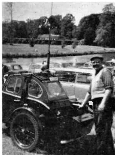
G3LZR/M, Romford, Essex, with his motorcycle combination, on which he journeys to many of the Rallies; he was at Longleat on June 17. His gear is on single-switch control; he has a transistorised speech amplifier and all home-built equipment; he can operate while motoring; and he gets ranges up to 20 miles under actual /M conditions.
