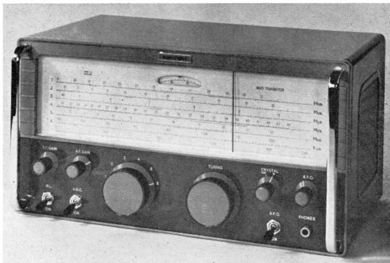
The Eddystone 960, seen on the stand of Webbs Radio at the Seymour Hall Exhibition this year, is a very interesting design in that it is all-transistor, tuning 500 kc to 30 mc in six ranges, and has a full communications specification. The power supply is a 12-volt battery.
