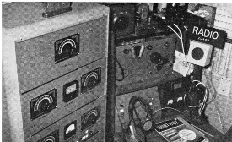
Neat station operated by Derek Morris, ZL4OP, 134 Stobo Street, Invercagill, New Zealand. His Tx is all-band with an 813 PA, modulated by a pair of 807's, and aerials are a ground-plane and an 80-metre Zepp. The main Rx is a BC-342, and the stand-by Tx an ARC-5. ZL4OP was licensed in 1957, comes from Lancing in Sussex, is active mainly on 20m. CW, 0300-1000 GMT, and has 62 countries confirmed. He has been out in N.Z. since 1952.
