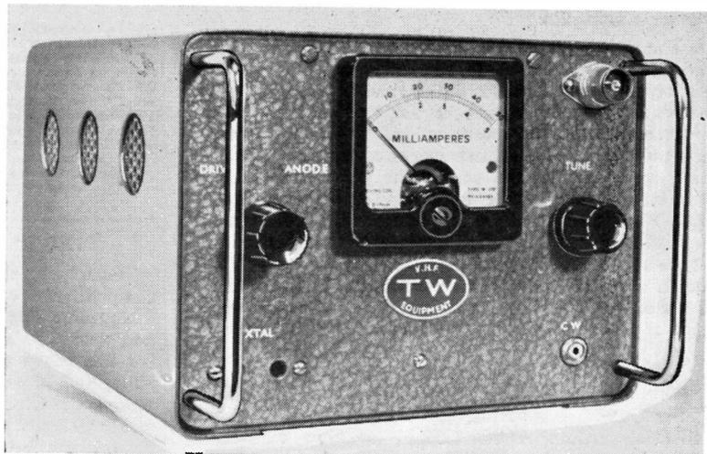
On view on the Withers stand at the International Radio Communications Exhibition — the TW VHF transmitter, a very neat little 10-watt CW/phone job which, in spite of its small size, is highly efficient. The PA is a QV03-10 modulated by a pair of EL84's. The transmitter is available for either 2, 4 or 6 metres (overseas).
