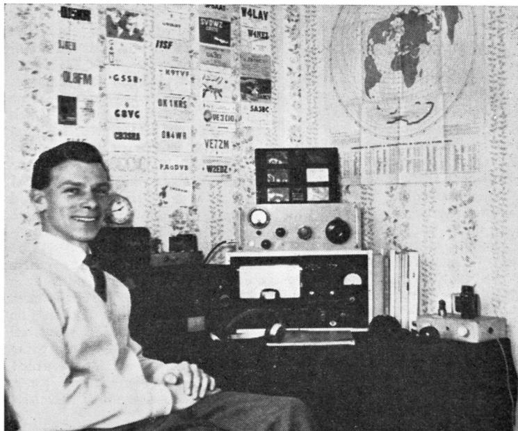
G3NRI is one of the Yorkshire stations, and runs a home-built Tx using a Gelo VFO driving a 6146 PA to about 45 watts, the receiver being an HRO. For the occasional phone QSO, cathode modulation is used, and the station equipment includes a dummy-load and SWR indicator incorporated in the ATU, also a 100 kc CC oscillator for calibration. Activity is mainly CW on the 15-20-40 metre bands.
